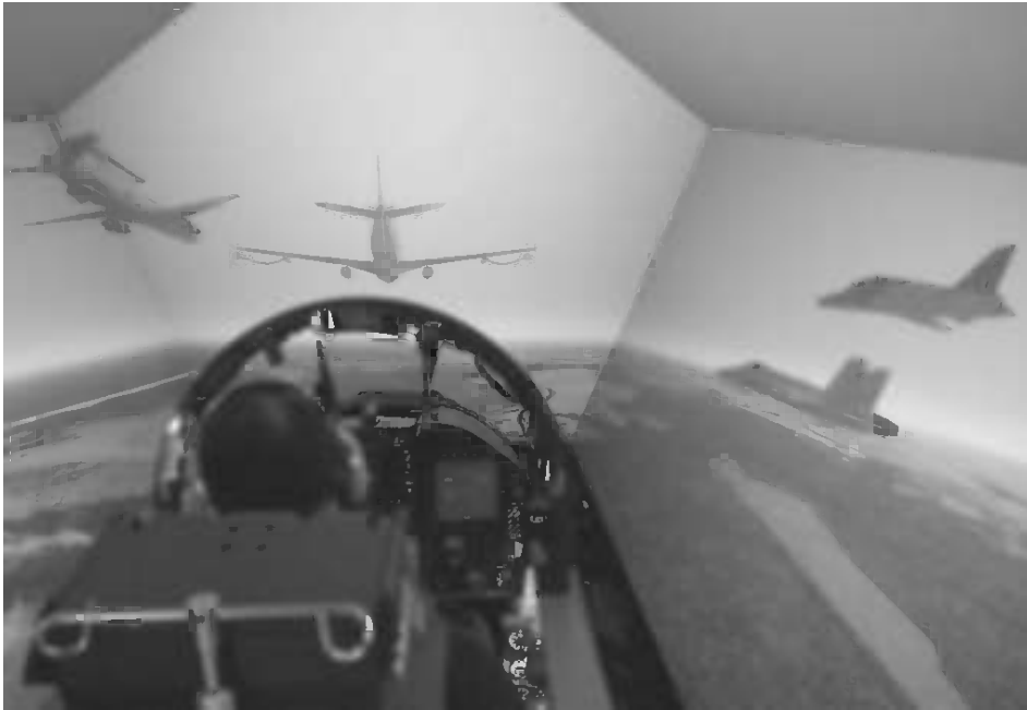
FIGURE 3. A Human-In-The-Loop F/A-18 Hornet Flight Simulator.
