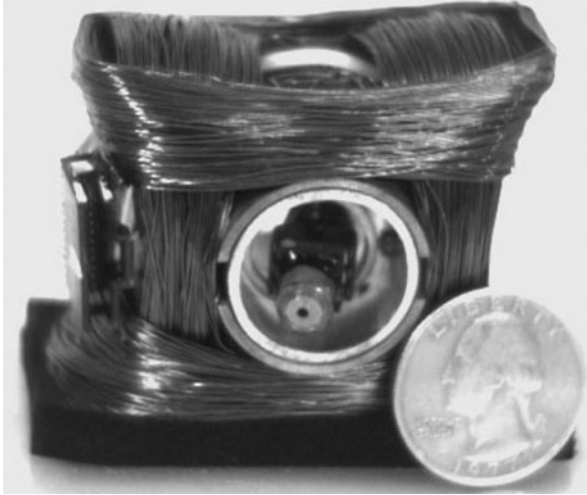
Fig. 1.13: Miniature pan-tilt actuator by Bederson et al. [58] ©1994 IEEE
