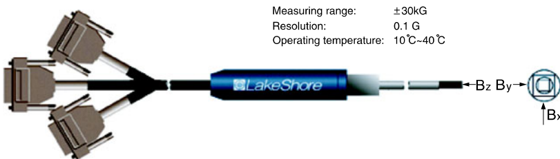
Fig. 5.3: Three-axis Hall probe (Lake Shore MMZ-2502-UH) [1]
