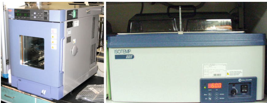
Fig. 7 Temperature humidity chamber (Left) and hot water chamber (Right)
