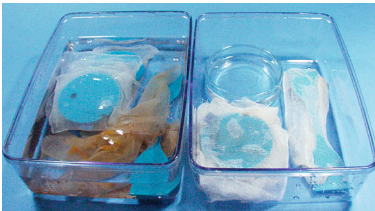
Fig. 8 Water immersion specimens in containers ( Left: water immersion, Right: vapor exposure )
