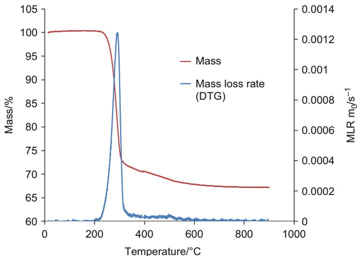
**Fig. 1** TGA and DTG curves for ATH decomposition in nitrogen at  $10\text{ °C min}^{-1}$
