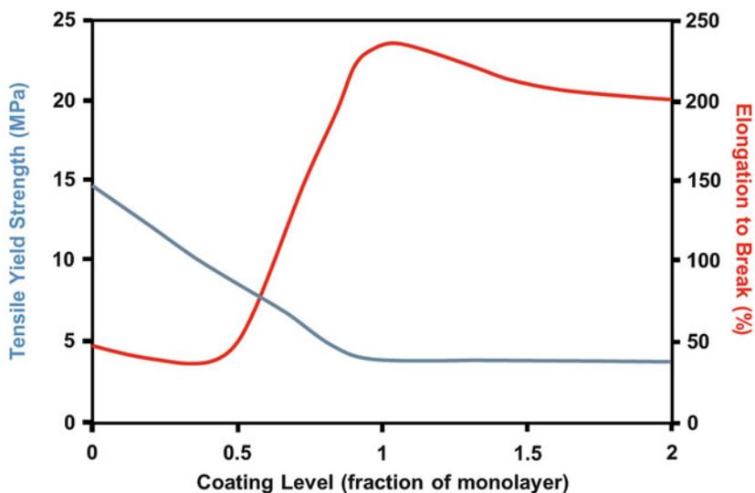
**Fig. 5** Effect of fatty acid coating level on the properties of a magnesium hydroxide-filled EVA compound (adapted from Rothern et al. 2002a)
