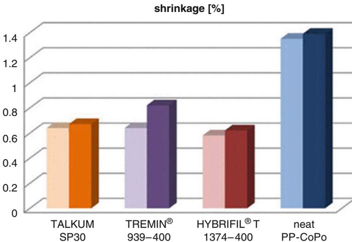
**Fig. 10** Shrinkage (parallel and perpendicular to injection molding direction) and anisotropy of the mineral mixture in comparison to talc and wollastonite
