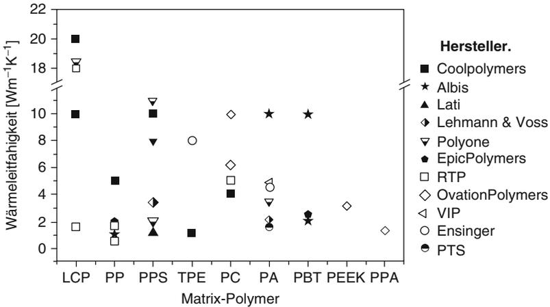
**Fig. 11** Commercial available thermally conductive compounds in various thermoplastics matrices (Heinle 2012)
