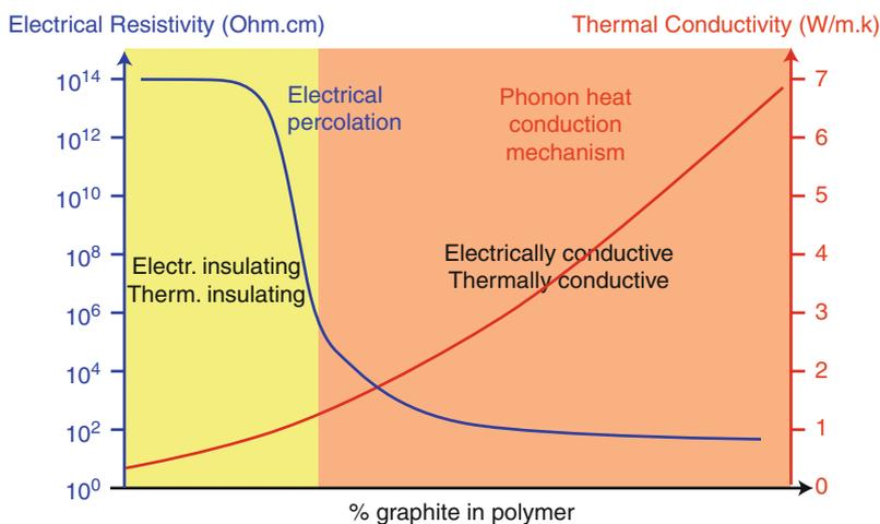
**Fig. 6** Schematic view of electrical and thermal conductivity as a function of graphite loading in polymer composite. The electrical resistivity decreases sharply at the percolation threshold, whereas the thermal conductivity increases smoothly
