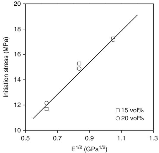
determined in PP/CaCO<sub>3</sub> composites from volume strain measurements is plotted against the stiffness of the matrix in Fig. 15 in the representation predicted by the model (Sudár et al. 2007). The correlation is close and corresponds to the prediction. Similarly, good correlations can be obtained if we plot debonding stress against the reversible work of adhesion (Pukánszky and Vörös 1996) or the particle size of the filler (Pukánszky et al. 1994b) (see Eq. 9).
