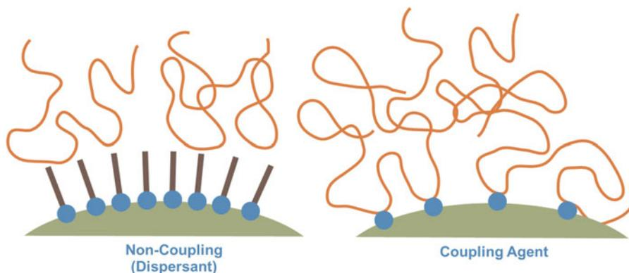
**Fig. 1** Noncoupling and coupling modifiers
