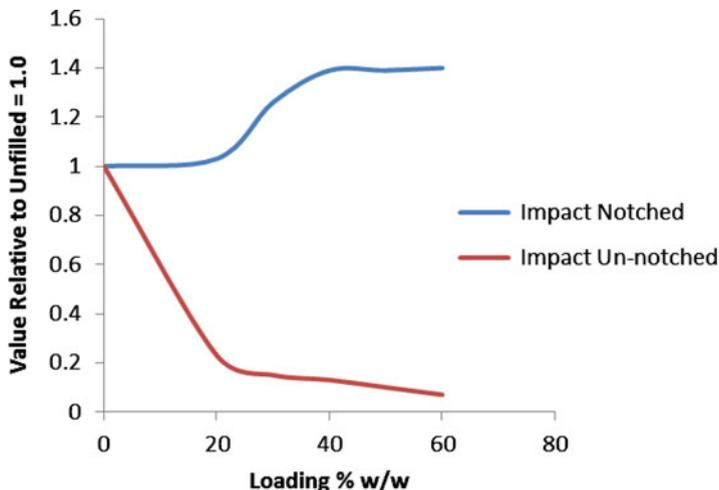
**Fig. 2** Effect of wood loading on the impact resistance of a polypropylene homopolymer (adapted from C.M. Clemons 2010)
