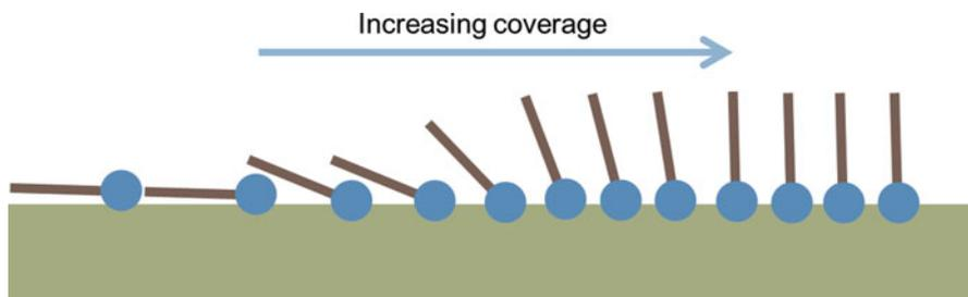
**Fig. 2** Different possible orientations of an adsorbed fatty acid chain
