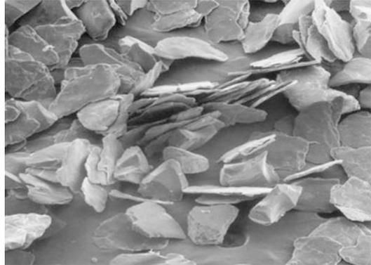
**Fig. 2** Microphotograph of a typical muscovite mica (500× polarized reflected light). Market data of mica minerals
