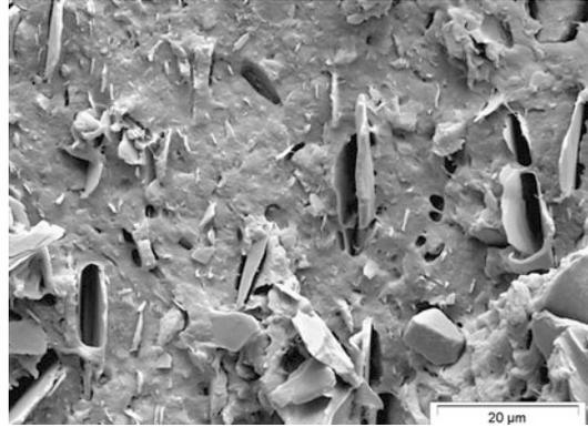
**Fig. 5** Scanning electron micrograph; micronized muscovite mica *with* surface treatment in polyamide after a tough fracture
