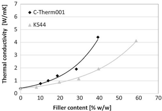
**Fig. 11** Through-plane thermal conductivity of compression-molded TIMREX C-THERM 001 (squares) and TIMREX KS44 (triangles) synthetic graphite-loaded HDPE
