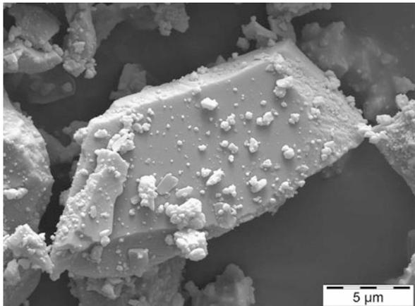
**Figure 7** SEM of precipitated silica
