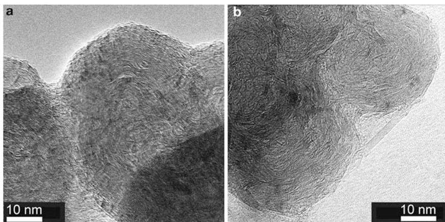
**Fig. 1** HRTEM images of typical primary particles for ENSACO<sup>®</sup> 250G (a) and acetylene black (b)
