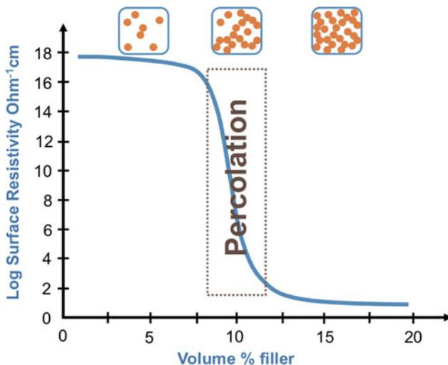
**Fig. 9** Percolation of electrically conductive particles
