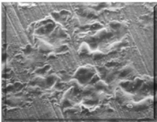
**Figure 3** SEM of feldspar flour 87% orthoclase, 7% albite, 4% kaolinite, 2% quartz
