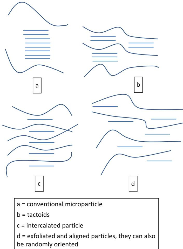
**Fig. 2** Different structures for a layered mineral composite
