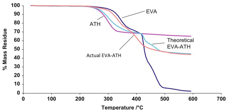
**Fig. 3** TGA curves of the individual components of an EVA-ATH compound (~27% vinyl acetate EVA at an ATH loading of ~70%) together with the theoretical curve obtained by adding the TGA curves of the individual components in proportion to their mass in the compound.
