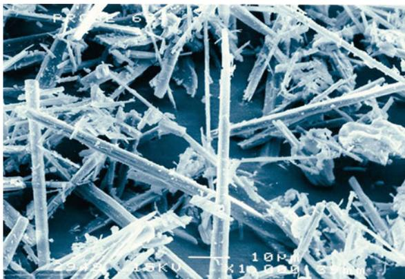
fractions with aspect ratio of up to 30:1 – is displayed in Fig. 3. This type is called high-aspect-ratio (HAR) wollastonite.
