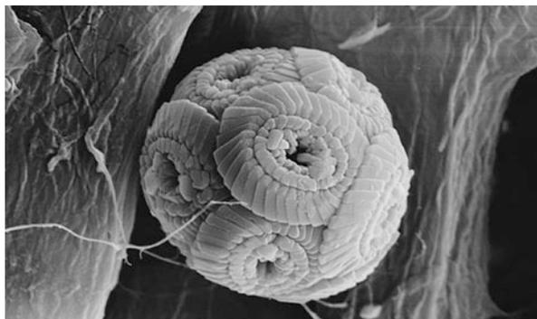
**Fig. 2** Fine chalk-based filler formed by breaking apart the calcite crystallites in a wet-grinding process
