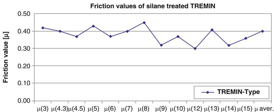
**Fig. 18** Friction values of a silane-treated HAR wollastonite
