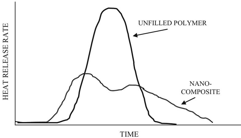
**Fig. 4** Schematic of the sort of cone calorimeter results obtainable from low levels of nanoclays (reproduced, with permission, from *Particulate-Filled Polymer Composites* (Ed Rothon R.N.), 2nd Edition, Rapra Technology, Shawbury UK, 2003)
