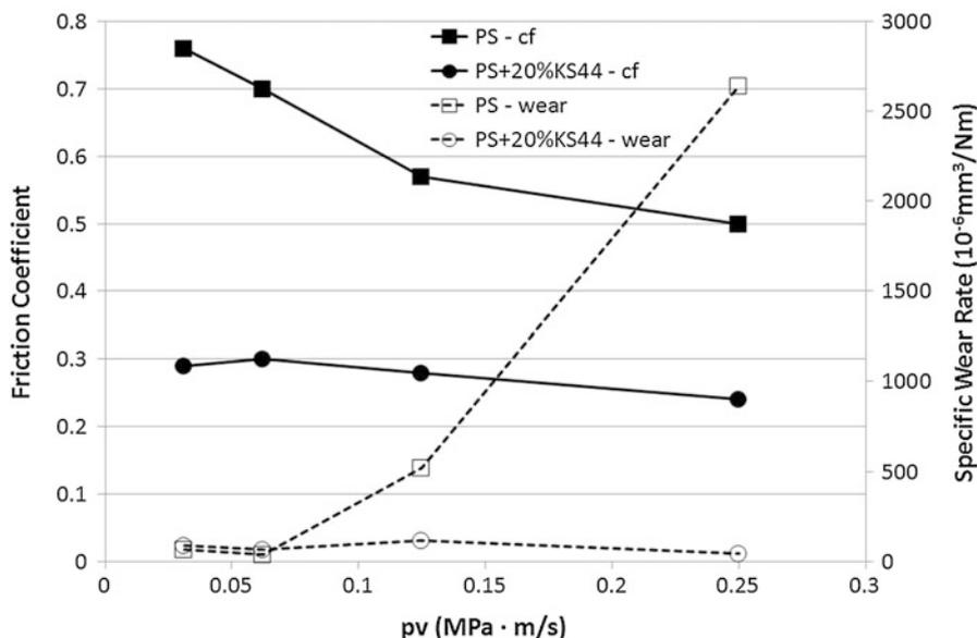
**Fig. 7** Friction coefficient and wear rate as a function of tribological stress for virgin PS and graphite-filled PS compound
