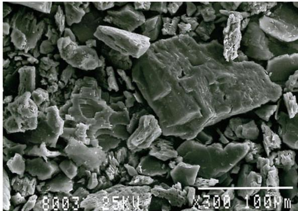
**Figure 6** SEM of calcined clay (kaolin)
