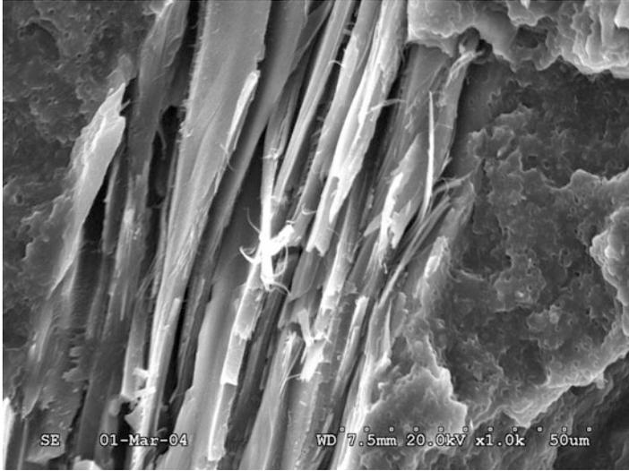
**Fig. 17** SEM micrograph showing the fracture of a wood particle during the deformation of PP/wood composites. Good adhesion of the components was achieved by the use of functionalized PP
