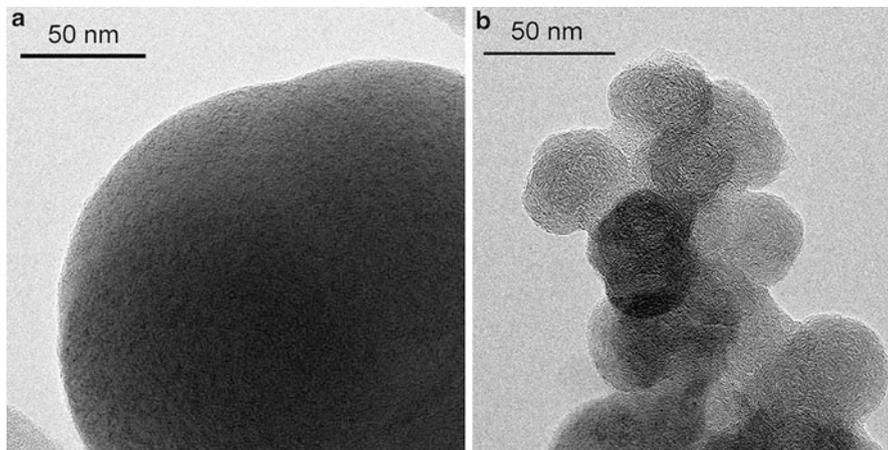
**Fig. 3** HRTEM images of primary particles of N990 (a) and N330 (b) carbon blacks
