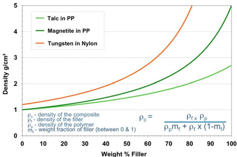
Fig. 1 Dependence of density on filler concentration
