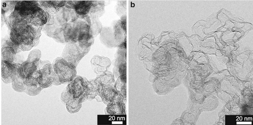
**Fig. 4** TEM (a) and SEM (b) images indicating the high carbon black structure of ENSACO<sup>®</sup> 250G consisting of agglomerates of carbon black aggregates with branched shape. An example of one aggregate is indicated by the *circle*
