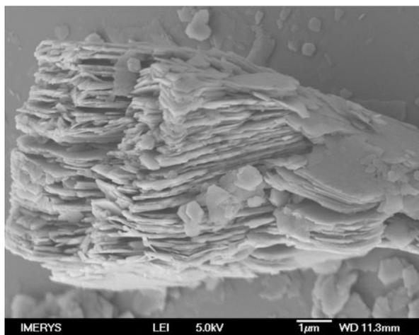
**Fig. 2** Typical kaolinite plates (reproduced with kind permission from Imerys)
