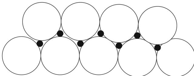
**Fig. 8** Use of the particle packing principle to maximize filler loading (reproduced with permission of Smithers Rapra)
