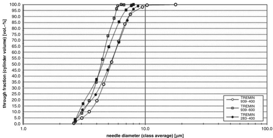
Fig. 4 Volume through fraction versus diameter of wollastonite fibers
