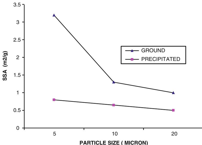
**Fig. 6** Variation of SSA with particle size for two types of aluminum hydroxide
