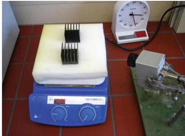
isolated versus the surroundings. Figure 5 shows the setup with the EP/alumosilicate heat sink at the front.
