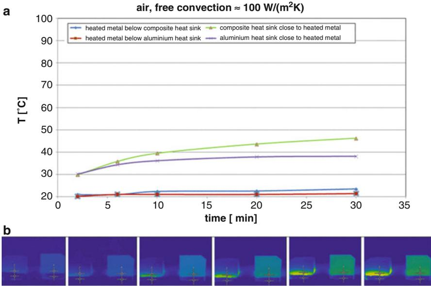
**Fig. 9** (a, b) Temperature over time of composite and aluminum heat sink, respectively, their metal support (as substitute for the electronics to be cooled) under forced convection (approx.  $100 \text{ W}/(\text{m}^2 \text{ K})$ ) with reduced material thickness on the composite heat sink base
