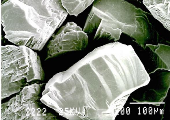
**Figure 5** SEM of anhydrite
