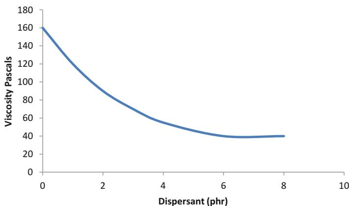
**Fig. 4** Use of a dispersing agent to reduce the viscosity of a highly filled UPR (275 phr ATH)
