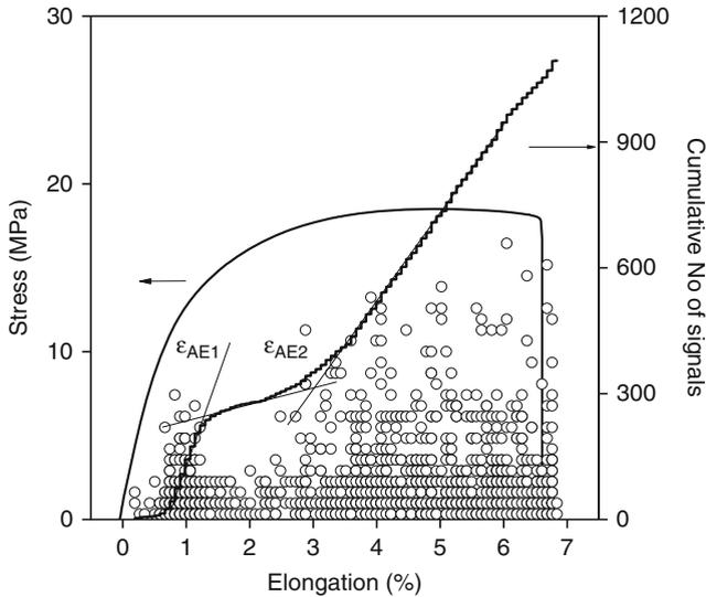
**Fig. 16** Acoustic emission testing of a PP composite containing 20 wt% wood without MAPP (poor adhesion). Small circles indicate individual acoustic events. Stress vs. strain and cumulative number of signal vs. strain traces
