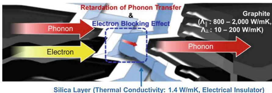
**Fig. 8** Illustration of the retardation of phonon transfer and electron blocking effect of silica-coated graphite. The size of the *red arrow* indicates the heat flux (reprinted from Choi et al. (2013) with permission from Elsevier)
