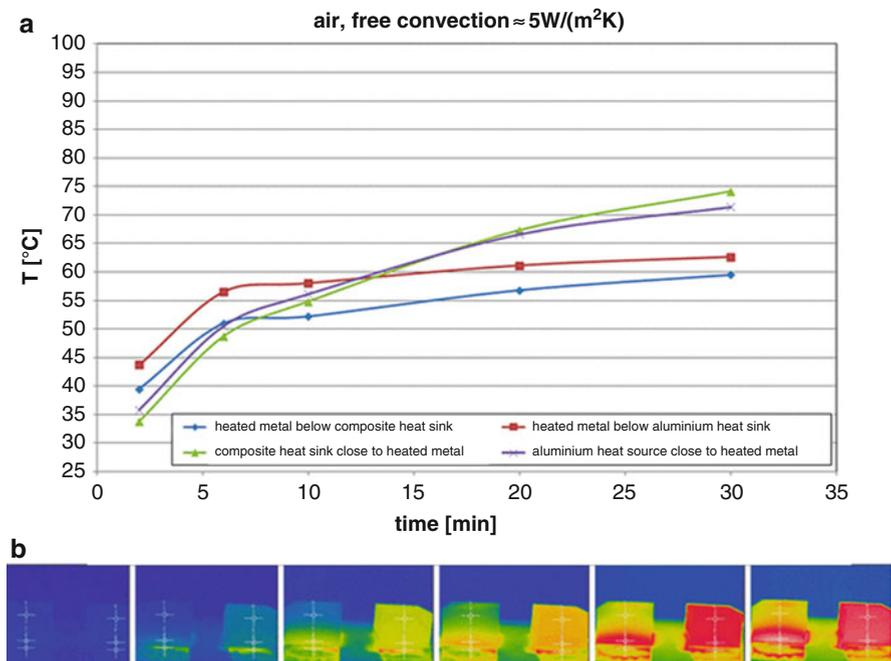
**Fig. 6** (a, b) Temperature over time of polymer composite and aluminum heat sink, respectively, their metal support (as substitute for the electronics to be cooled) under free convection (approx.  $5\text{ W}/(\text{m}^2\text{ K})$ )
