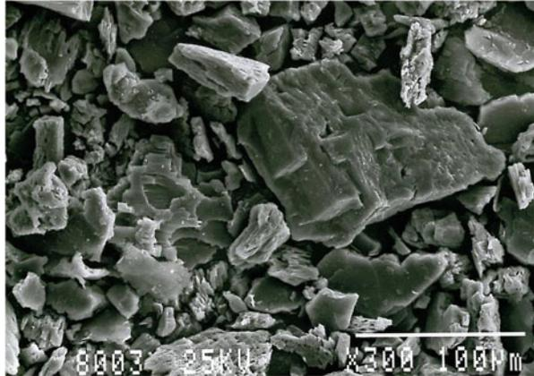
**Fig. 4** SEM of nepheline syenite flour: 25% nepheline, 73% feldspars, and 2% analcime and natrolite
