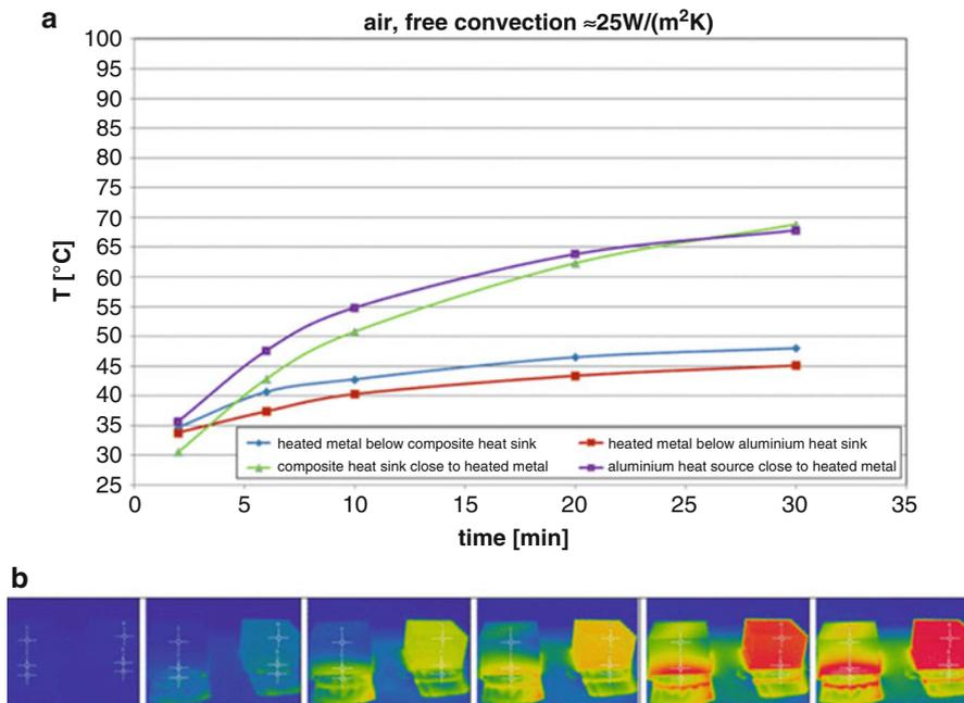
**Fig. 7** (a, b) Temperature over time of polymer composite and aluminium heat sink, respectively, their metal support (as substitute for the electronics to be cooled) under free convection (approx.  $25\text{ W}/(\text{m}^2\text{ K})$ )
