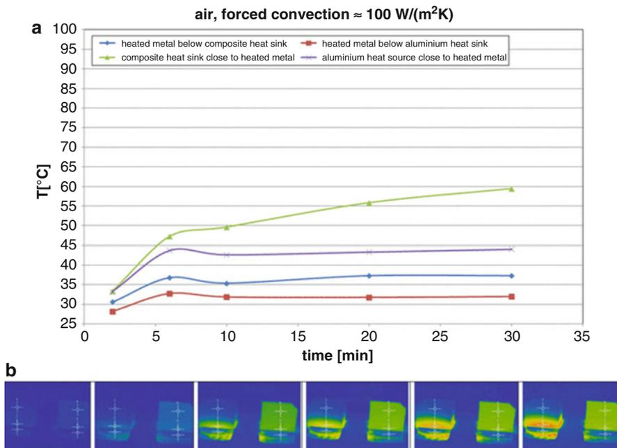
**Fig. 8** (a, b) Temperature over time of composite and aluminum heat sink respectively their metal support (as substitute for the electronics to be cooled) under forced convection (approx.  $100 \text{ W}/(\text{m}^2 \text{ K})$ )
