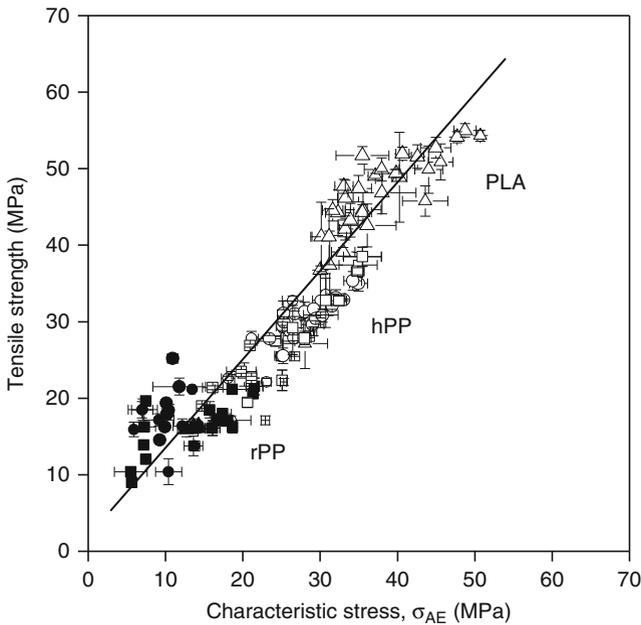
**Fig. 18** Close correlation between the initiation stress of the dominating deformation process and the strength of the composite. Symbols: ( $\square$ ) rPP/wood, ( $\circ$ ) hPP/wood, ( $\Delta$ ) PLA/wood. Full symbols: poor adhesion, empty symbols: good adhesion
