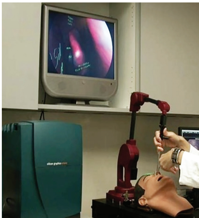
Fig. 46.6: ES3 simulator showing the endoscope and multiuse tool within the mannequin, as well as the apparatus utilizing screen guidance in a similar fashion to the operating room.
