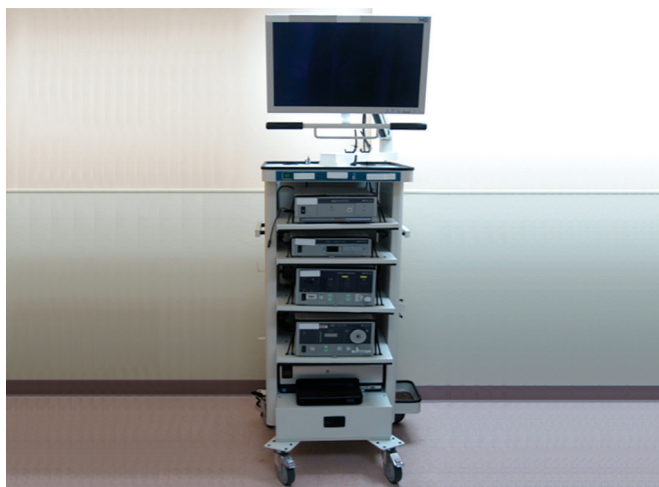
Fig. 47.2: The endoscopic tower consists of a high-definition monitor, digital video and still photograph recorder, and light source.
