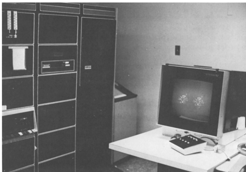
Fig. 1. View of the interactive graphics display in the Biographics Laboratory, Texas A&M University. Primary control of the display is through the 10 control dials.
