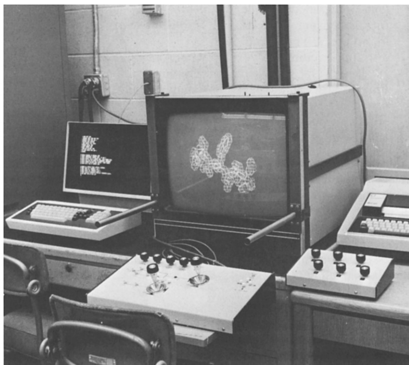
Fig. 2. The controls of the MMS-X molecular graphics system developed by the Computer Systems Laboratory of Washington University, St. Louis and now in use at Purdue University (courtesy of M. Rossmann, Purdue University).
