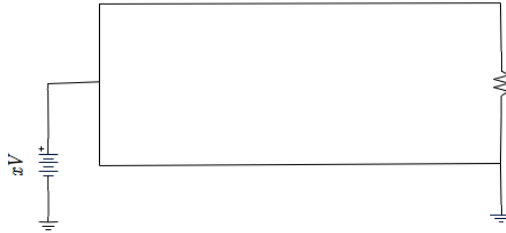
Fig. 7.28 Common mode conversion to differential mode interference
