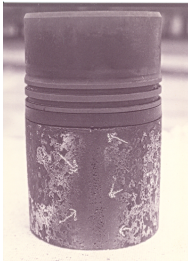
Figure 12. Corrosion in a carbon steel jacket on the water face in a diesel combustion engine truck.
