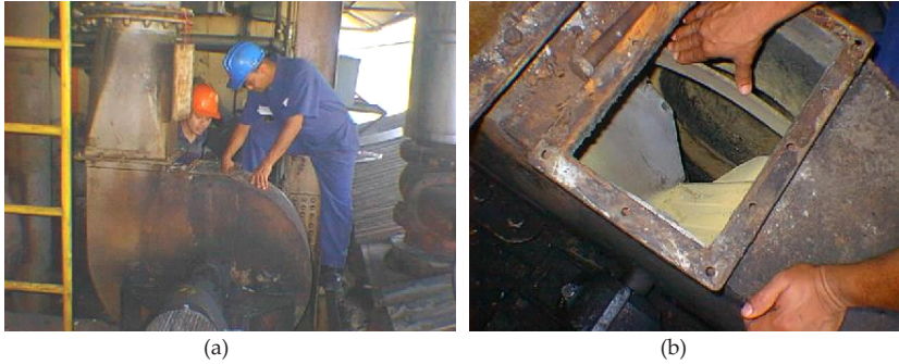
Figure 7. Photos of the attack-sites of samples: a) Ventilator extractor where samples were placed, b) Ventilator damp where samples were anchored.
