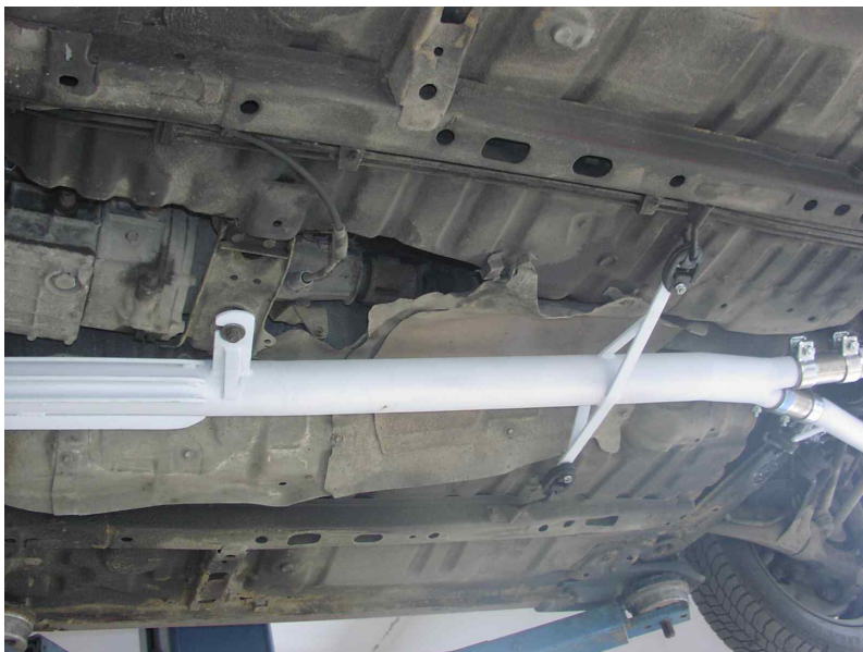
Figure 13. Corrosion on carbon steel exhaust pipes coated with aluminum.
