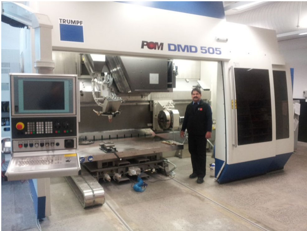
Figure 1. POM DMD (direct metal deposition machine) featuring 6-axis rotating, CAD-CNC control using a 5kW CO 2 Trumpf laser.
