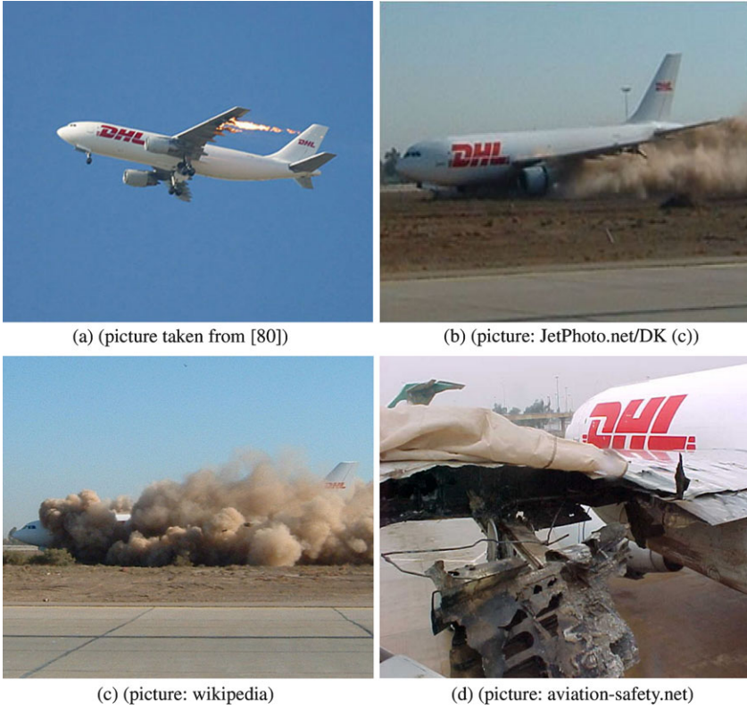
Fig. 1.3 DHL A300B4 emergency landing after being hit by missile in Baghdad, 2003
