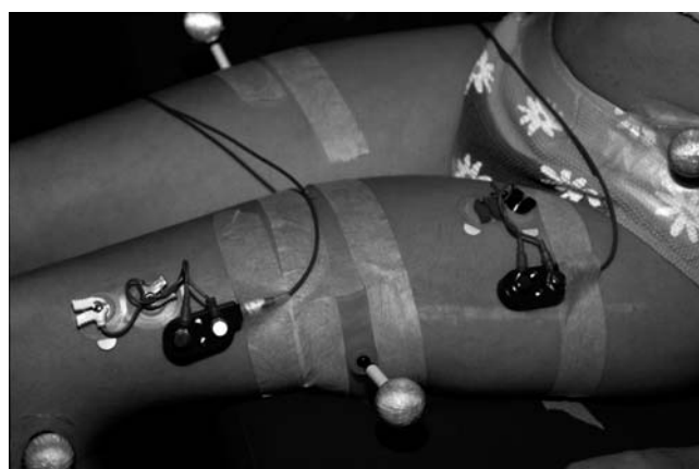
Figure 16.9 Patient with bipolar surface electrodes and small instrumentation amplifiers for recording dynamic EMG while the subject walks. This illustrates the electrode placement for the left vastus lateralis (distal location) and left rectus femoris (proximal location). Each electrode is connected to an instrumented backpack and then hardwired to the recording instruments. A wireless EMG recording system using similar electrodes but with individual transmitters for each muscle is shown in Figure 16.4.
