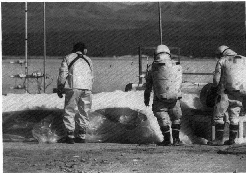
Figure 8 Nitrogen tetroxide spill covered with foam.
