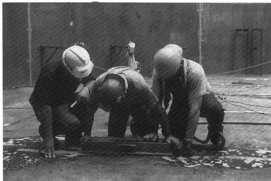
Figure 10 A vacuum box and soapy water can be used to check for leaks in welds on the floor of low-pressure tanks.
