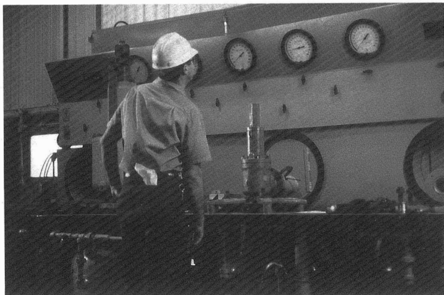
Figure 16 A well-trained mechanic testing a safety relief valve just as it is received from the unit.
