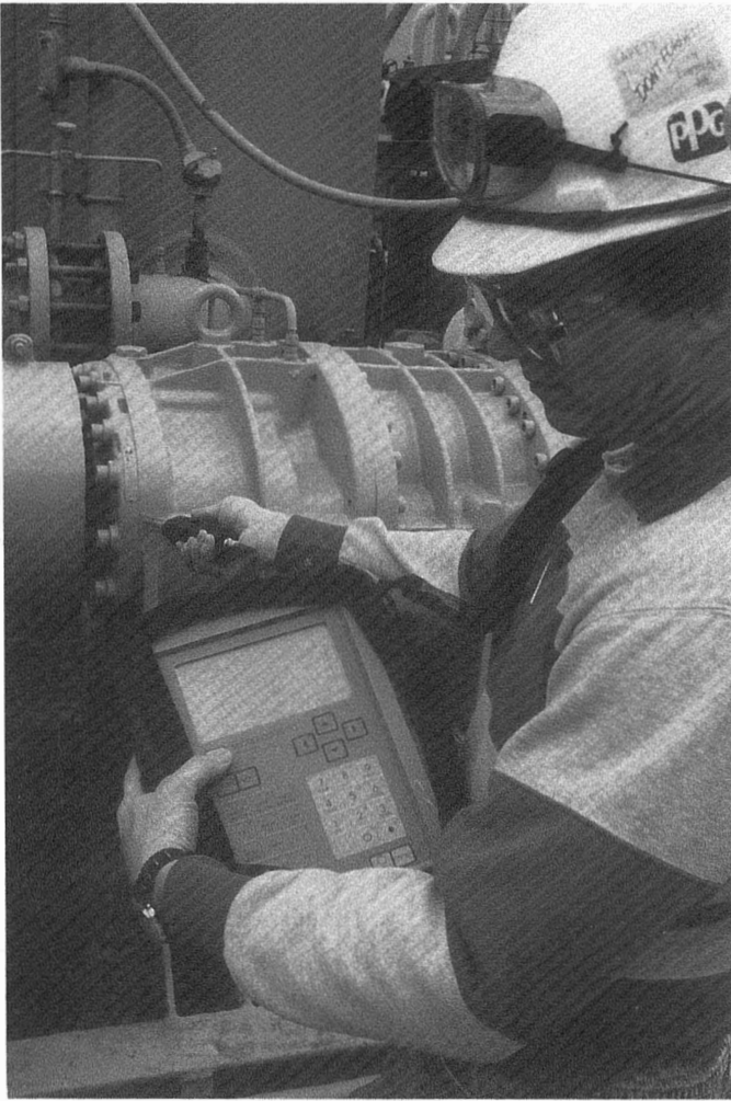
Figure 3 A close-up of a rotating machinery specialist with a vibration data acquisition module.
