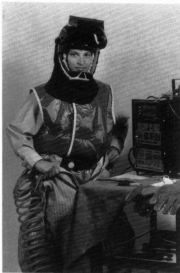
Figure 4 Supplied-air respirators provide protection in many operations including welding and paint spraying. (Courtesy of Racal Health & Safety, Inc.)
