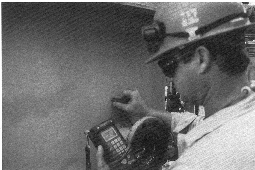
Figure 9 An inspector verifying wall thickness on a vessel near a nozzle that had experienced metal loss.
