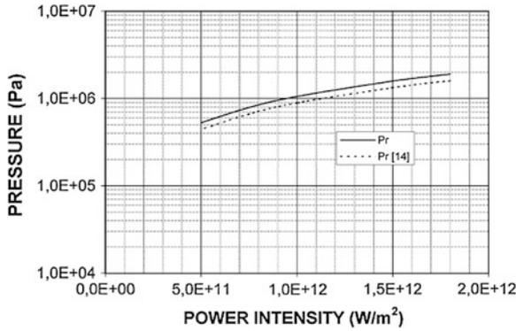
Fig. 2.62 Interface pressure with power intensity [35]
