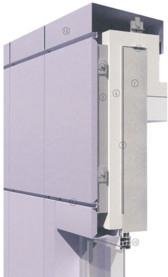
3-D view of window and parapet detail in rainscreen wall system
