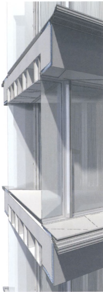
Sectional and exploded views of louvre shading system
