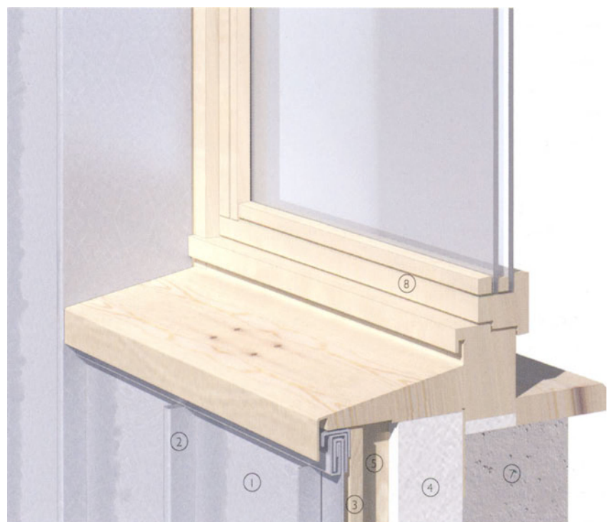
3-D view of window cill detail within profiled metal sheet system
