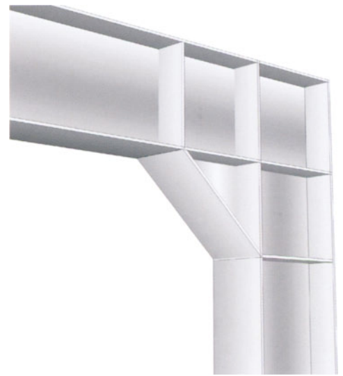
Rigid steel frame corner detail
