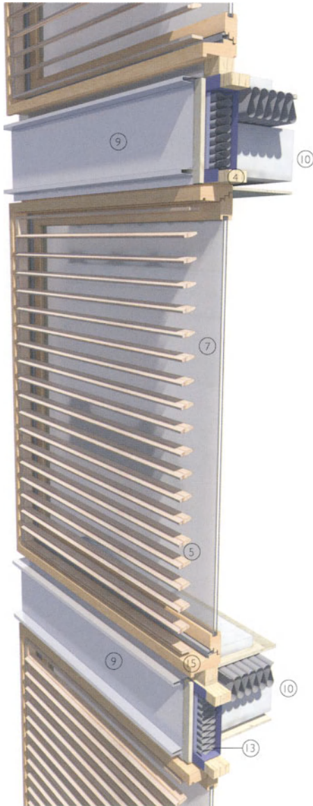
3-D view of timber cladding panel consisting of fixed glazing and louvre screen
