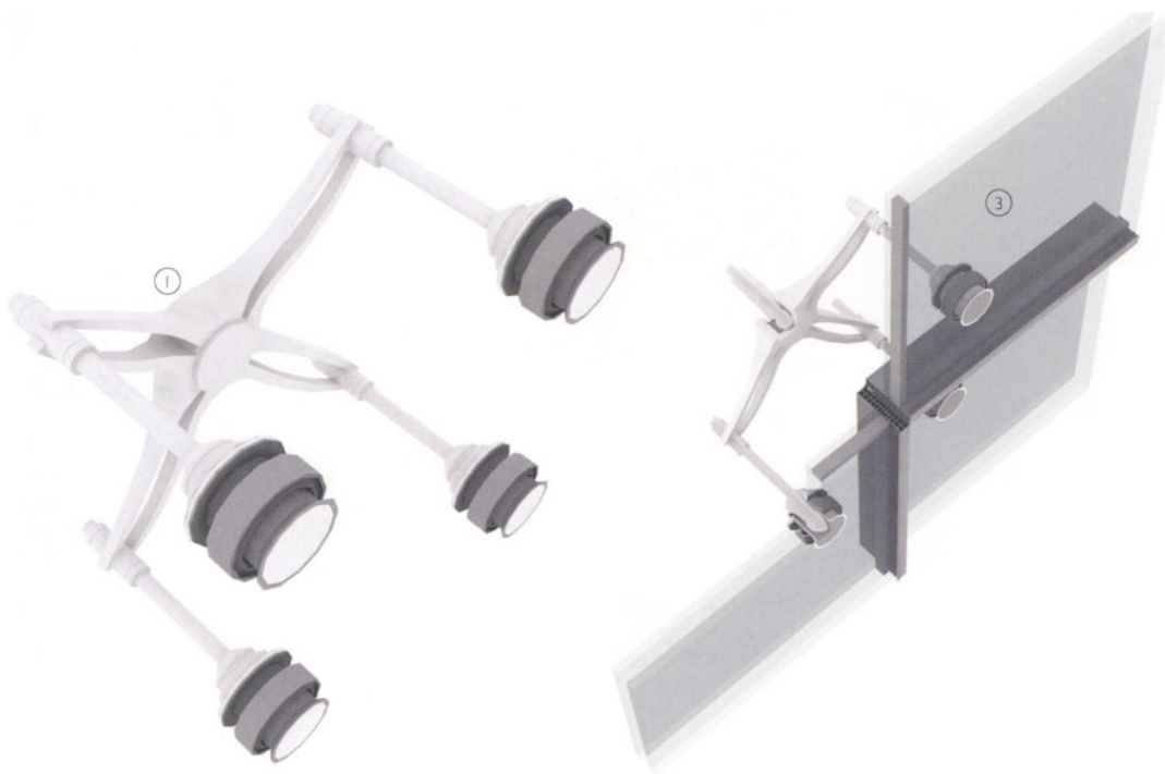
Detail of bolt fixing and 4 point glass connection
