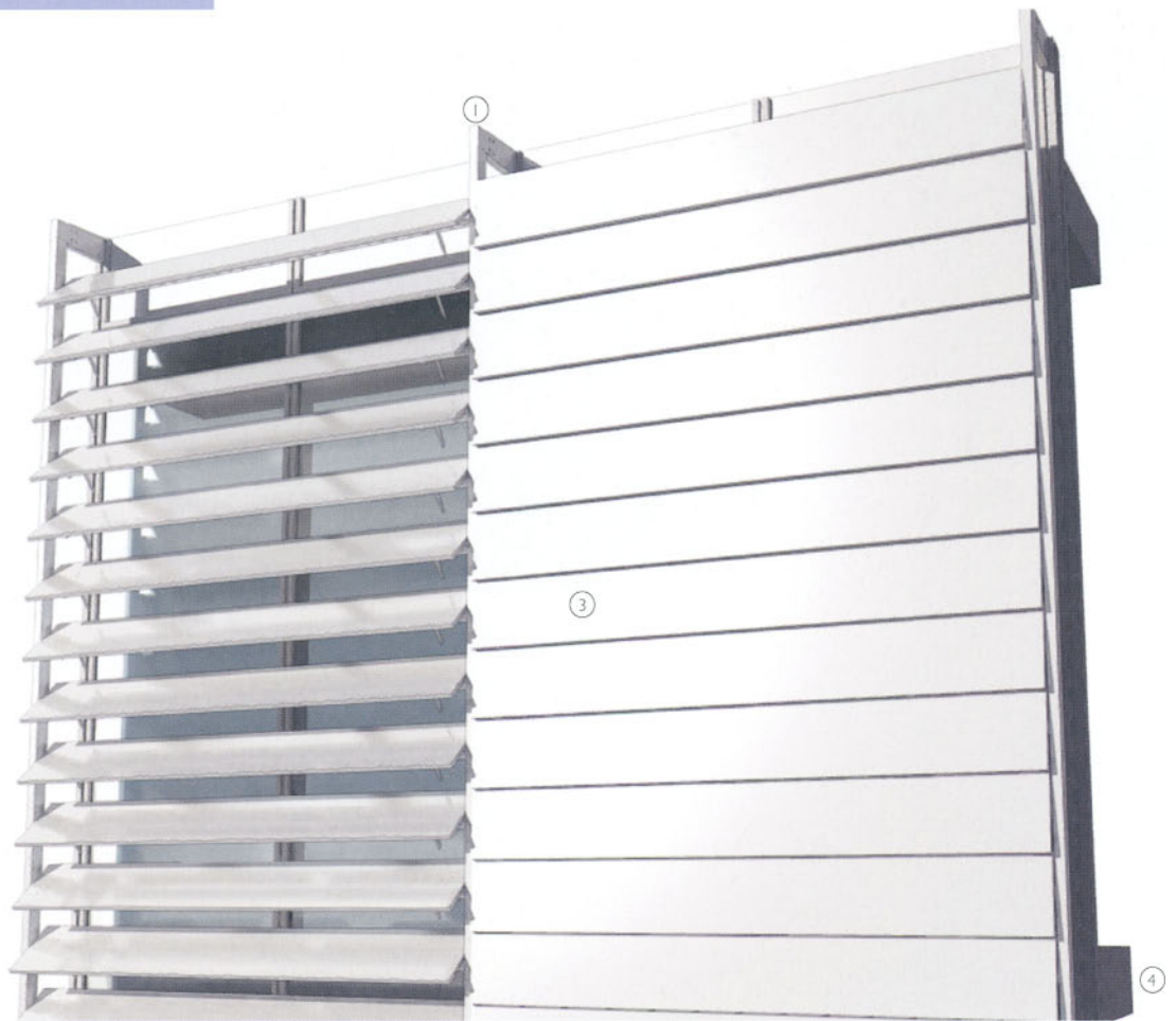
3-D view of metal louvre screen
