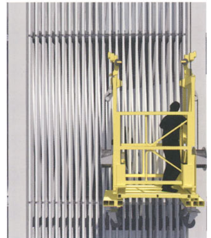
Plan 1:50 Davit supporting cradle in two positions
