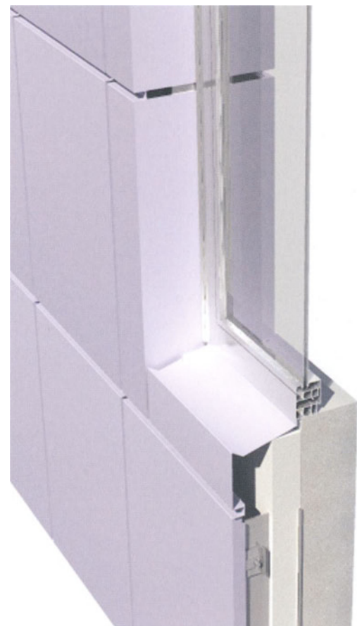
3-D view of window and parapet detail in rainscreen wall system
