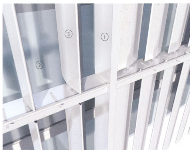
3-D views showing profiled aluminium louvres and fixing system
