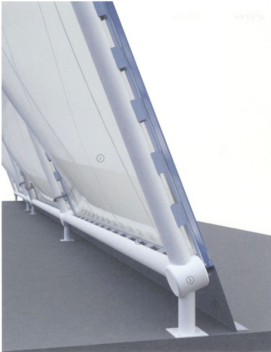
3-D detail of junction between ETFE facade and ground
