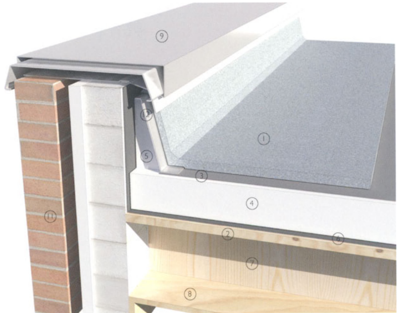
3-D view of low parapet wall
