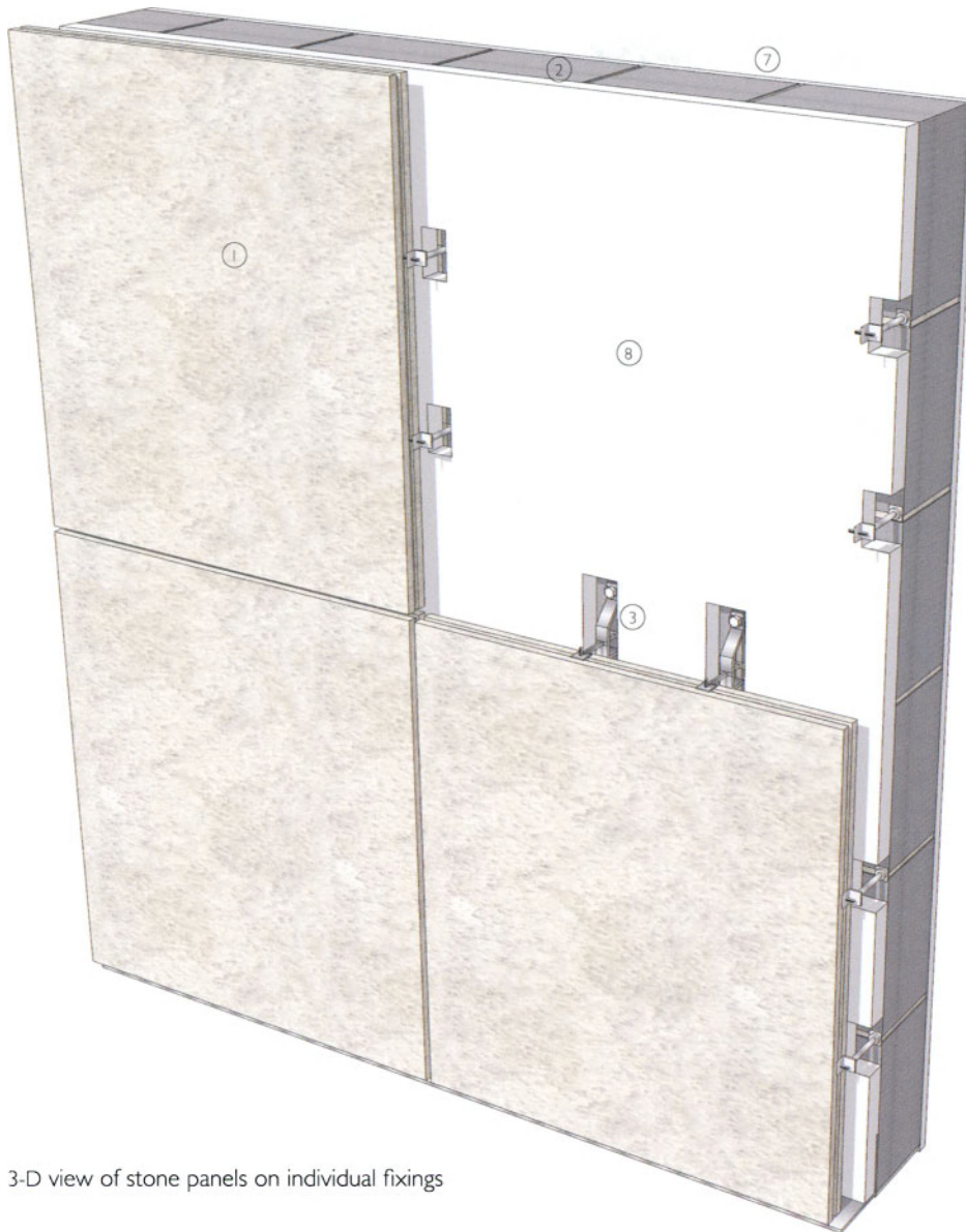
Plan 1:10. Typical stone carrier system made from extruded aluminium section
