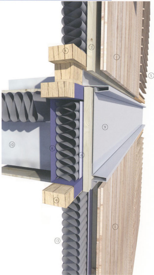
3-D view of connection between timber cladding panel and supporting frame
