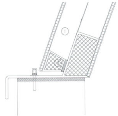
Vertical section 1:10. Junction at base
