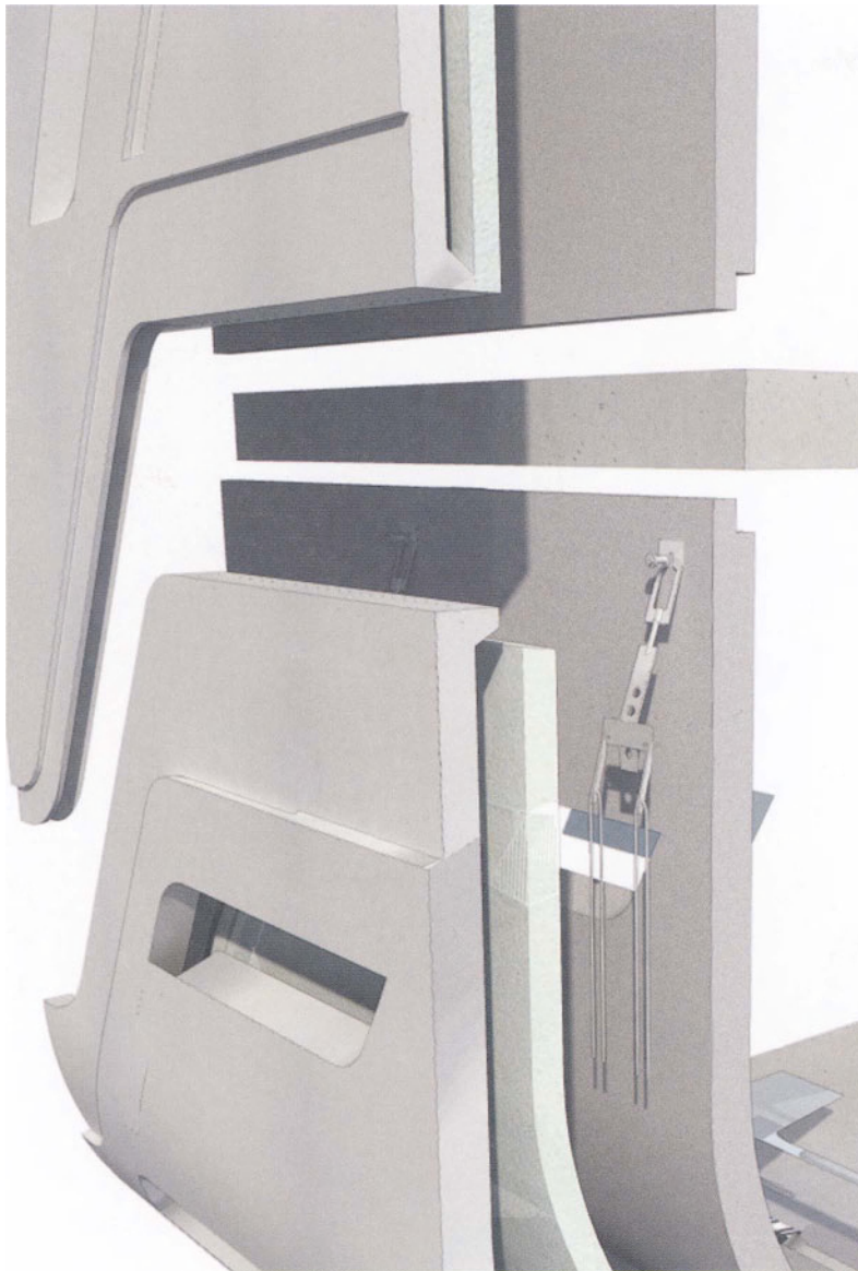
Exploded, sectional views showing the fixing system for large precast concrete cladding panels with structural reinforced concrete wall behind
