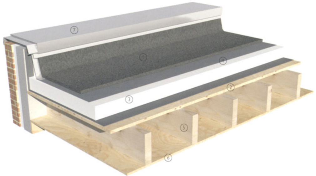
3-D overview showing typical flat timber roof construction with rigid insulation above roof structure
