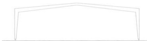
2 pin timber frame
