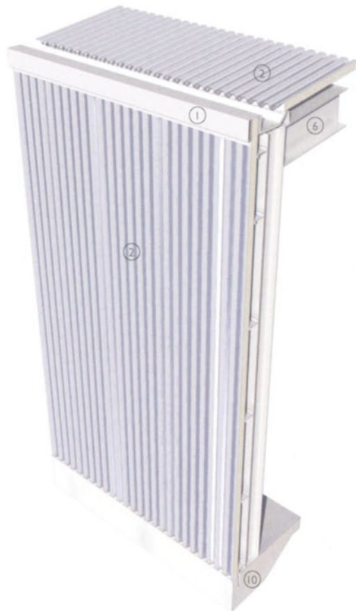
3-D view of concealed gutter
