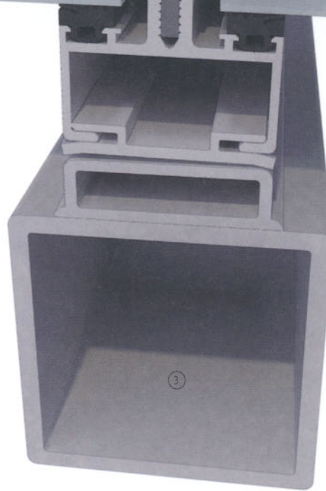
3-D view of panel to panel junction detail without capping
