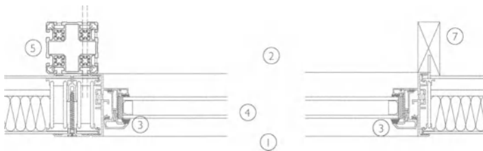
Horizontal section 1:10. Outward opening windows set within large scale window assembly
