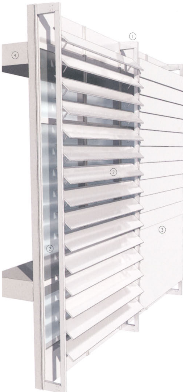
3-D view of louvre panel fixing to curtain wall system
