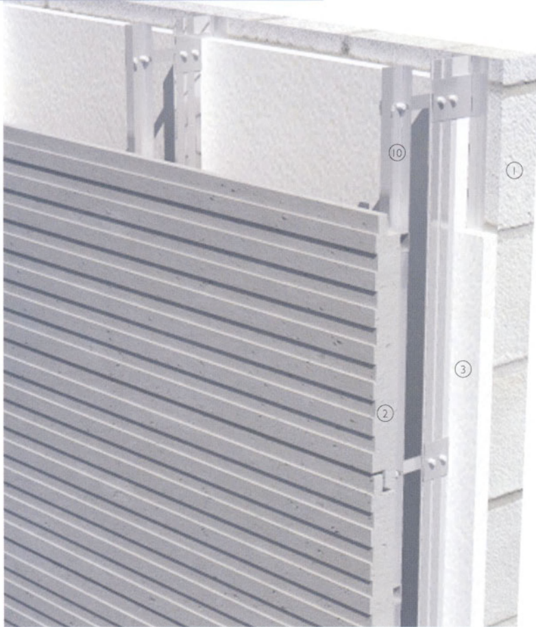
3-D view of wall assembly with profiled, precast concrete tiles
