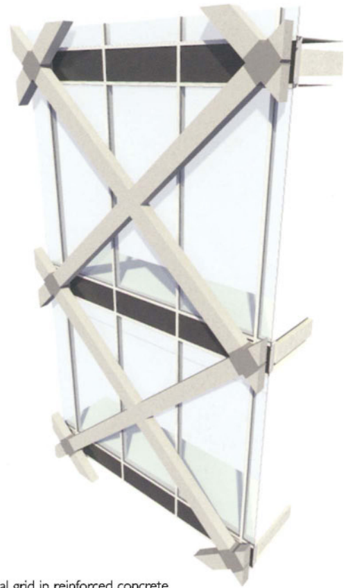
Structural facade system using a regular diagonal grid in reinforced concrete
