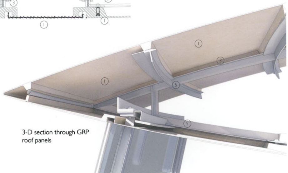
Vertical section 1:10. Panel to panel junction
