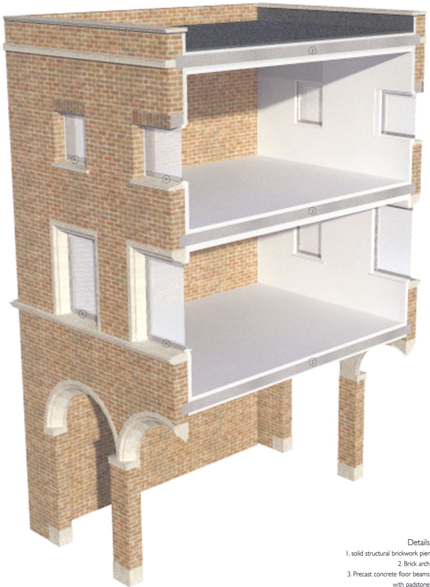
3-D sectional model showing loadbearing masonry construction
