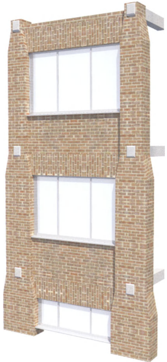
3-D elevation of typical loadbearing brick bay
