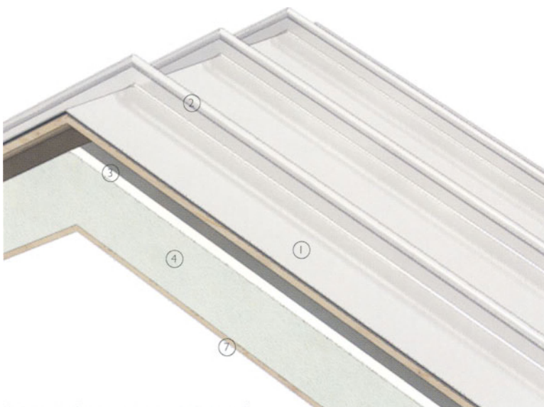
3-D view of sheet metal on timber roof
