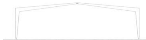
3 pin timber frame
