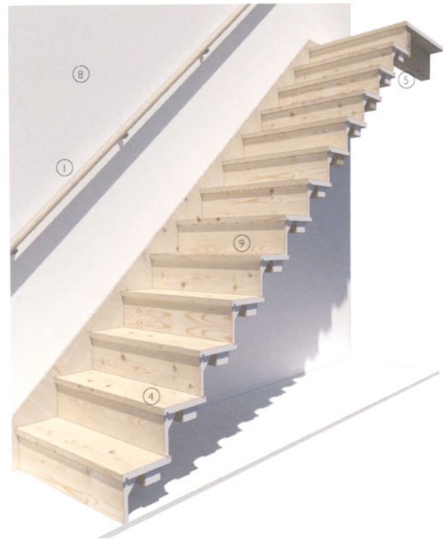
3-D view of timber stair
