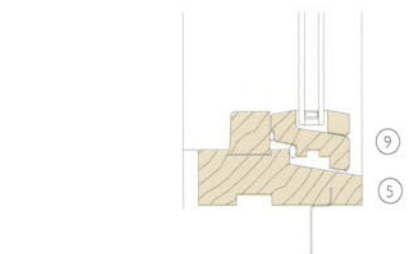
Section 1:5 Outward opening casement windows
