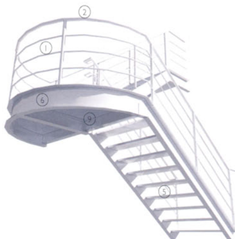
3-D view of steel stair
