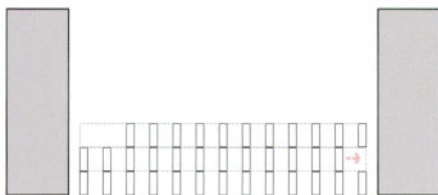
Unligned: both layers of moving system out of alignment - exposed window area = approx. 30%
