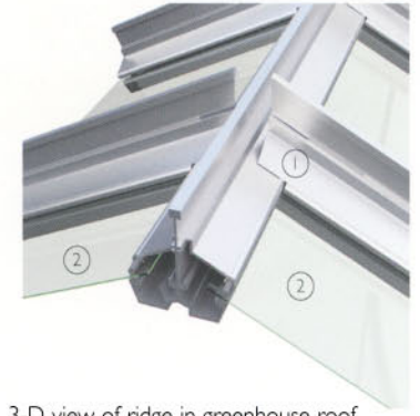
3-D view of ridge in greenhouse roof
