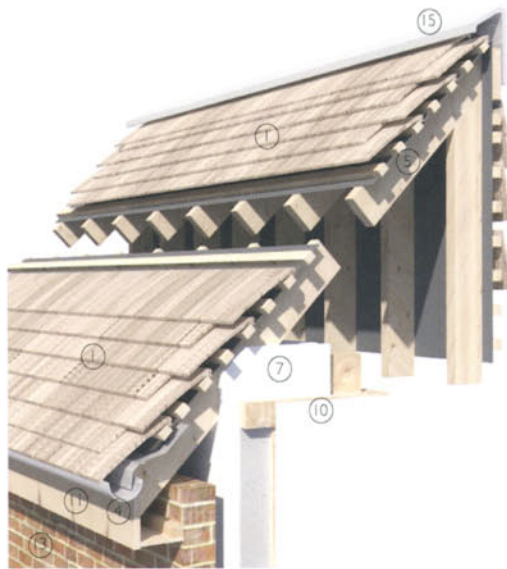
3-D view of timber shingles on timber roof construction
