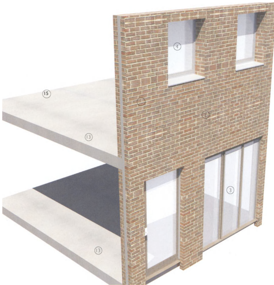
3-D view of double brick skinned cavity wall system
