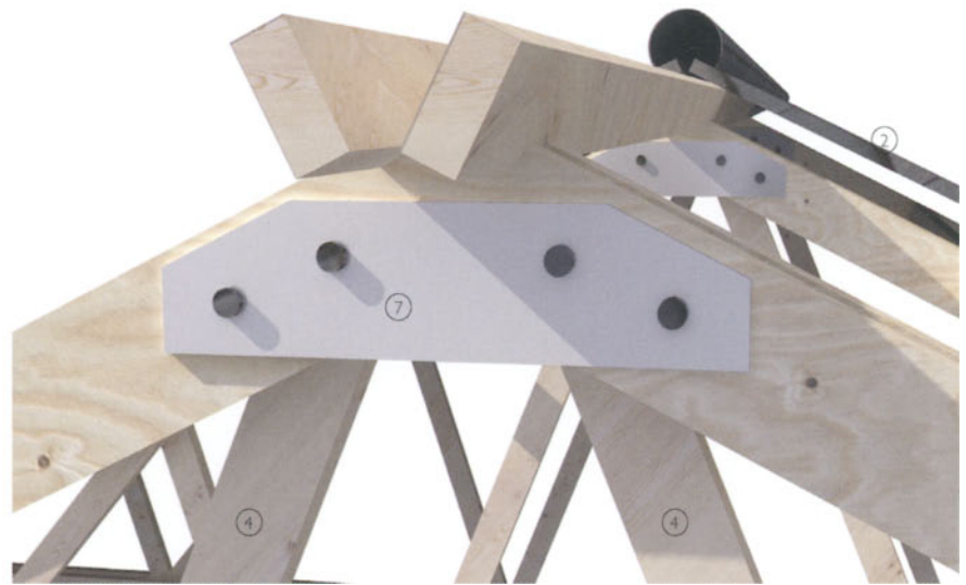
Steel plate connecting timber elements at roof ridge
