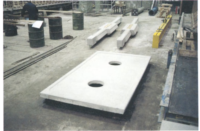
Precast floor components, from timber-based mould to floor panel, beam and panels being installed
