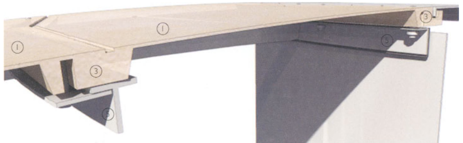
3-D detail of GRP panel connection to supporting aluminium frame
