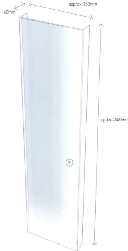
3-D view of typical glass panel vertically hung
