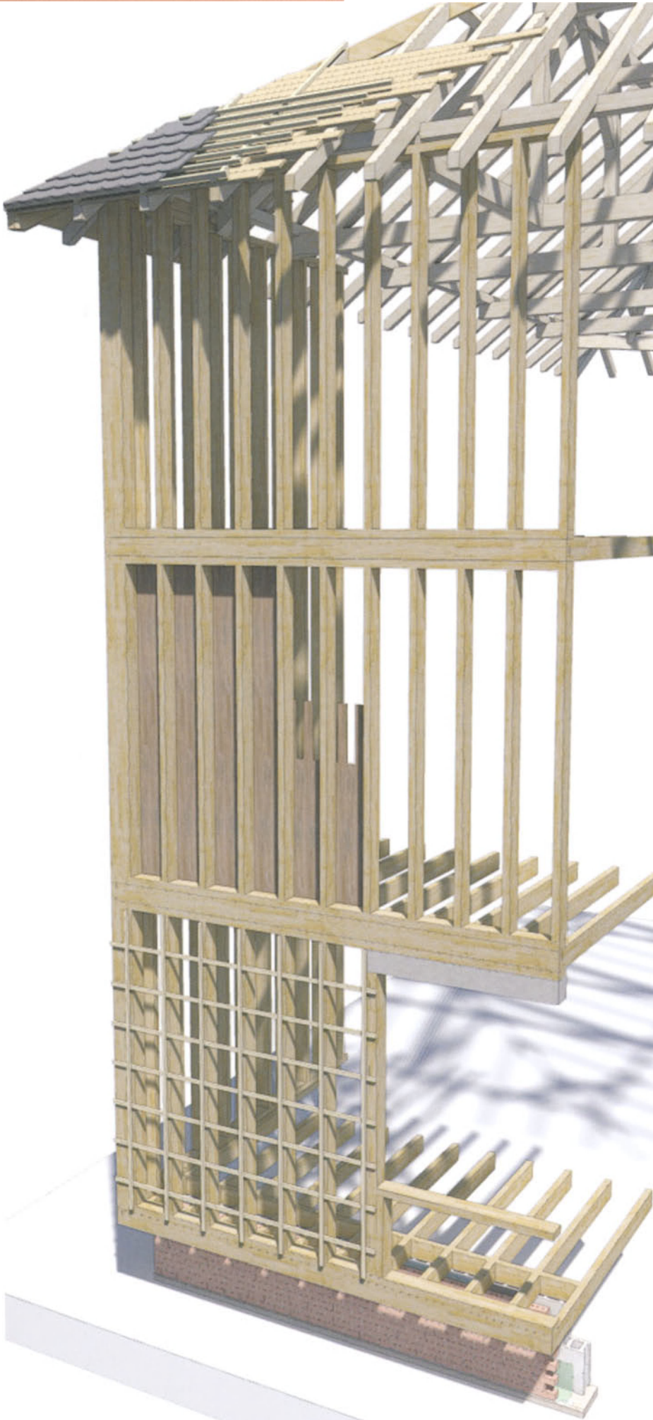
Typical timber balloon frame on a masonry base
