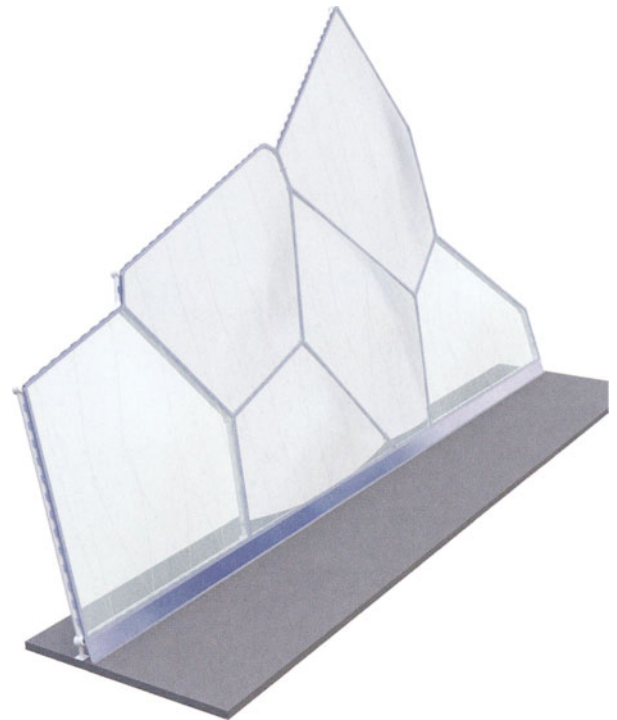
3-D Overview of irregular shaped ETFE cushions used in facade assembly
