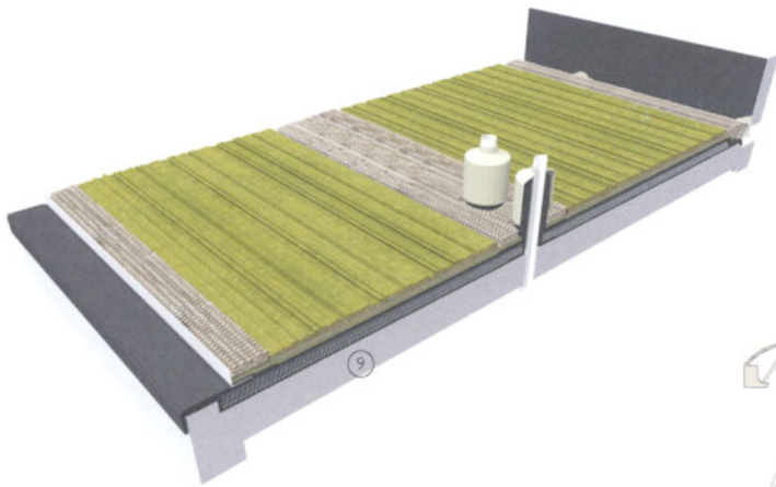
3-D overview of concrete roof with light (sedum) planting
