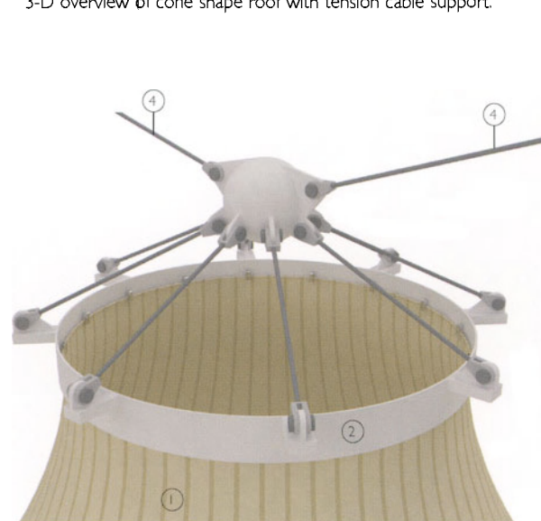
3-D detail of edge ring supported by tension cables
