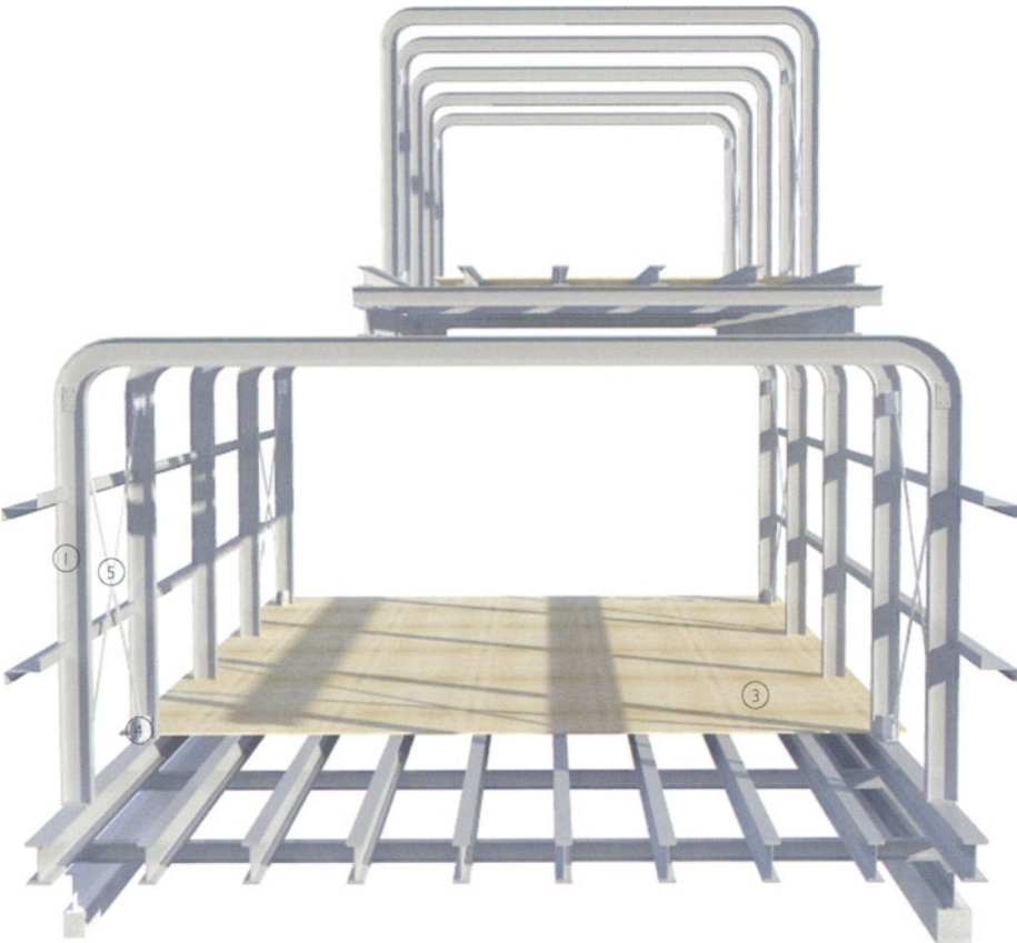
3-D section through curved brace frame construction
