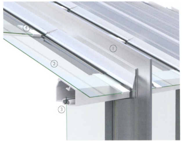
3-D view of typical eaves connection
