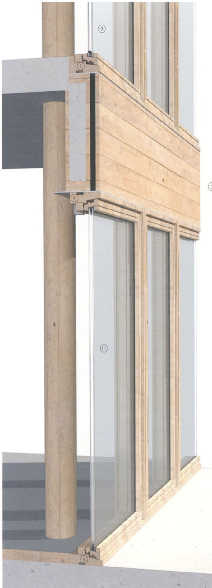
3-D view of timber doors and windows in wall system
