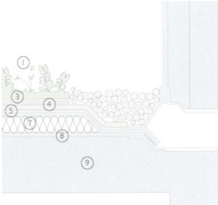
Section 1:10. Light planting. two-way outlet
