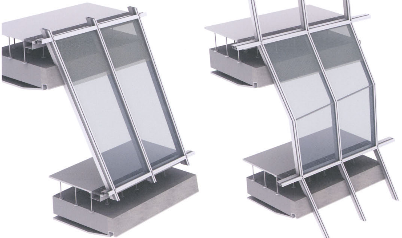
Possible methods of creating a twisted panel using flat glass
