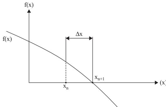
**Figure 1.9.** Newton’s second order method.
