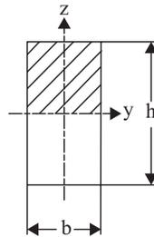
**Figure 5.14.** Example 5.12 Shear area.
