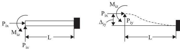
**Figure 5.16.** Geometric stiffness.
