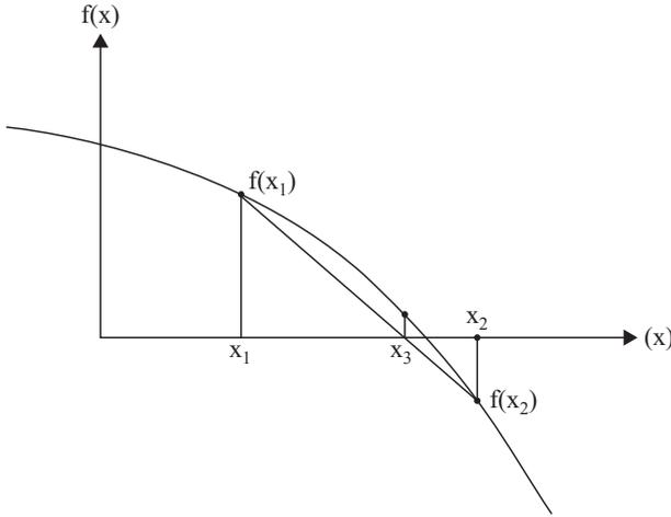
**Figure 1.4.** Method of false position or linear interpolation.
