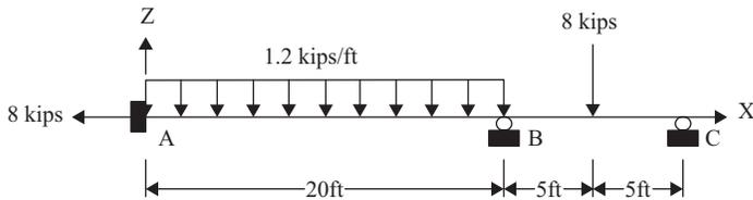
Figure 4.24. Example 4.12 Slope-deflection.
