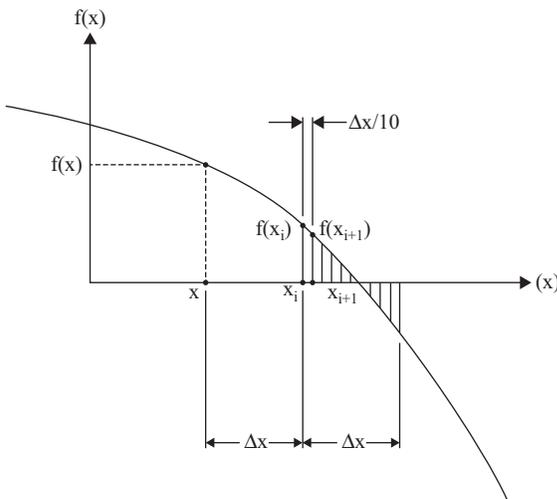
**Figure 1.2.** Refined incremental search method.
