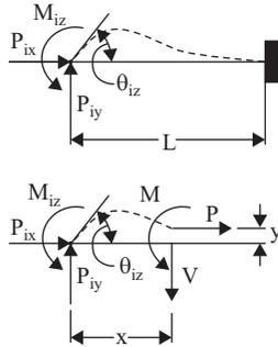
**Figure 5.18.** Example 5.15 Geometric stiffness.
