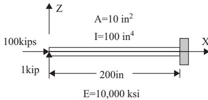
**Figure 5.20.** Example 5.17 Geometric stiffness.
