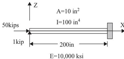
**Figure 5.19.** Example 5.16 Geometric stiffness.
