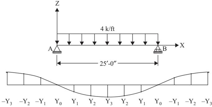
Figure 3.4. Example 3.10 Simple beam with difference operator.
