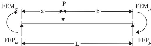
Figure 5.8. Example 5.6 Non-prismatic member stiffness.
