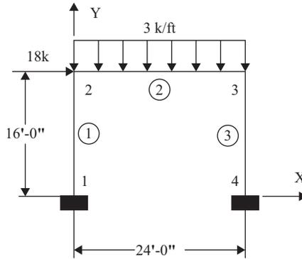
**Figure 4.35.** Example 4.20 Global joint stiffness.
