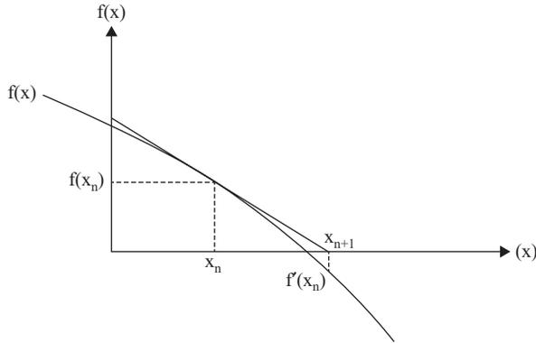
**Figure 1.6.** Newton–Raphson method or Newton’s tangent.
