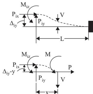
**Figure 5.17.** Example 5.14 Geometric stiffness.
