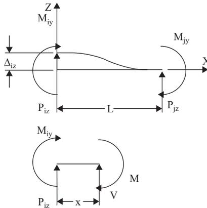
**Figure 5.11.** Example 5.9 Shear stiffness.
