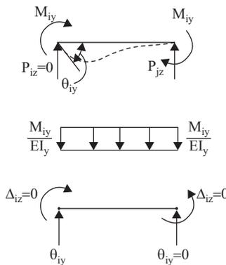
**Figure 5.1.** Example 5.1  $\Delta_{iz}$  end release.
