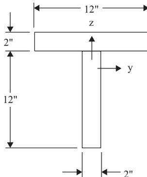
Figure 5.15. Example 5.13 Shear area.
