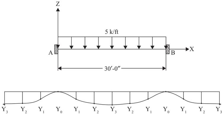
**Figure 3.7.** Example 3.11 Fixed beam with difference operator.
