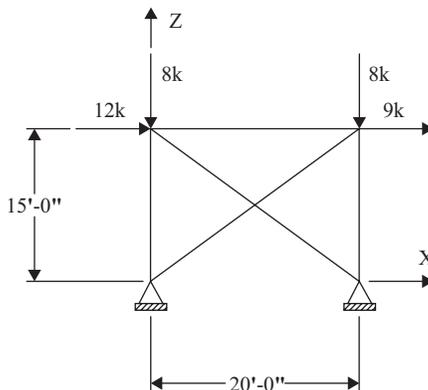
Figure 4.33. Example 4.19 Global joint stiffness.
