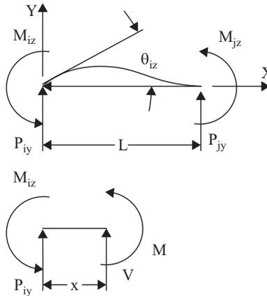
**Figure 5.12.** Example 5.10 Shear stiffness.
