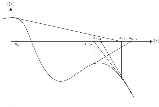
**Figure 1.8.** Newton–Raphson method or Newton’s tangent.
