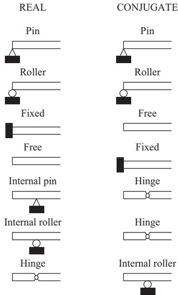
**Figure 4.12.** Conjugate versus real supports.
