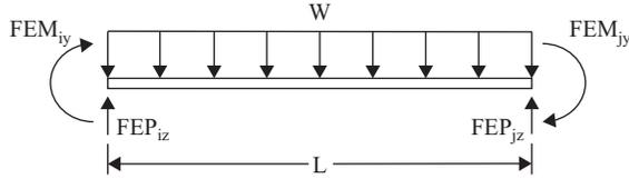
**Figure 5.7.** Example 5.5 Non-prismatic member stiffness.
