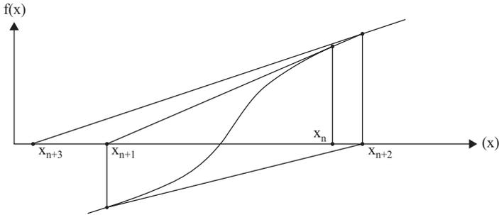
**Figure 1.7.** Newton–Raphson method or Newton’s tangent.
