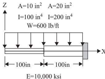
**Figure 5.9.** Example 5.7 Non-prismatic member stiffness.
