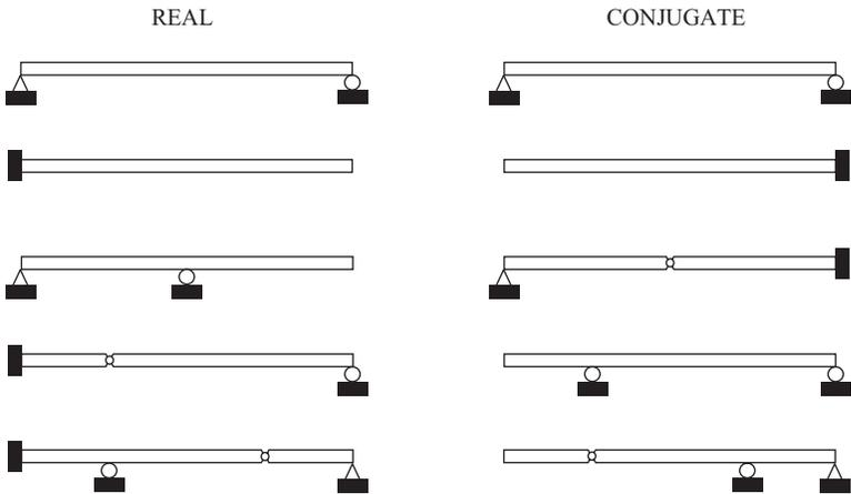
**Figure 4.13.** Conjugate versus real beams.
