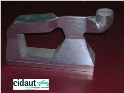
Fig.5 Solid secondary that substitutes the channel carrying molten aluminium.
