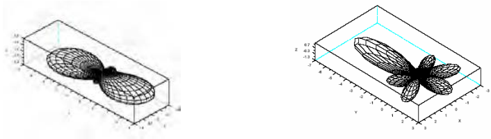
Fig.1 Radiation pattern of a dipole antenna in the presence of a human head at 900 (left) and 1800 (right) Mhz – Non uniform (4-tissues) model.
