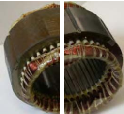
Figure 2: Stator part with semi-closed slots (right) and the novel construction without any slots (left).
