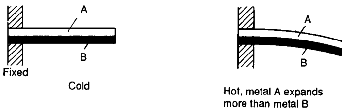
Figure 1.21 Bimetallic strip
