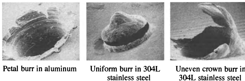
Figure 2. Burr shapes from same drill for different work materials and edge geometries
