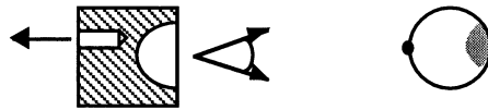
Figure 1. Visibilities of a hole and a pocket, and their representations on the sphere
