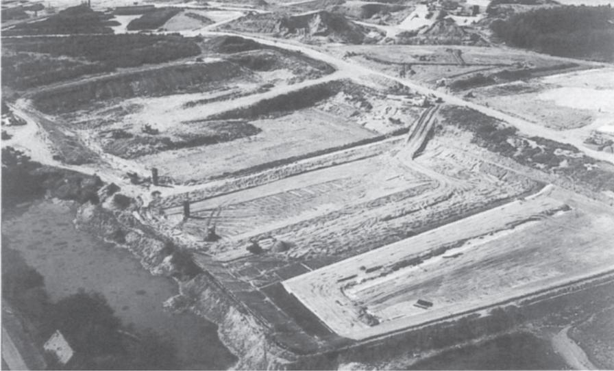
FIGURE 11.1 Landfill refuse disposal site in Belgium. This is a state-of-the-art facility with geosynthetic clay and high-density polyethylene lining to prevent leaching. Each pit can hold ca. 250,000 tonnes of waste. The gas generated during decomposition will be captured for electricity generation
