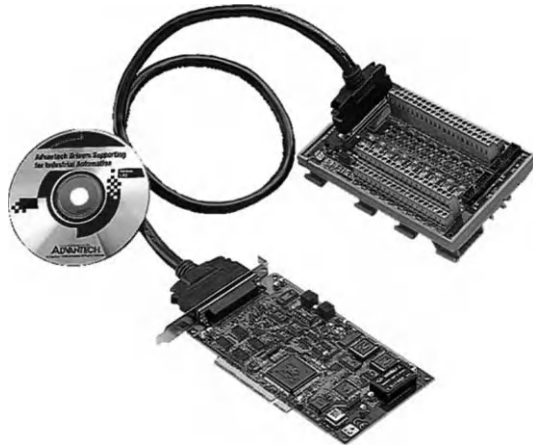
Figure 13.30. PCI 1711 Advantech data acquisition board
