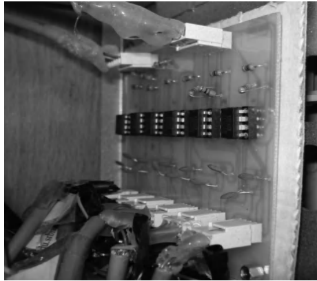
Figure 13.19. The final PCB board for recording the loadcell output
