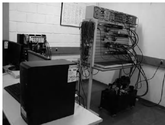
Figure 21.3. Photo of didactic laboratory for activities on hydraulic and pneumatic command systems, and industrial automation
