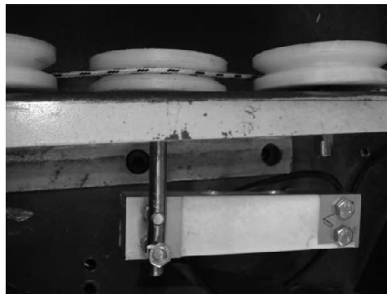
Figure 13.16. Force sensor that is connected to torque measurement mechanism
