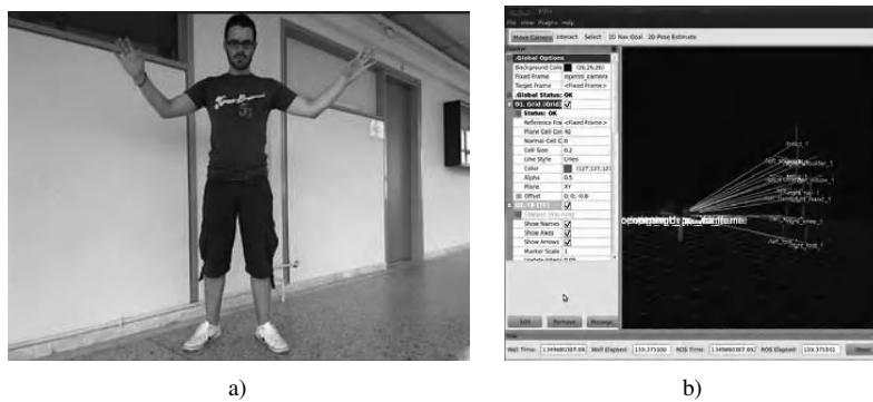
Figure 20.12. a) The color reference image of the Microsoft Kinect and b) the skeleton detection and tracking processes as illustrated on the mini-PC
