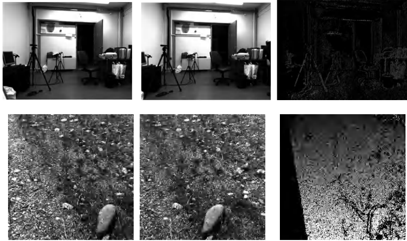
Figure 20.14. The first row depicts a stereo pair and the respective disparity of an indoor scene, while the second row depicts a stereo pair and the respective disparity map of an outdoor scene
