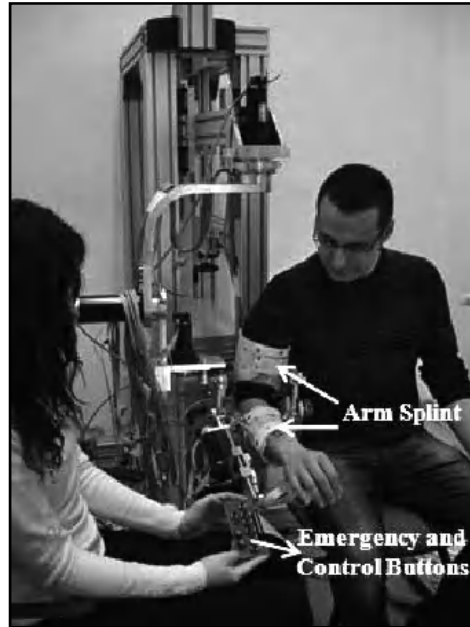
Figure 7.3. The RehabRoby system with arm splint and emergency buttons
