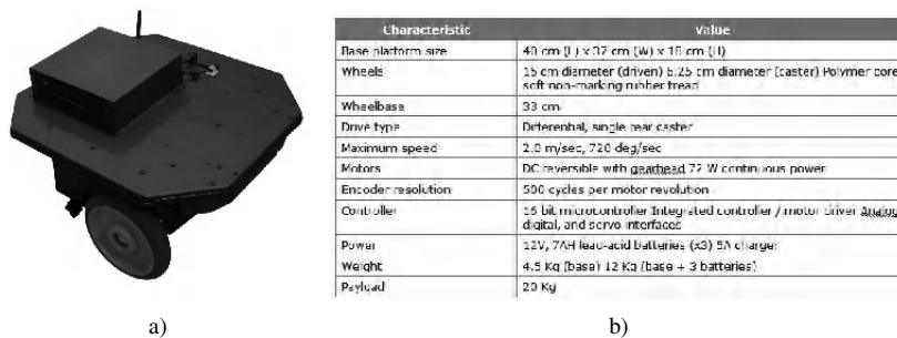
Figure 20.2. a) The Videre Erratic mobile platform and b) the respective specifications
