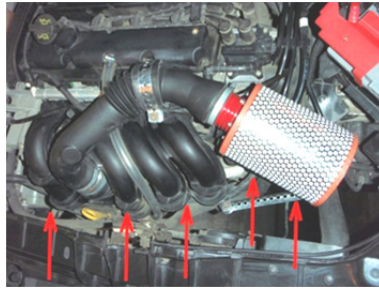
Figure 36. Filter assembly without the cooling radiator's integrated deflector
