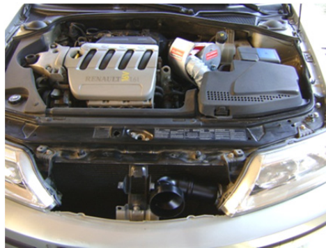
Figure 25. DATD mounted on Renault LAGUNA 1.6 16V
