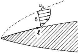
$$\mu \frac{\partial^2 u}{\partial y^2} \sim \mu \frac{u_e}{\delta^2} \quad (2.173)$$
