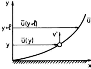
The distance along which the agglomerations lose their excess momentum is called mixing length  $l$ . Normal to the direction of the main flow the change of velocity between two layers, by the distance  $l$  apart from each other, is
