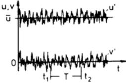
In general the time-averaged mean value of the squares and the product of the two components (correlation) of the fluctuation velocity do not vanish. When they are multiplied by the density, they have the dimension of stress. The time-averaged correlation can be interpreted as the transport of momentum per unit area in the radial direction, while the squares represent normal stresses.
