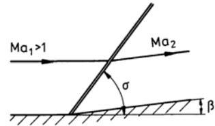
The flow quantities downstream from the shock can also be determined for a double wedge at angle of attack. With vanishing turning or nose angle of the wedge the shock intensity  $Ma_1 \sin \sigma$  tends to unity, and the shock deteriorates to a sonic line.
