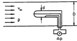
Plot  $v_\infty / \sqrt{\frac{2\Delta p}{\rho}}$  as a function of  $\frac{d}{D}$ !
