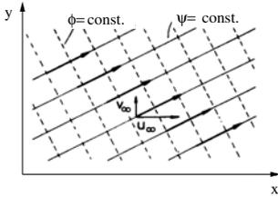
$$\frac{dy}{dx} = \frac{v_\infty}{u_\infty} = \text{const.} \quad . \quad (2.123)$$
