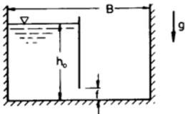
$$B = 20 \text{ m} \quad h(t=0) = h_0 = 5 \text{ m}$$
