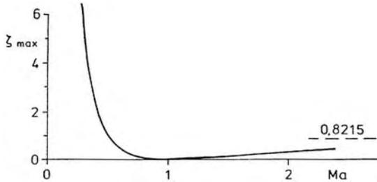
For a given perfect gas with constant specific heats the resistance coefficient  $\zeta_{max}$  depends only on the Mach number, and is - as the Mach number - therefore a state variable of the adiabatic pipe flow.
