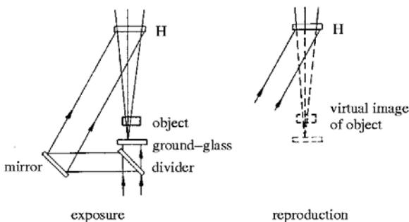
ground-glass plate. The object is behind the ground-glass plate in the diffused light. The wave fronts, passing through the object, interfere with the reference beam and are recorded on the photographically sensible layer.
