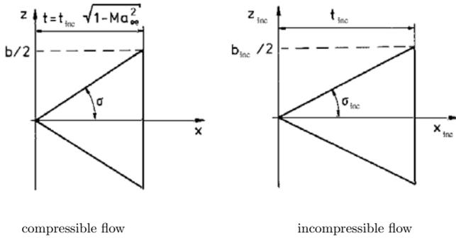
The sweep angle  $\sigma$  for compressible flows is
