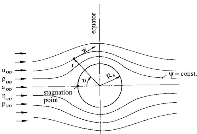
The velocity and the pressure on the surface of the sphere in incompressible flow are described by the following relations:
