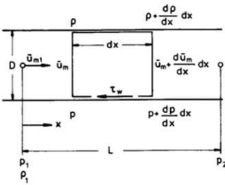
$$\begin{aligned} \rho \bar{u}_m &= \left( \rho + \frac{d\rho}{dx} dx \right) \times \\ &\quad \times \left( \bar{u}_m + \frac{d\bar{u}_m}{dx} dx \right) \\ &= \rho_1 \bar{u}_{m1} \end{aligned}$$
