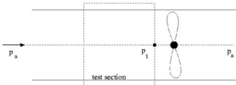
$$\begin{aligned} v_\infty &= 80 \frac{\text{m}}{\text{s}}; \quad A_{Str.} = 1.2 \text{ m}^2 \\ \Rightarrow N_{Str.} &= \frac{9}{2} A_{Str.} v_\infty^3 = 384 \text{ kW} \\ N_{eff} &= 180 \text{ kW} \text{ Göttingen-type tunnel} \\ Ma &= 0.24 \Rightarrow \text{air} \approx \text{incompressible} \end{aligned}$$
