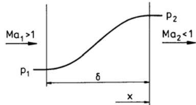
The increase of the entropy can now be explained as an action of the frictional forces and the heat conduction within the shock region of finite thickness. The conservation equations for one-dimensional, steady, viscous, and heat conducting flow are
