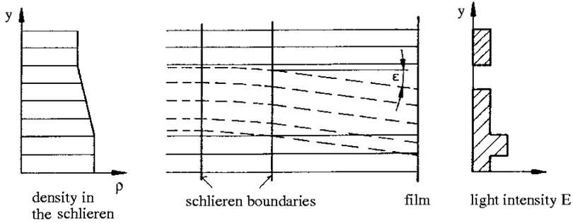
It is clear from the sketch above, that a constant density gradient in the phase object deflects the entire incident light, but does not change the distribution of the light intensity on the film. Only a change of the density gradient leads to a brightening and darkening of parts of the image. The light intensity is approximately given by
