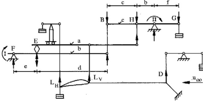
In the diagrammatic sketch the equilibrium condition for the individual systems (beams of balance) is given: The external forces  $L_H$  and  $L_V$  act on the beam of balance in the middle (a), and the equilibrating forces are  $D$  and  $H$ .
