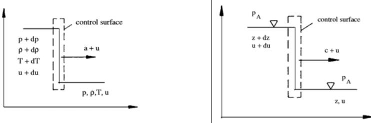
The changes of conditions generated by the wave element appear to be steady to an observer moving with the control surface. For this frame of reference the fundamental equations can be formulated for steady flow:
