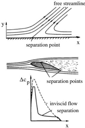
At the  $x$ -position, where  $\tau_w = 0$ , the flow separates from the body contour. The reversed flow often leads to formation of vortices downstream from the separation point. In the separated region, also called recirculation or dead-water region, the boundary layer equations are no longer valid. The wall-shear stress can only be determined up to the separation point.
