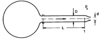
$$\begin{aligned} L = 100 \text{ m} \quad D = 10^{-2} \text{ m} \\ d = 0.5 \cdot 10^{-2} \text{ m} \quad p_a = 10^5 \frac{\text{N}}{\text{m}^2} \\ p_1 = 1.075 \cdot 10^5 \frac{\text{N}}{\text{m}^2} \quad \rho = 10^3 \frac{\text{kg}}{\text{m}^3} \\ \mu_1 = 10^{-3} \frac{\text{Ns}}{\text{m}^2} \end{aligned}$$
