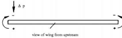
Since the lift vanishes at the wing tips, the circulation has to satisfy the condition  $\Gamma(y = \pm b/2) = 0$ . For this reason the circulation distribution over the span is assumed to be given by a discontinuous step curve with small increments  $\Delta\Gamma$ ; the vortex elements of strength  $\Delta\Gamma$  leave the wing in the downstream direction as free vortices, shown in the following sketch, and form a vortex sheet, which rolls up into the two free tip vortices.
