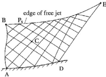
With the procedure described, the flow in the region  $B - D - E$  can be determined, one side of which is bounded by the edge of the jet (free boundary), and the other by the Mach line, originated in the point  $D$ . If the boundary conditions downstream from the points  $D$  and  $E$  are known, the computation of the flow can be continued.
