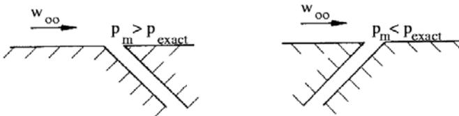
2. The roughness, or burr, and chamfers or radii at the edge of the borehole disturb the flow in the borehole and falsify the measurement.
