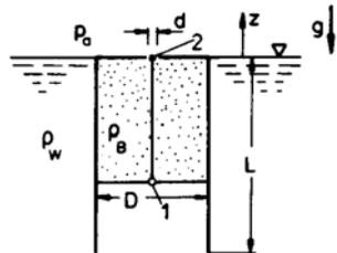
$$p_1 + \rho_B g z_1 + \frac{\rho_B}{2} v_1^2 = p_a + \frac{\rho_B}{2} v_2^2$$
