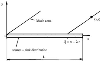
The change of the upper limit of integration is necessitated by the finite extent of the region of influence of supersonic flows. A point  $P(x, r)$  on the surface of the Mach cone, given by  $\xi = x - \lambda r$ , cannot be influenced by the sources and sinks further downstream.
