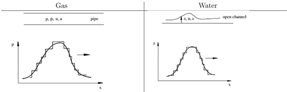
Consider a continuous solitary wave of finite amplitude in the sketch. It is approximated by a sequence of a finite number of wave elements, in which the flow conditions are changing discontinuously.
