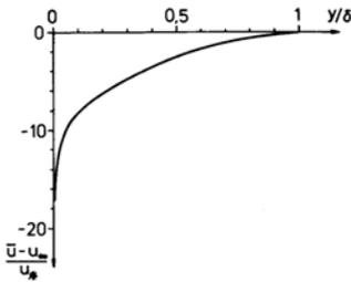
which is shown in the diagram. With the universal law of the wall and the von Kármán integral relation the drag coefficient of the flat plate can be determined as a function of the Reynolds number.
