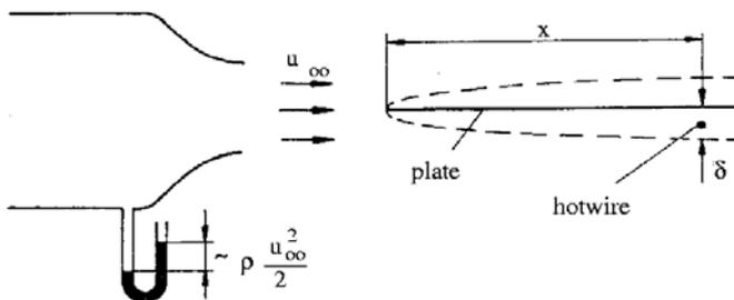
In the experiment the hot wire is positioned shortly upstream of the trailing edge of the plate in the boundary layer. Its signal is recorded with an oscillograph. If the velocity  $u_\infty$  is slowly increased, the following signals are observed:
