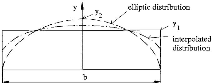
It is to be noted, that the Schrenk approximation does not drop to zero at the end of a rectangular wing. The error is of minor importance, if one remembers the simplicity of the method.
