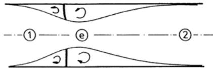
For low Mach numbers  $Ma_1$  the friction coefficient depends only on the Reynolds number, i. e.  $\zeta_O = \zeta_O(Re)$ . It is almost constant. With increasing Mach number  $Ma_1$  the friction coefficient also depends on the Mach number, i. e.  $\zeta_O = \zeta_B(Re, Ma)$ , increasing only slightly until the speed of sound is reached in the narrowest cross section near the orifice ( $Ma_e = 1$ ) for the so-called critical inflow Mach number  $Ma_{1crit}$ .
