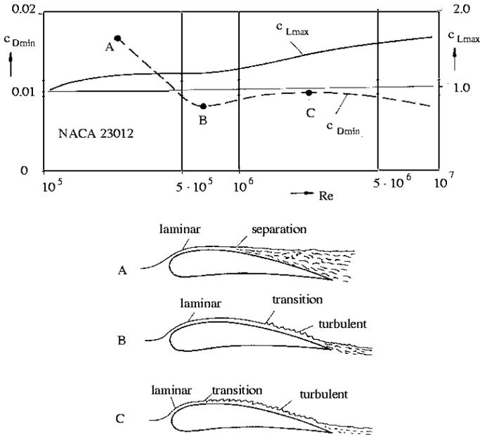
The dependence of the aerodynamic force coefficients (e. g.  $c_{Dmin}$  and  $c_{Lmax}$ ), and of the behavior of the boundary layer on the Reynolds number  $Re$  is briefly discussed for the profile NACA 23012 with the following diagrams.
