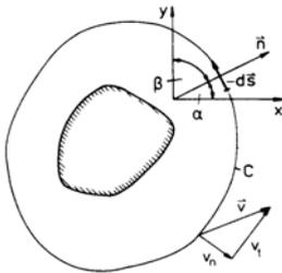
The force acting on an arbitrary body can be determined with the momentum theorem. If the local pressure is eliminated with Bernoulli's equation, the momentum equation yields the force acting on the body.
