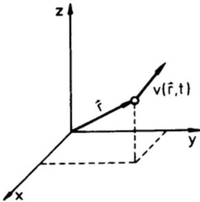
The motion of the fluid is completely determined, if the velocity  $\mathbf{v}$  is known as a function of time everywhere in the flow field
