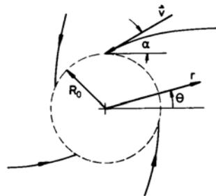
$$\begin{aligned} \Psi &= \frac{E}{2\pi} \theta - \frac{\Gamma}{2\pi} \ln \frac{r}{R} \\ v_r &= \frac{E}{2\pi r} \\ v_\theta &= \frac{\Gamma}{2\pi r} \end{aligned}$$
