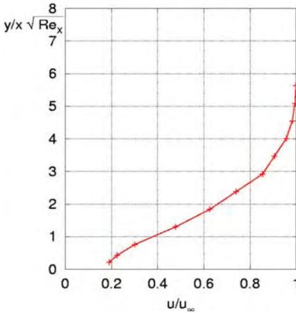
laminar boundary layer on a flat plate
