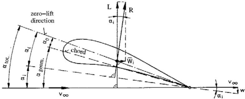
The local lift is now no longer determined by the geometric angle of attack  $\alpha_{geom}$ , but by the local “effektive” angle of attack  $\alpha_i = \alpha_e$ .
