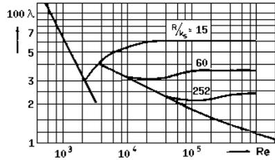
The diagram shows the influence of the relative sand roughness on the pipe friction coefficient. According to this diagram, above a certain Reynolds number the friction coefficient  $\lambda$  depends only on  $k_s/R$ . For completely rough pipes the quadratic resistance law is valid and the pipe friction coefficient can be determined by the following relation.
