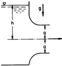
For  $\frac{a}{h} \rightarrow 0$  the volume flow per unit time is  $\dot{Q}_0 = 2 a B \sqrt{2 g h}$ . Determine the relative error  $\frac{\dot{Q}_0 - \dot{Q}}{\dot{Q}}$  for  $\frac{a}{h} = \frac{1}{4}$ ,
