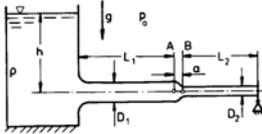
$$p_a = 10^5 \frac{\text{N}}{\text{m}^2} \quad L_1 = L_2 = 5 \text{ m} \gg a$$
