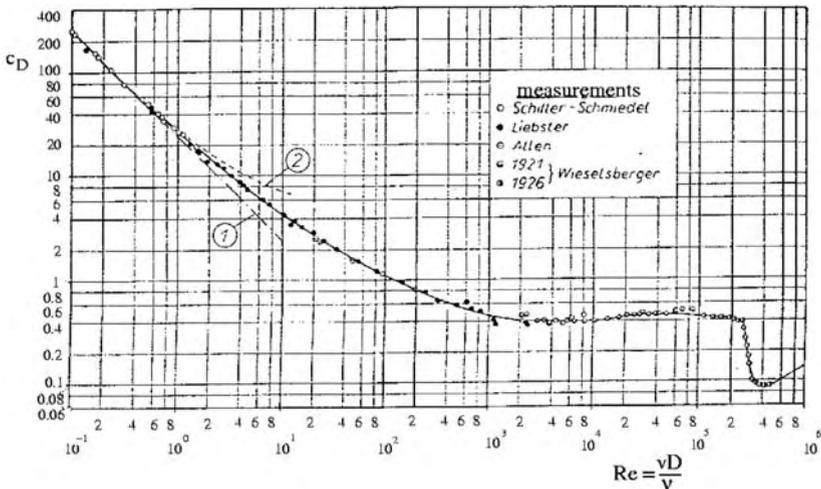
The above diagram shows the drag coefficient as a function of the Reynolds number after H. Schlichting [1982]; curve(1): Theory of Stokes; curve(2): Theory of Oseen.
