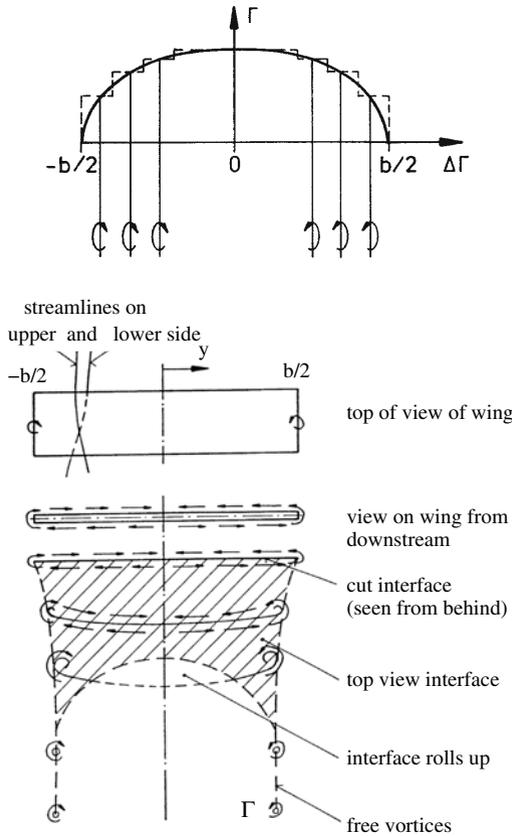
At every position  $y$  on the wing a downwash velocity  $w_i(y)$  and thereby an angle of attack  $\alpha_i(y)$  is induced; according to the Biot-Savart law they are
