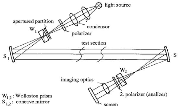
The light of the source is focussed by a condenser in a point, which is so chosen that it coincides with the focus of a concave reflector. The light rays leaving the reflector are parallel to each other. They pass the test section and are focussed again by a second reflector. Special imaging optics are required to depict the test section in a suitable size on the film.
