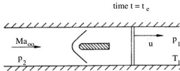
$$p_1 = 10^5 \text{ Pa}; \quad T_1 = 300 \text{ K}; \quad \gamma = 1.4;$$
