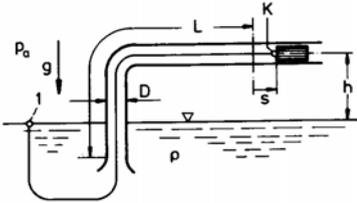
$$\begin{aligned} p_a &= p_p + \rho g h + \frac{\rho}{2} v_p^2 \\ &\quad + \rho \int_{s_1}^{s_p} \frac{\partial v}{\partial t} ds \\ \int_{s_1}^{s_p} \frac{\partial v}{\partial t} &\approx L \frac{dv_p}{dt} \quad \left( \frac{s_0}{L} \ll 1 \right) \\ p_p &= p_a - \rho g h + \rho s_0 \omega^2 \times \\ &\quad \left[ L \sin \omega t - \frac{s_0}{2} \cos^2 \omega t \right] \\ p_{pmin} &= p_v \\ p_p &= p_{pmin} \text{ with } \cos \omega t = 0 \end{aligned}$$
