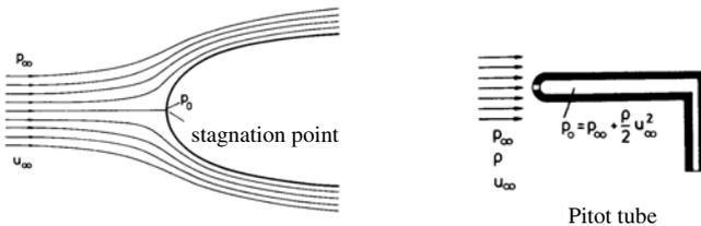
It follows from Bernoulli's equation that the pressure in the stagnation point (total pressure  $p_0$ ) is equal to the sum of the static pressure  $p_\infty$  and of the dynamic pressure  $\rho u_\infty^2/2$  of the oncoming flow. The total pressure can be determined with the Pitot tube, the opening of which is positioned in the opposite direction of the flow.
