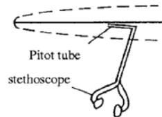
In this experiment the velocity  $u_\infty$  is kept constant, and the Pitot tube is held at a constant distance from the wall and moved downstream. The coordinate  $x$ , where a clear high-frequency crackling is first heard, is used for determining the critical Reynolds number.
