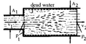
The pressure loss is obtained with the control surface shown in the sketch above by the dashed line to
