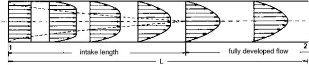
In the intake region an additional pressure loss arises, which can be described by a loss coefficient ( $\zeta_i \approx 1.16$ )
