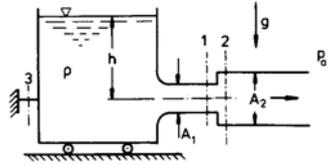
$$h = 5 \text{ m} \quad A = 0.1 \text{ m}^2 \quad p_a = 10^5 \frac{\text{N}}{\text{m}^2}$$
