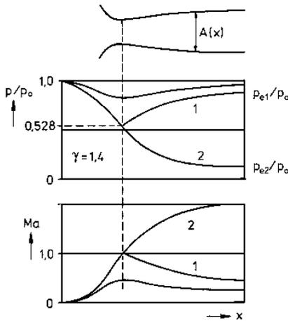
If the pressure in the exit cross section is between  $p_{e1}$  and  $p_{e2}$ , the flow cannot adjust isentropically to the conditions existing in the exit cross section. Then a discontinuous increase of the density, pressure, and temperature occurs in the supersonic part of the nozzle, known as normal compression shock. The flow is decelerated to subsonic speed. This discontinuous process causes losses, which result in an increase in entropy.
