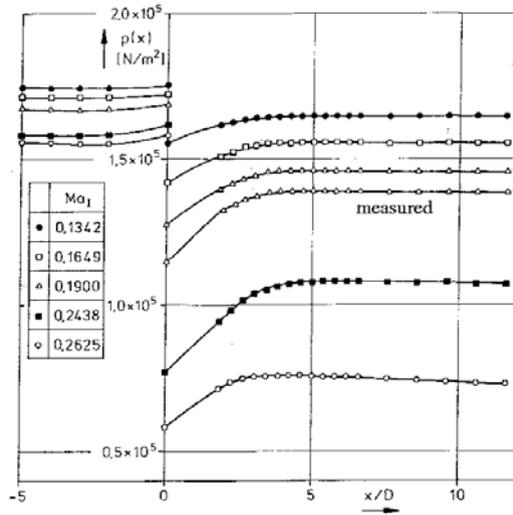
2. The resistance coefficient of the orifice, the ratio of the stagnation pressures  $p_{0II}/p_{0I}$ , and the increase of entropy  $\Delta S_{II}/R$  are to be plotted in the corresponding diagrams.
