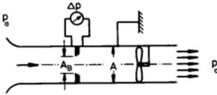
$$p_a = 10^5 \frac{\text{N}}{\text{m}^2} \quad \Delta p_w = 300 \frac{\text{N}}{\text{m}^2}$$
