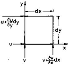
The flux of vorticity is closely related to the circulation  $\Gamma$ , being defined as the line integral extended over the scalar product of the velocity and the line element of a closed curve  $C$ .
