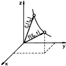
The path line begins at time  $t = t_0$  at a point defined by the position vector
