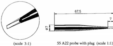
A single hot-wire probe is shown above. The wire has a diameter of the order of  $5 \mu\text{m}$ . Modern hot-wire anemometers measure all three velocity components with three wires, orthogonally arranged to each other in a measuring volume of about  $1 \text{ mm}^3$ , gold-soldered to six prongs, which lead the electric current to the bridge.
