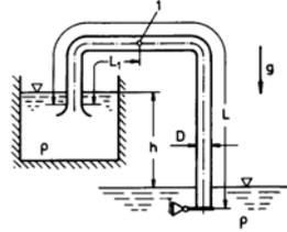
$$L = 20 \text{ m} \gg D \quad h = 5 \text{ m} \quad L_1 = 5 \text{ m}$$
