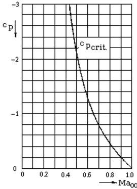
7.7 Consider a transonic flow at  $Ma_1 = 0.95$  about a wing section with the relative thickness  $\delta_1 = 0.05$ . The minimum pressure on the contour is measured to be  $c_{p1min} = 0.3$ . Use the von Kármán similarity rule and compute the relative thickness  $\delta_2$  and the pressure coefficient  $c_{p2min}$  of a second wing section for a free-stream Mach number  $Ma_2 = 0.9$ .
