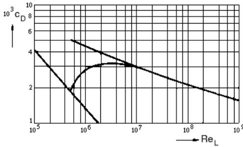
The following interpolation formula suggested by Prandtl can be used for the transition regime from laminar to turbulent flow
