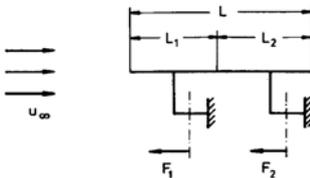
$$\begin{aligned} u_\infty &= 1 \frac{\text{m}}{\text{s}} \quad L = L_1 + L_2 = 0.36 \text{ m} \\ B &= 1 \text{ m} \quad \rho = 10^3 \frac{\text{kg}}{\text{m}^3} \quad \nu = 10^{-6} \frac{\text{m}^2}{\text{s}} \end{aligned}$$
