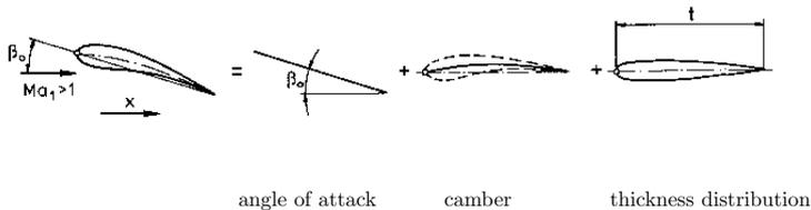
The local angle of attack consists out of three parts: The angle of attack of the chord  $\beta_0$ , the angle of attack of the mean camber line  $\Delta\beta_c(x)$  with respect to  $\beta_0$ , and the angle of attack of the thickness distribution  $\Delta\beta_t(x)$ , with respect to the mean camber line
