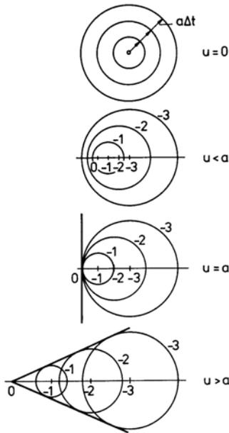
in the space downstream from the source, and for supersonic speed, the sound can spread out only in the so-called Mach cone, the half angle of which is given by
