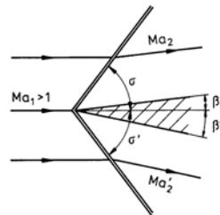
A closed-form solution of the conservation equations does not exist for the flow field between the bow shock and the wedge. In a certain point on the shock, the tangent of the shock is normal to the direction of the free-stream velocity.
