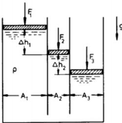
$$F_1 = 1100 \text{ N} \quad F_2 = 600 \text{ N} \quad F_3 = 1000 \text{ N}$$
