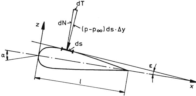
The length element in the spanwise direction  $\Delta y$ , for example, is chosen to be  $1\text{ m}$ . The normal component is:
