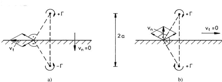
3. A vortex in the vicinity of the edge of a free jet is generated by mirror imaging of a vortex of the same circulation and the same direction of rotation (see afigure above).
