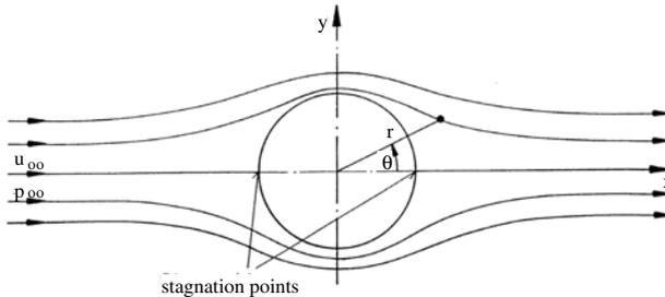
The pressure distribution is symmetric with respect to the  $y$ -axis; it follows that the resulting drag force is zero – in contrast to all experience – (*The d'Alembert Paradox*).
