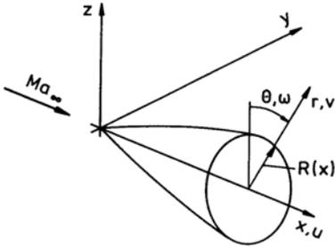
The linearized potential equation for bodies of revolution, in comparison to plane flows, contains an additional term, which results from the continuity equation, written in cylindrical coordinates: For a volume element of the flow in cylindrical coordinates the mass balance for steady flow yields the continuity equation in the following form
