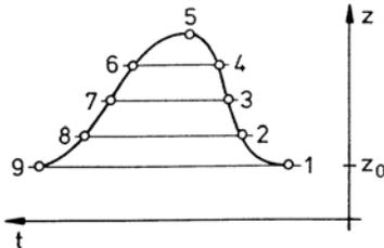
The initial wave (measuring position I) is to be subdivided into at least 8 sections, for which the theoretical propagation velocity is to be determined. The change of the shape of the wave, which would result from the propagation of the wave through the open channel is to be compared with the measured values.
