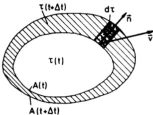
For steady flows the time rate of change of momentum is given by the surface integral of the last equation. The surface  $A$  of the volume  $\tau$  considered is called control surface. The external forces, which are in equilibrium with the time rate of change of momentum, are volume and surface forces, for example, volume forces due to the gravitational force:
