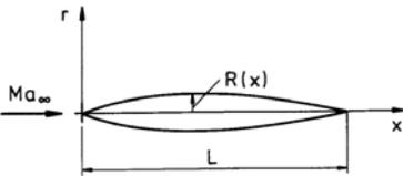
If the contour of the body is specified by a certain distribution of the local radius over the length of the body  $L$ , the exact boundary condition is
