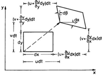
$$\dot{\epsilon}_x = \frac{\partial u}{\partial x} \quad \dot{\epsilon}_y = \frac{\partial v}{\partial y} \quad \dot{\epsilon}_z = \frac{\partial w}{\partial z} \quad (2.20)$$
