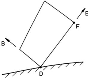
Then the computation begins in the point  $F$ , which is assumed to lie on the characteristic curve through the point  $D$  in its vicinity. The computation is continued in the direction towards the free boundary along the characteristic  $D - B$ . The flow in the region  $A - B - D$  is not influenced by the flow condition prescribed.
