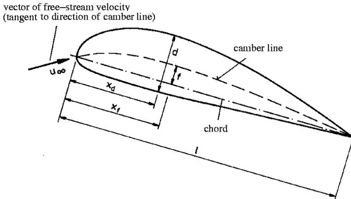
Chord of the profile  $l$ : The characteristic parameter, to which all dimension sizes are referenced. Maximum relative profile thickness  $d/l$ ; relative thickness position  $x_d/l$ ; maximum relative camber  $f/l$ ; relative camber position  $x_f/l$ .
