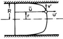
For the fully developed turbulent pipe flow the splitting of the component in the axial direction yields
