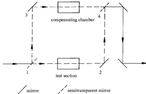
If the reflectors 2 and 4 are not turned, the light rays pass through. A phase difference is generated and thereby an interference field.
