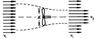
$$A' = 7.06 \text{ m} \quad v_1 = 5 \frac{\text{m}}{\text{s}} \quad v_2 = 8 \frac{\text{m}}{\text{s}}$$
