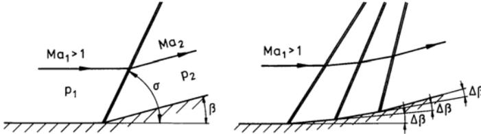
If the compression is designed in such a way, that the turning of the flow is the same in both cases, i. e.  $\beta = n \Delta \beta$ , then the pressure after the  $n$ -th turning is
