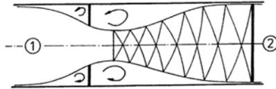
The resistance coefficient of the orifice attains its maximum value  $\zeta_{Omax}$ , if the supersonic flow extends to the wall of the pipe. A further increase of the Mach number beyond  $Ma_{1max}$  is not possible.
