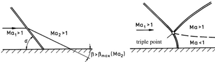
Again a line of discontinuity of entropy is formed downstream from the triple point. The static pressure has the same value on both sides of the line, but all other flow quantities attain different values.
