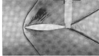
An analogy between the supersonic flow of gases and the supercritical flow of water can therefore be inferred by such an observation alone. This analogy also exists for subsonic gas flows, as an exact analysis of [Preiswerk 1938] shows.
