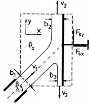
*Discontinuous Widening of a Pipe*
