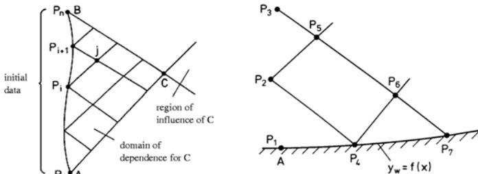
It is therefore necessary to prescribe boundary conditions for the computation of the other parts of the flow field. Two kinds of boundary conditions, representing streamlines of the flow field, are to be distinguished: the rigid wall and the free boundary, for example the edge of a
