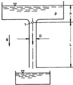
$$\begin{aligned} \tau = 10 \text{ cm}^3 \quad \rho = 900 \frac{\text{kg}}{\text{m}^3} \quad L = 0.1 \text{ m} \\ h = 0.05 \text{ m} \quad D = 1 \text{ mm} \quad T = 254 \text{ s} \\ g = 10 \frac{\text{m}}{\text{s}^2} \end{aligned}$$
