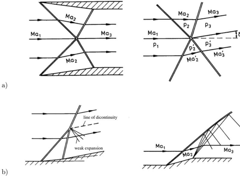
If two oblique shocks are generated by two wedges, one downstream from the other (see sketch b), they coalesce and form a single shock, which approximately produces the same rise of the static pressure as the two other oblique shocks. A mutual pass through of the shocks is not possible, and a weak expansion or compression can arise downstream from the point of intersection to balance the static pressure.
