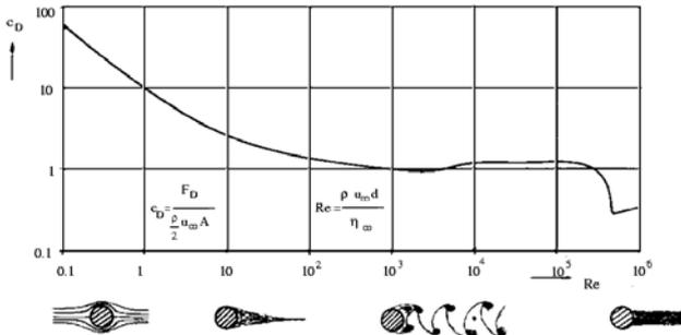
For Reynolds numbers  $200 < Re < 10^5$  (subcritical region) the drag coefficient is approximately constant and the drag is proportional to the square of the free-stream velocity. The boundary layer on the cylinder is laminar and separates at an angle of about 83 degrees, measured from the stagnation point. Downstream from the separation points the flow in the wake rolls up into
