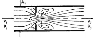
$$\zeta_o = \frac{\Delta p_l}{\frac{\rho}{2} v_1^2} = \left( \frac{1 - \psi m}{\psi m} \right)^2 \quad (1.77)$$
