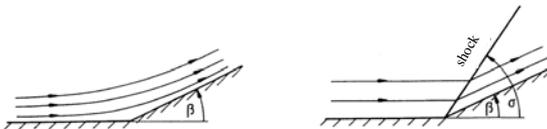
If the turning angle does not exceed a certain angle and if the Mach number in front of the shock is sufficiently large, in two-dimensional flow the shock is straight.
