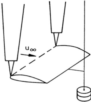
The model is suspended with two swords, fastened at the wing tips and with a wire downstream from the wing, schematically depicted in the sketch. In order to keep the interference between the model and the suspension small, the drag of the swords should be as small as possible. This requirement implies, that the size of the wing should be sufficiently large, so as to guarantee an accurate measurement of the drag.
