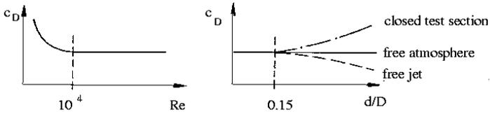
For the range of Reynolds numbers for which  $c_D = \text{const.}$ , one obtains the sketched behavior of wind-tunnel measurements compared to measurements in the atmosphere ( $d = \text{diameter of the circular disk, and } D \text{ is the diameter of the air stream in the wind tunnel}$ ). As long as the ratio  $d/D$  is small (here  $d/D < 0.15$ ), the wind tunnel measurements of the drag coefficient  $c_D$  agree with the values measured in the atmosphere.
