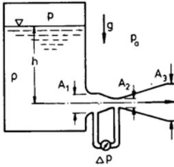
$$A = 0.3 \text{ m}^2 \quad A_2 = 0.1 \text{ m}^2 \quad A_3 = 0.2 \text{ m}^2$$
