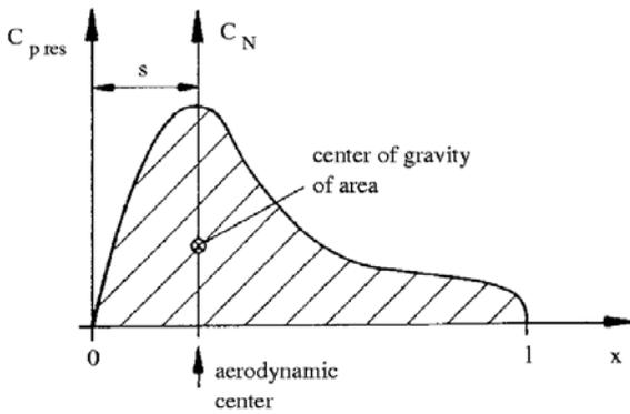
The center of gravity of the shaded area is the location of the aerodynamic center of the profile, i. e. of that point, at which the resulting force acts. The product of the distance of the aerodynamic center from the leading edge of the profile  $s$  and the normal force  $N$  is the pitching moment  $M$  about the leading edge of the profile.
