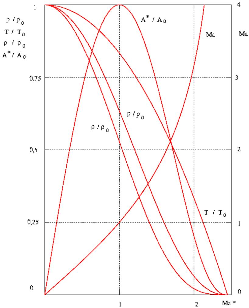
Gasdynamic quantities of the Laval-nozzle flow ( $\gamma = 1.4$ )
