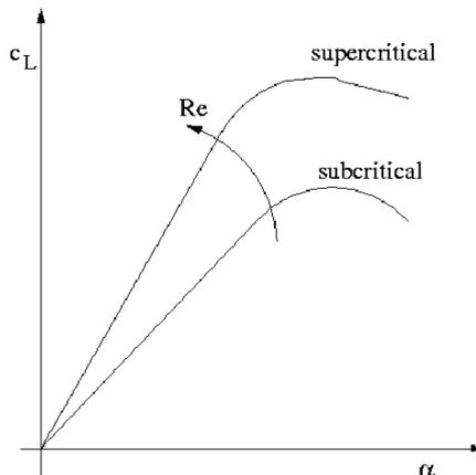
For low Reynolds numbers laminar separation is observed first and leading edge stall may result. The maximum lift coefficient is very low. With increasing Reynolds number transition is possible, and the flow can reattach. The maximum lift therefore increases with increasing Reynolds number.
