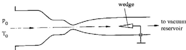
A supersonic flow with a Mach number of  $Ma \approx 2.0$  in the test section is generated by expansion of the air in the Laval nozzle.
