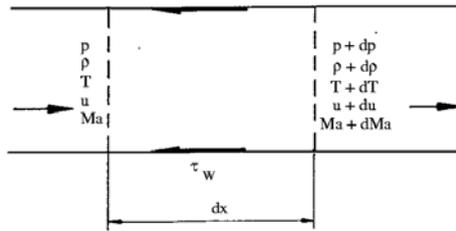
The stagnation conditions  $(T_0, p_0)$  of a flowing gas are defined by the assumption, that they are generated by an isentropic deceleration to zero velocity  $u = 0$ . The following relations are then valid:
