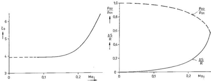
Resistance coefficient  $\zeta_B$ , increase of entropy, and loss of stagnation pressure of a standard orifice with  $m = 0.5$  as a function of the free-stream Mach number  $Ma_1$
