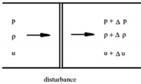
The compression of a gas by an explosion does not take place without losses, and the speed of propagation is larger than the speed of sound. Consider a small disturbance moving with the velocity  $u$  through a gas at rest. For an observer moving with the flow, the flow process is steady. The mass and momentum balance
