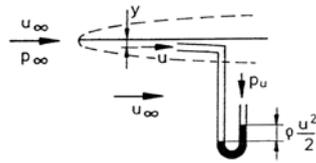
The Pitot tube is held by a support, its distance  $y$  from the surface of the plate is varied with a screwed spindle and read on a scale. The diameter of the Pitot tube must be considerably smaller than the thickness of the boundary layer, in order not to falsify the measurements. The dimension sizes of the Pitot tube are given in the sketch in mm.
