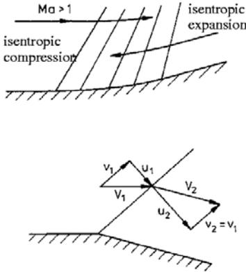
In a supersonic flow a continuously curved contour therefore generates an isentropic compression, if the turning angle is increased, and an expansion, if the turning angle is decreased.
