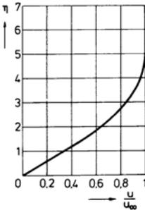
Equations (2.204) and (2.205) represent a two-point boundary-value problem, with boundary conditions to be specified at the wall and at the outer edge of the boundary layer. Because of the nonlinearity of the momentum equation, the solution is obtained by numerical integration. The profile of the tangential velocity component is shown in the following diagram.
