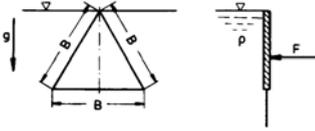
$$B = 1 \text{ m} \quad \rho = 10^3 \frac{\text{kg}}{\text{m}^3} \quad g = 10 \frac{\text{m}}{\text{s}^2}$$
