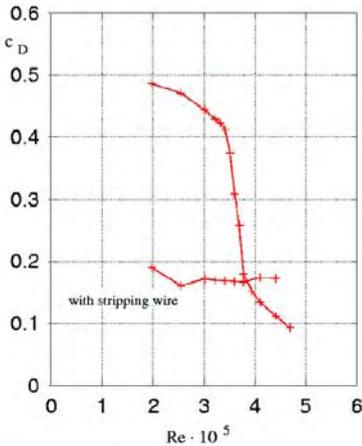
If measurements of different wind tunnels are compared, the test conditions have to be considered. For example, the intensity of the free stream, which depends on the wind tunnel used, can markedly influence the result. In earlier investigations this effect was not taken into account, as the intensity of turbulence was not known yet.
