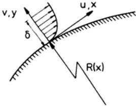
In the following only incompressible boundary layers are considered. The boundary-layer equations as listed above are also valid for flows with curved walls, if  $x$  is taken as the coordinate in the tangential direction and  $y$  in the direction of the outward normal. The boundary-layer approximation remains valid as long as
