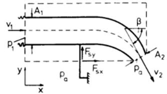
The velocities in the inlet and outlet cross section are determined with Bernoulli's equation and the continuity equation:
