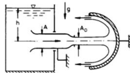
$$A = 0.2 \text{ m}^2 \quad A_D = 0.1 \text{ m}^2 \quad h = 5 \text{ m}$$
