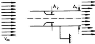
$$A_1 = 0.2 \text{ m}^2 \quad A_2 = 0.1 \text{ m}^2 \quad v_\infty = 40 \frac{\text{m}}{\text{s}}$$
