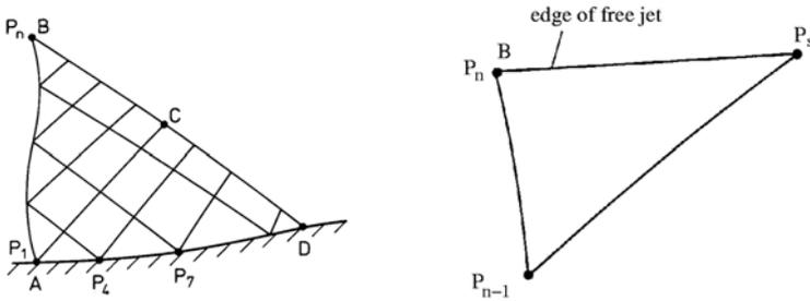
The location of the point  $P_s$  is determined by letting the streamline through the point  $B$  intersect the Mach line through the point  $P_{n-1}$ .
