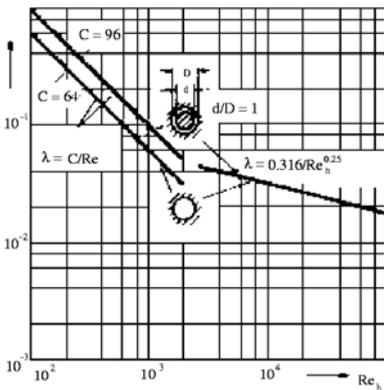
Friction coefficient for laminar and turbulent pipe flow with non-circular cross section
