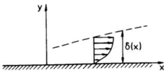
In the boundary layer the coordinate normal to the wall  $y$  is  $y = O(\delta)$  and hence  $\bar{y} = O\left(\frac{\delta}{L}\right) = O\left(\frac{1}{\sqrt{Re_L}}\right)$ . It follows from the continuity equation, that
