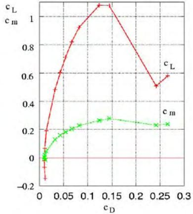
Evaluation of a three-components measurement  $L_{tot.}, D_{tot.}, M_y$  for a rectangular wing, profile NACA 23012
