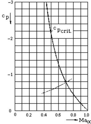
$$\begin{aligned} c_L &= \frac{1}{t} \int_0^t (c_{pl} - c_{pu}) dx \\ &\Rightarrow c_{Lc} \sqrt{1 - Ma_{\infty c}^2} \\ &= c_{La} \sqrt{1 - Ma_{\infty a}^2} \\ \Rightarrow c_{Lc} &= 0.2246; \quad c_{Lin.} = 0.214 \end{aligned}$$
