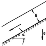
$$\delta = 3 \cdot 10^{-3} \text{ m} \quad B = 1 \text{ m} \quad \alpha = 30^\circ$$
