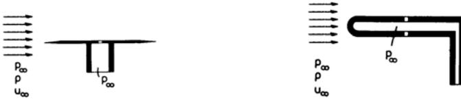
*Measurement of the Dynamic Pressure (Prandtl's Static Pressure Tube)*
