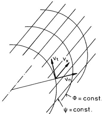
Since the streamlines  $\psi = \text{const.}$  are normal to the equi-potential lines, it follows that  $v_t = 0$ . The boundary conditions therefore are:  $v_n = 0$  for the closed test section, and  $v_x = v_t = 0$  for the open test section.
