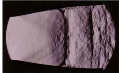
Supersonic flow with compression shock in a Laval nozzle. Mach lines can be noted upstream of the shock, which are originated on the wall of the nozzle.
