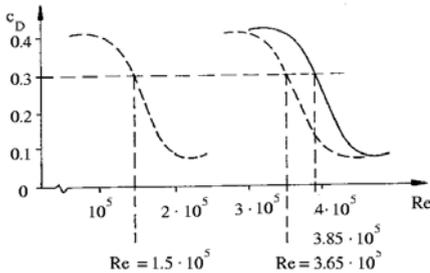
$Re_{crit.} = 1.5 \cdot 10^5$  windtunnel of poor quality (high turbulence intensity)
