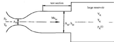
During the test the temperature in the container is  $T_v = 280 \text{ K} = \text{const.}$  At time  $t = 0$  the pressure in the container is  $p_v(t = 0) = 0.08 \cdot 10^5 \text{ Pa}$ .
