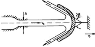
$$A = 0.1 \text{ m}^2 \quad v_0 = 60 \frac{\text{m}}{\text{s}} \quad 2\beta = 45^\circ$$
