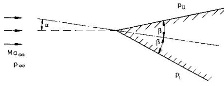
How large can the angle of attack  $\alpha$  become, without having the compression shock detach from the wedge?
