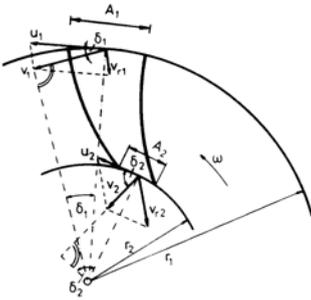
This relation is called Euler's turbine equation. The power delivered to the turbine is with the relations
