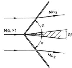
If the nose angle of the wedge  $\beta$  is  $\beta > \beta_{max}$ , the shock is detached from the wedge and deforms into a bow shock in front of the wedge.
