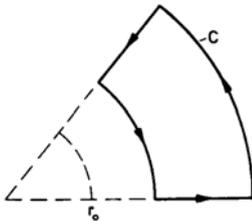
$$\begin{aligned} \Gamma &= \oint_c \mathbf{v} ds = 0 \\ \omega &= 0 \end{aligned}$$
