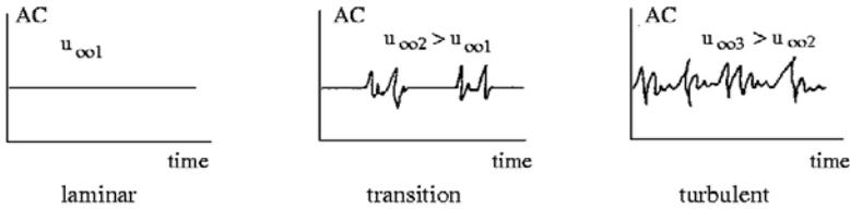
At a certain velocity  $u_\infty_{crit.}$  first fluctuations appear clearly visible (see the sketch in the middle). The critical Reynolds number is computed with this velocity.
