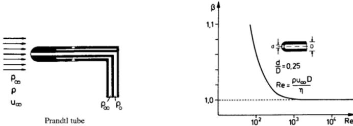
Prandtl's static pressure tube combines the static pressure probe and the Pitot probe for the measurement of the dynamic pressure, which can be determined with Bernoulli's equation from the difference of the total and the static pressure.
