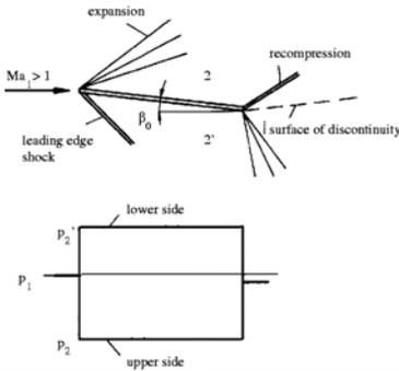
$$\begin{aligned} F_L &= (p'_2 - p_2) t \cos \beta \\ F_D &= (p'_2 - p_2) t \sin \beta \end{aligned} \quad (4.102)$$
