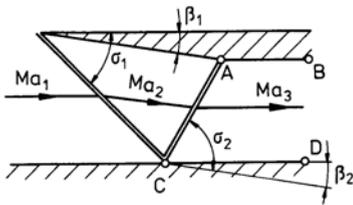
In the following sketch the reflexion of an oblique compression shock on a rigid wall is shown. If a shock impinges on a wall, it is reflected, as the wall affects the oncoming flow as a wedge.
