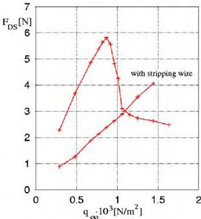
In order to obtain the drag of the sphere, the total drag of the sphere and the support must be reduced by the drag of the support (comp. Sect. 4).
