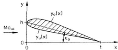
5.4 Air flows through a two-dimensional cascade. The lower side of the blades are flat, the contour of the upper side is given by the relation  $\frac{y}{t} = \frac{h}{t} \cos(\frac{\pi}{2} \frac{x}{t})$ .
