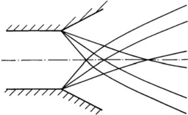
Non-simple regions also exist on the downstream side of curved compression shocks. Then the changes of the entropy have to be included in the determination of the pressure, density, temperature, and velocity. The interdependence between the distribution of entropy and the velocity field is described in the Crocco vorticity theorem.
