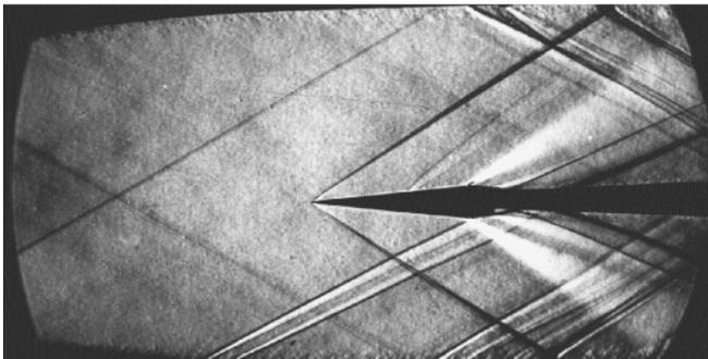
The Mach line, inclined by the angle  $\alpha$ , can be recognized in the photograph. In the actual flow it is a very weak oblique compression shock, generated by a small perturbation of the flow, caused by a piece of Scotch tape, pasted to the wall.
