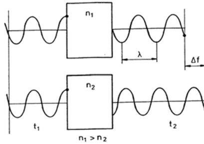
The shift  $\Delta f$  is called phase difference. If the two light rays are superposed, they cancel each other, if  $\Delta f$  is an uneven, integral multiple of one half of the wave length. If  $\Delta f$  is an integral multiple of the wave length, then they amplify each other.
