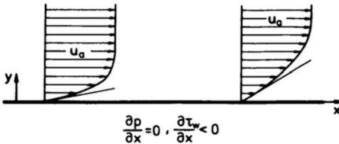
For the flat plate boundary layer, the left-hand side is zero and the velocity profile has a point of inflection at the wall. The flow in the boundary layer is retarded only by friction forces, and the change of the velocity profile in the  $x$ -direction causes a decrease of the wall shear stress.
