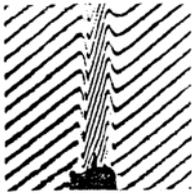
3. The picture shows a photograph of a candle light, obtained with a differential interferometer as finite fringe interferogram.
