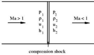
$$\begin{aligned} \rho_1 u_1 &= \rho_2 u_2 \\ p_1 + \rho_1 u_1^2 &= p_2 + \rho_2 u_2^2 \\ h_1 + \frac{u_1^2}{2} &= h_2 + \frac{u_2^2}{2} \end{aligned} \quad (4.52)$$
