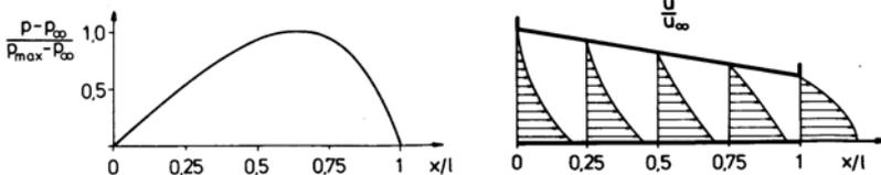
The pressure distribution and the  $x$ -component of the velocity
