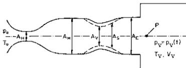
$p_0 = 10^5 \text{ Pa}; \quad T_0 = T_v = 280 \text{ K};$
