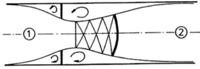
If then  $p_2/p_{01}$  is further increased,  $\zeta_O$  increases rapidly, and downstream from the orifice the flow expands to supersonic speed, subsequently being decelerated again to subsonic speed by a compression shock. The narrowest cross section of the stream, where  $Ma_e = 1$ , is enlarged. As a consequence the mass flow is increased, and  $Ma_1$  exceeds  $Ma_{1crit.}$ .
