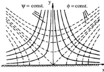
$$\Phi = a(x^2 - y^2) \quad \Psi = 2ax y \quad , \quad (2.125)$$
