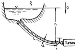
$$h = 200 \text{ m} \quad L = 300 \text{ m} \quad A = 0.2 \text{ m}^2$$
