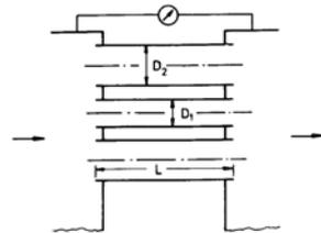
$$\begin{aligned} D_1 = 0.025 \text{ m} \quad D_2 = 0.064 \text{ m} \\ L = 10 \text{ m} \quad \rho = 10^3 \frac{\text{kg}}{\text{m}^3} \quad \lambda = 0.025 \\ \Delta p = 10^5 \frac{\text{N}}{\text{m}^2} \quad \zeta = 1 \end{aligned}$$
