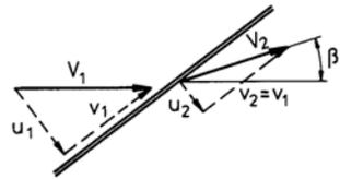
$$\frac{s_2 - s_1}{R} = \ln \left\{ \left[ 1 + 2 \frac{\gamma}{\gamma + 1} (Ma_1^2 \sin^2 \sigma - 1) \right]^{\frac{1}{\gamma - 1}} \left[ \frac{(\gamma + 1) Ma_1^2 \sin^2 \sigma}{(\gamma - 1) Ma_1^2 \sin^2 \sigma + 2} \right]^{-\frac{\gamma}{\gamma - 1}} \right\}, \quad (4.74)$$
