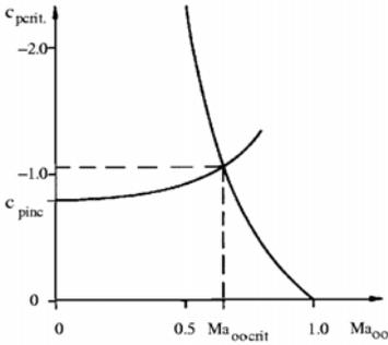
The application of the Göthert rule will be shown as the third example. According to this rule the product of the thickness ratio  $\frac{d}{t}$  and  $(1 - Ma_\infty^2)^{\frac{1}{2}}$  remains constant. If the pressure distribution of a wing, known for a given angle of attack in incompressible flow, is to be converted to a compressible subsonic flow, the chord of the wing  $t$  is changed for constant maximum thickness to
