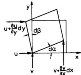
Generalization of the last equation to three space coordinates leads to the vector of rotation or vorticity
