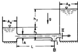
$$h_1 = h_2 = 5 \text{ m} \quad L = 10 \text{ m} \gg D$$
