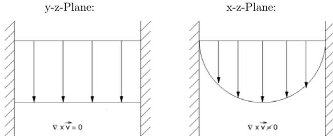
It can be shown, that the velocity components, averaged over the gap between the plates can be derived from a potential, and it can be concluded that the flow of a viscous fluid is analogous to an irrotational flow with regards to the velocity components averaged over the gap between the two plates.
