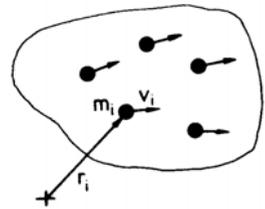
Similar to the derivation of the momentum theorem the transition from the particle system to the continuum is achieved by substituting the sum on the left-hand side of (1.99) by a volume integral
