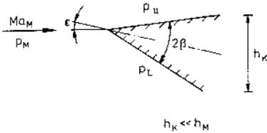
How large can the angle of attack  $\epsilon$ , be, without detachment of the compression shock? How large are the pressure difference  $p_l - p_u$ , and the Mach numbers  $Ma_u$  and  $Ma_l$  for this case?
