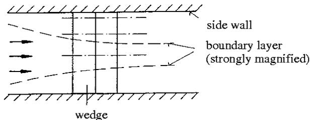
The sketch shown above depicts the top view of the wedge in the test section of the wind tunnel. The model extends to both side walls of the tunnel. As indicated in the sketch by the dashed curved lines a turbulent boundary layer develops on the side walls. The thickness of the boundary layer is strongly magnified. Also indicated in the sketch are 3 sections, one in the middle of the tunnel (section 1), one closer to the side wall (section 2), and the third near the wall (section 3).
