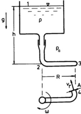
In order to be able to determine the out-flow velocity  $v_r$ , the flow between the fluid surface in the reservoir and the exit cross section is assumed to be loss-free. The energy equation for the system considered is
