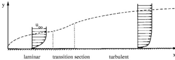
The transition from laminar to turbulent flow is influenced by disturbances in the inviscid flow and in the boundary layer, by the pressure gradient, the curvature and the roughness of the wall, the wall temperature, and density changes in compressible flow.
