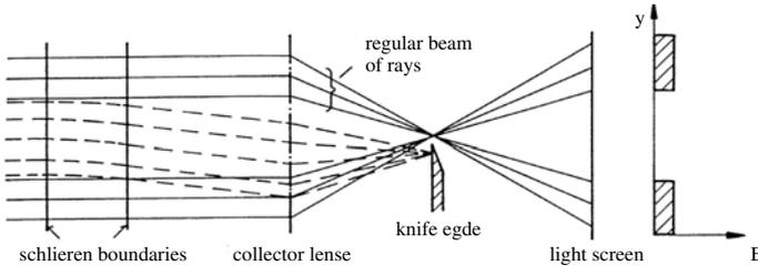
Because of the finite size of the focal spot, about half of it is covered with the knife edge, so that the optical system is sufficiently sensitive. The schlieren then appear in different grey tints, depending on their direction and intensity, which is approximately given by
