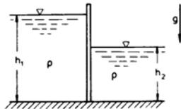
$$B = 10 \text{ m} \quad h_1 = 5 \text{ m} \quad h_2 = 2 \text{ m}$$
