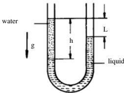
$$h = 0.3 \text{ m} \quad L = 0.2 \text{ m} \quad \rho_w = 10^3 \frac{\text{kg}}{\text{m}^3}$$
