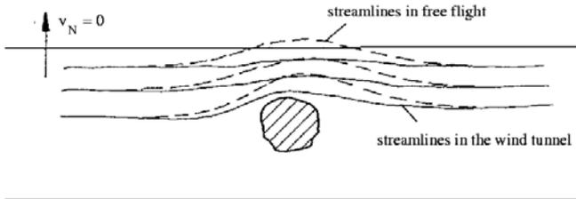
In an open test section the conditions are reversed; the flow can stronger expand in the direction normal to the oncoming flow than in the free atmosphere.
