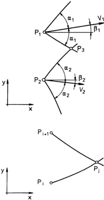
With the Prandtl-Meyer angle  $\nu_3$  known, the Mach number  $Ma_3$  and the other flow quantities can be determined. The location of the point  $p_3$  is computed with a difference-solution of the characteristic equations.
