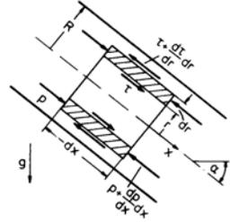
*Flow in the Intake Region of a Pipe*
