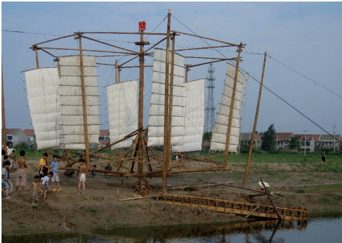
Fig. 2 The field-test of the vertical shaft type wind-power Chinese square-pallet chain-pump in Haihe in the northern Jiangsu province
