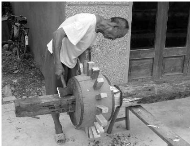
a) Assembling driven gear and transmission shaft
