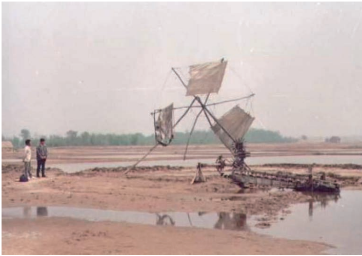
Fig. 6 A horizontal-axle windmill driving a water-lifting device [15]
