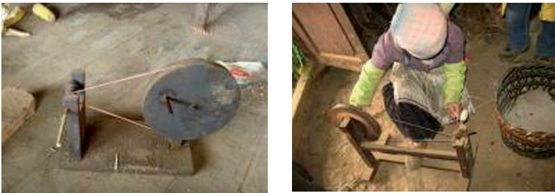
Fig. 3 (a) A woof reel (Jan. 2007) ( left ); (b) A woman winding a hemp thread on a spool with a woof reel (Jan. 2007) ( right )
