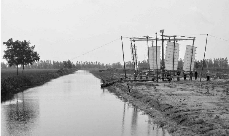
Fig. 14 The reconstructed traditional CGW and Its SPCP in a field in Sheyang County, Jiangsu Province (2006)
