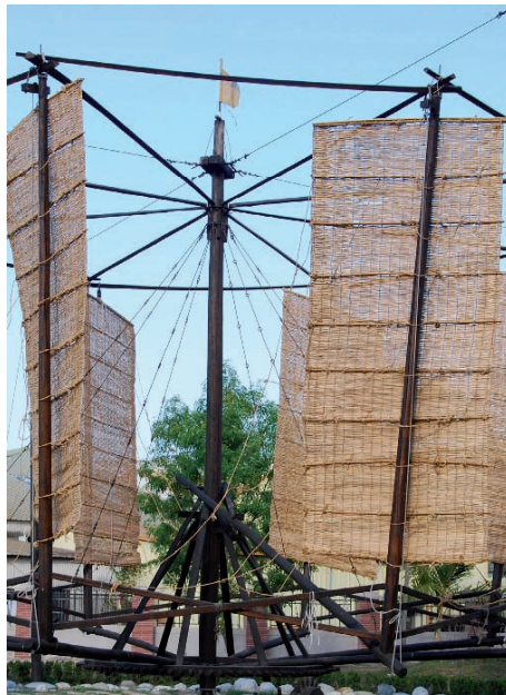
Fig. 11 (a) The position of the sails while against the wind; (b) The bulrush sails and its rig
