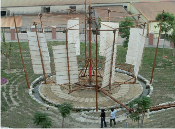
Fig. 3 The vertical shaft type wind-power Chinese square-pallet chain-pump stands on the campus of the Southern Taiwan University
