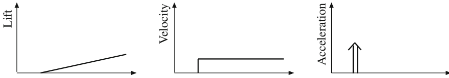
Fig. 1.2 A simple ramp. This is a poor design
