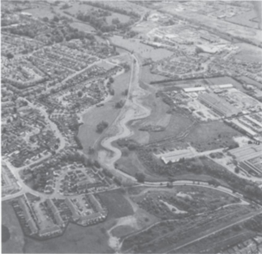
*Plate 6.4* The restored River Skerne, Darlington, UK, showing the introduced meander and rehabilitated floodplain (photo copyright AirFotos, Newcastle upon Tyne)
