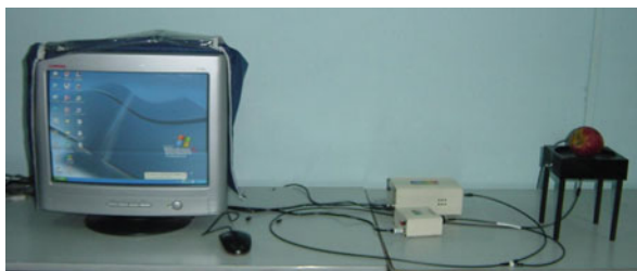
Fig. 6.29 NIR spectra acquisition set-up
