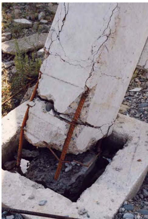
Fig. 2-4: Shear failure of precast concrete column at foundation socket (1999 Kocaeli earthquake)
