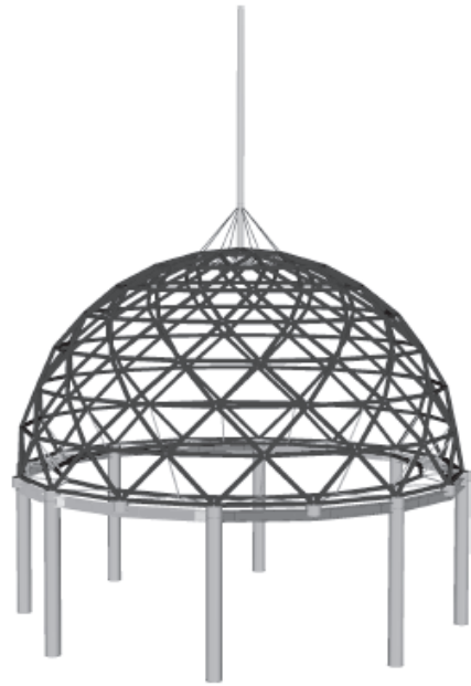
FIGURE 7.3 The single-layered semi-spherical dome at the roof of a building.
