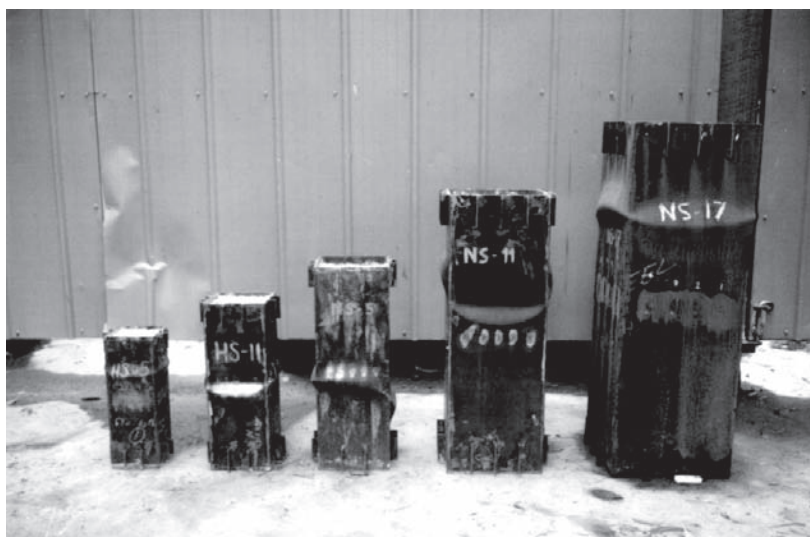
FIGURE 6.53 Local buckling of concrete-filled steel columns (Uy, 2000).
