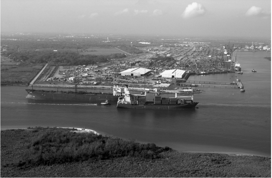
FIGURE 15-2. (Continued) "Texas Chicken" Maneuver at Barbour's Cut on the Houston Ship Channel; approach and passing sequence. (U.S. Coast Guard Digital).
