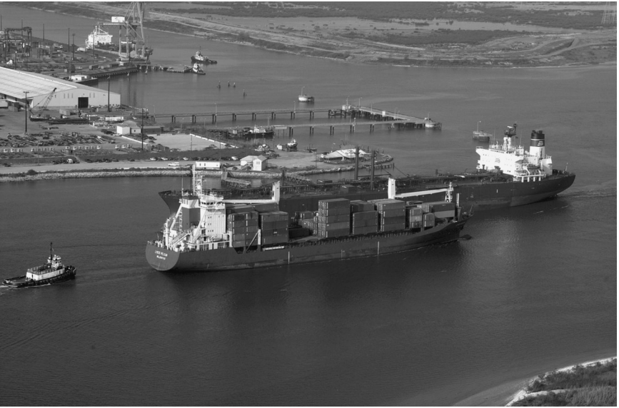
FIGURE 15-2, Top and Bottom: "Texas Chicken" Maneuver at Barbour's Cut on the Houston Ship Channel; approach and passing sequence. (U.S. Coast Guard Digital). (Continued)
