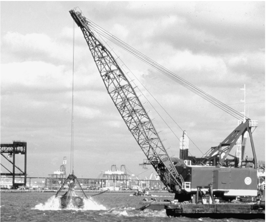
FIGURE 10-8. Clamshell Dredge (COE, Digital Visual Library).
