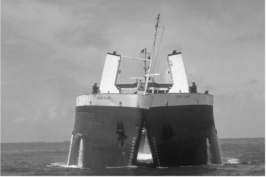
FIGURE 10-2. Hopper Dredge Splits Its Hull in Gulf of Mexico near Galveston, Texas (COE, Digital Visual Library).
