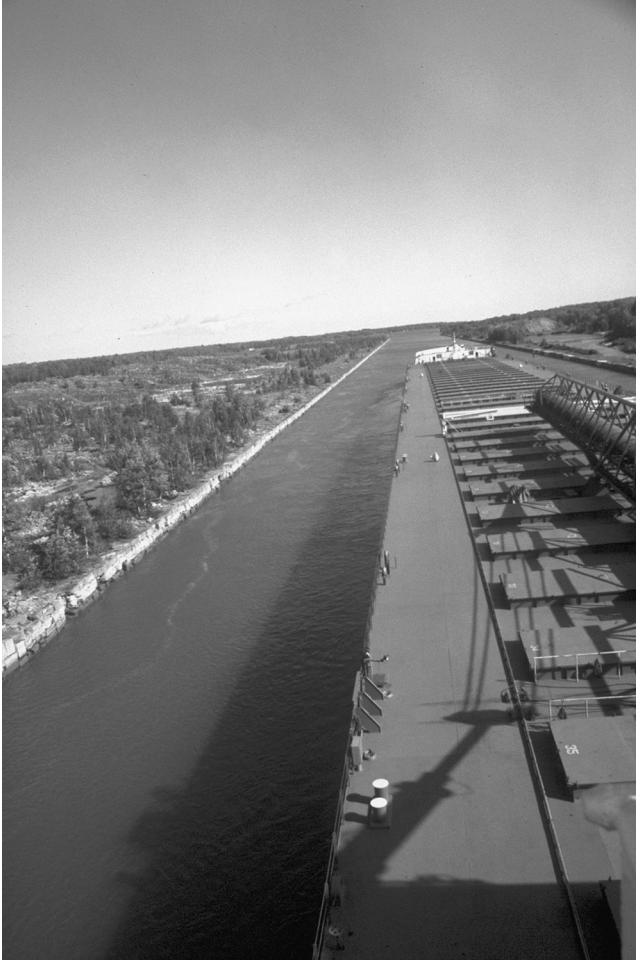
FIGURE 8-3. 1,000-Foot Laker in the Rock-Cut Portion of the St. Mary's River, Michigan (COE-Digital Visual Library).
