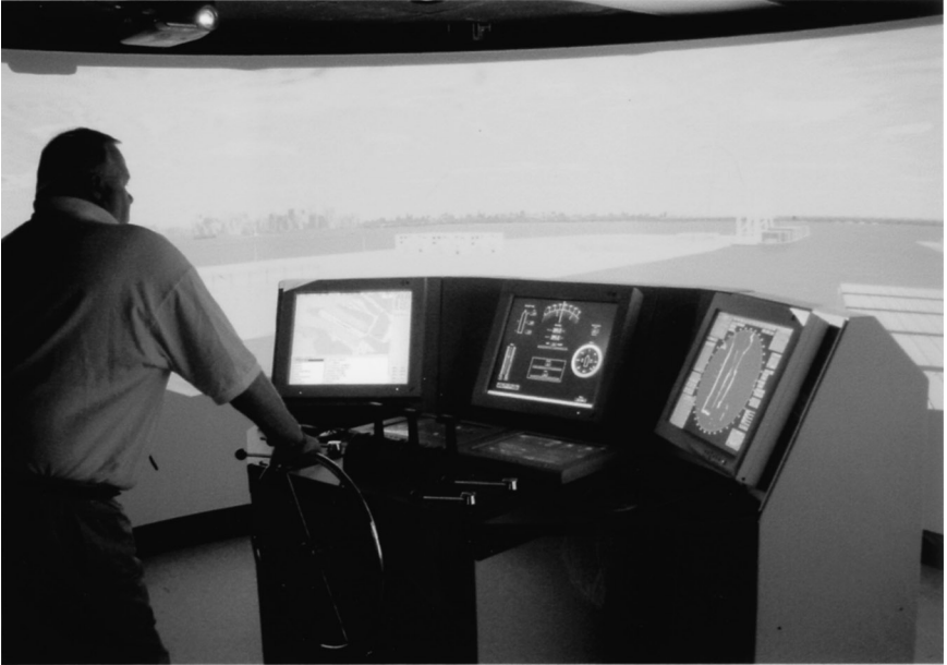
FIGURE 15-1. Vessel Simulator (COE Waterway Experiment Station).
