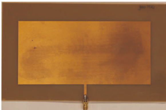
Fig. 4.58 Microstrip patch antenna with microstrip line feed matched to 50\ \Omega
