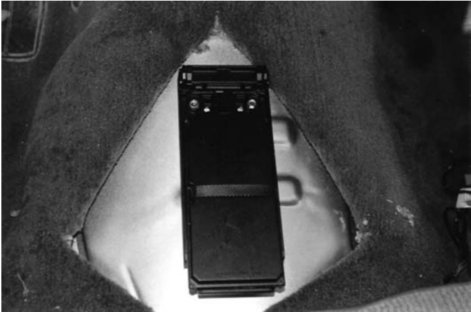
Figure 13.7 Accelerometer in test vehicle.
