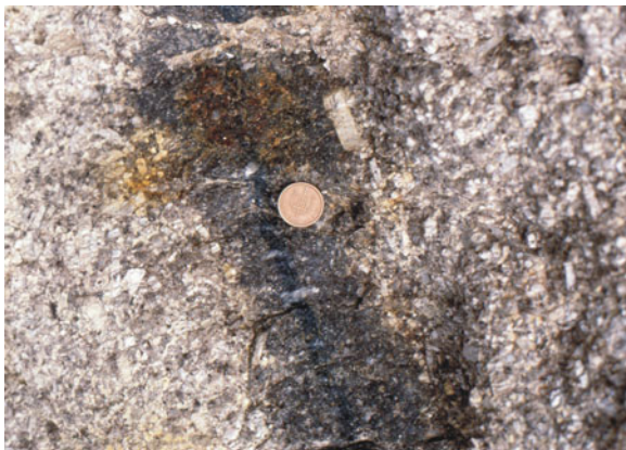
Fig. 2.8 Example of a greisen vein cutting granite (subsequently kaolinised), Cligga Head, Cornwall, UK. A central tourmaline vein is flanked by greisen in which feldspars are largely replaced by muscovite and quartz
