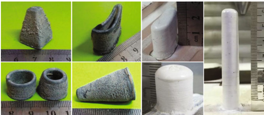
Fig. 5.2 Ceramic structures fabricated by laser engineered net shaping
