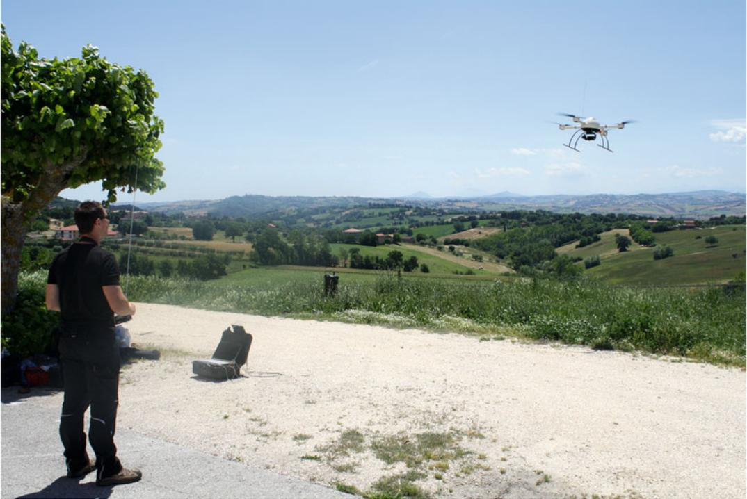
**Fig. 4.9** Experiments with a quadcopter during aerial photography survey over the site of *Trea* (June 2013) (Photo by the author)
