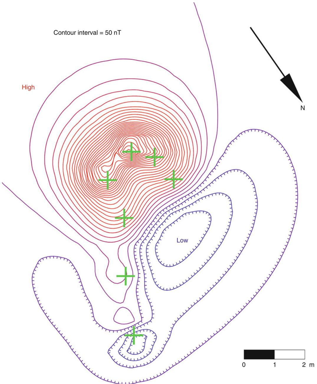
**Fig. 7.14** The calculated magnetic field of a modeling program approximates the measurements that were made on the underground kiln in Fig. 7.10
