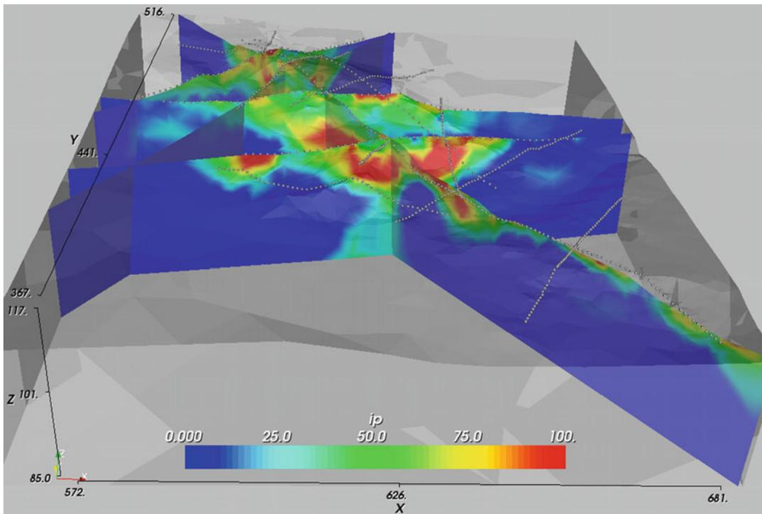
**Fig. 10.7** Three-dimensional presentation of ERT data: IP effect measured on a slag mound in Ain Al-Hajar, Morocco (Ullrich et al. 2007b)
