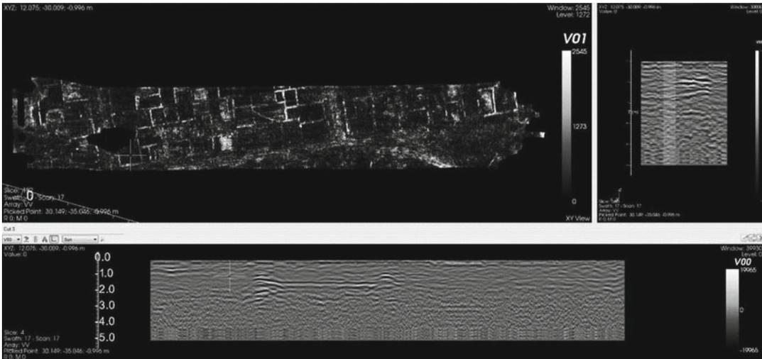
**Fig. 9.9** Interactive view of depth slice at 0.996 m depth (*top left*), perpendicular section (*top right*) and longitudinal section (*bottom*). The area is approximately 1 ha and was collected in 2 h at 6 cm × 12 cm resolution
