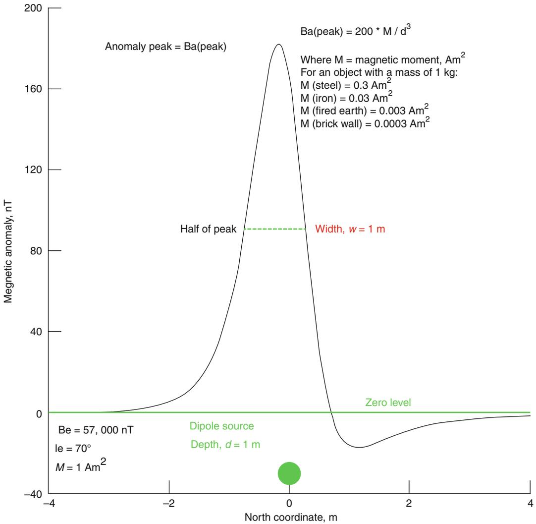
**Fig. 7.13** The half-width rule approximates the depths of objects and estimates of mass are also possible
