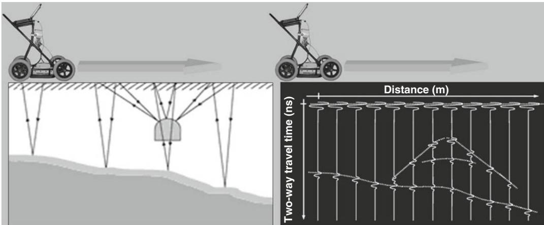
**Fig. 9.1** The GPR cart is moved along a certain distance in order to equidistantly acquire reflected energy traces
