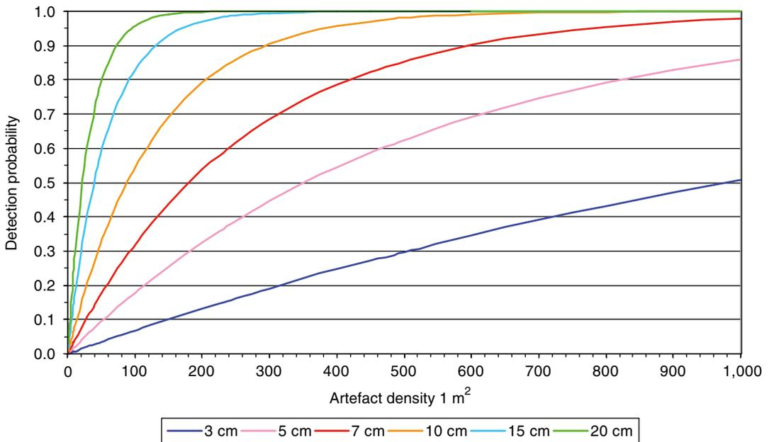
**Fig. 12.10** Detection probabilities for different core diameters (Source: Tol et al. 2004, reproduced with permission)
