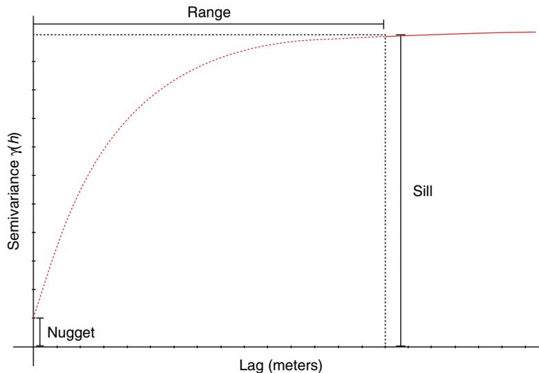
**Fig. 13.8** Representation of a theoretical variogram
