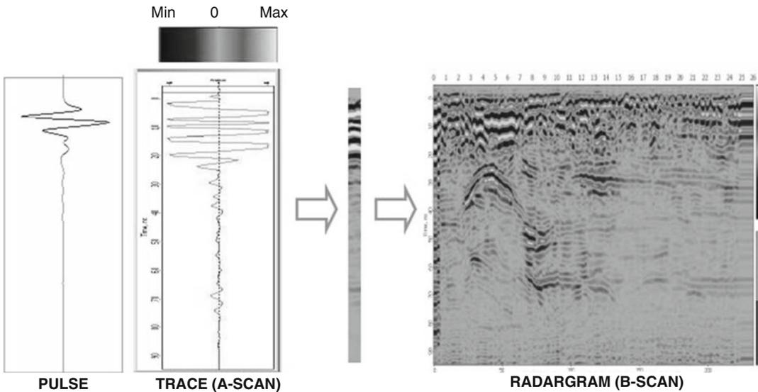
**Fig. 9.4** From left to right: *Pulse* transmitted by the transmitter. *Trace (A-scan)* recorded by the receiver. *Radargram (B-scan)* representing a sequence of A-scans equidistantly spaced along the X axis
