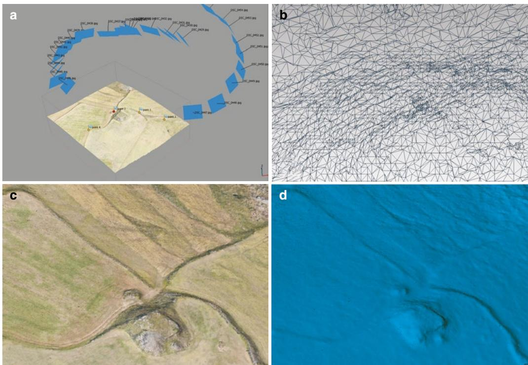
**Fig. 13.5** Different stages in the production of DEMs through photogrammetric restitution. (a) Orientation of cameras over the photo-texturized DTM. (b) Mesh
