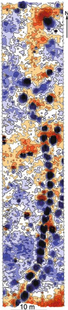
**Fig. 7.2** Bronze-Age cooking pits in Denmark form lines of circular magnetic anomalies that have amplitudes of over 20 nT
