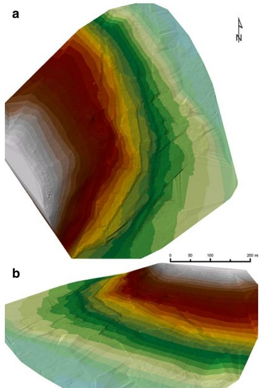
**Fig. 13.10** TIN model of the Roman Town of *Ammaia*. The faceted aspect of the model is clearly visible in the orthogonal (a) and the perspective (b) views. (Marvão, Portugal)
