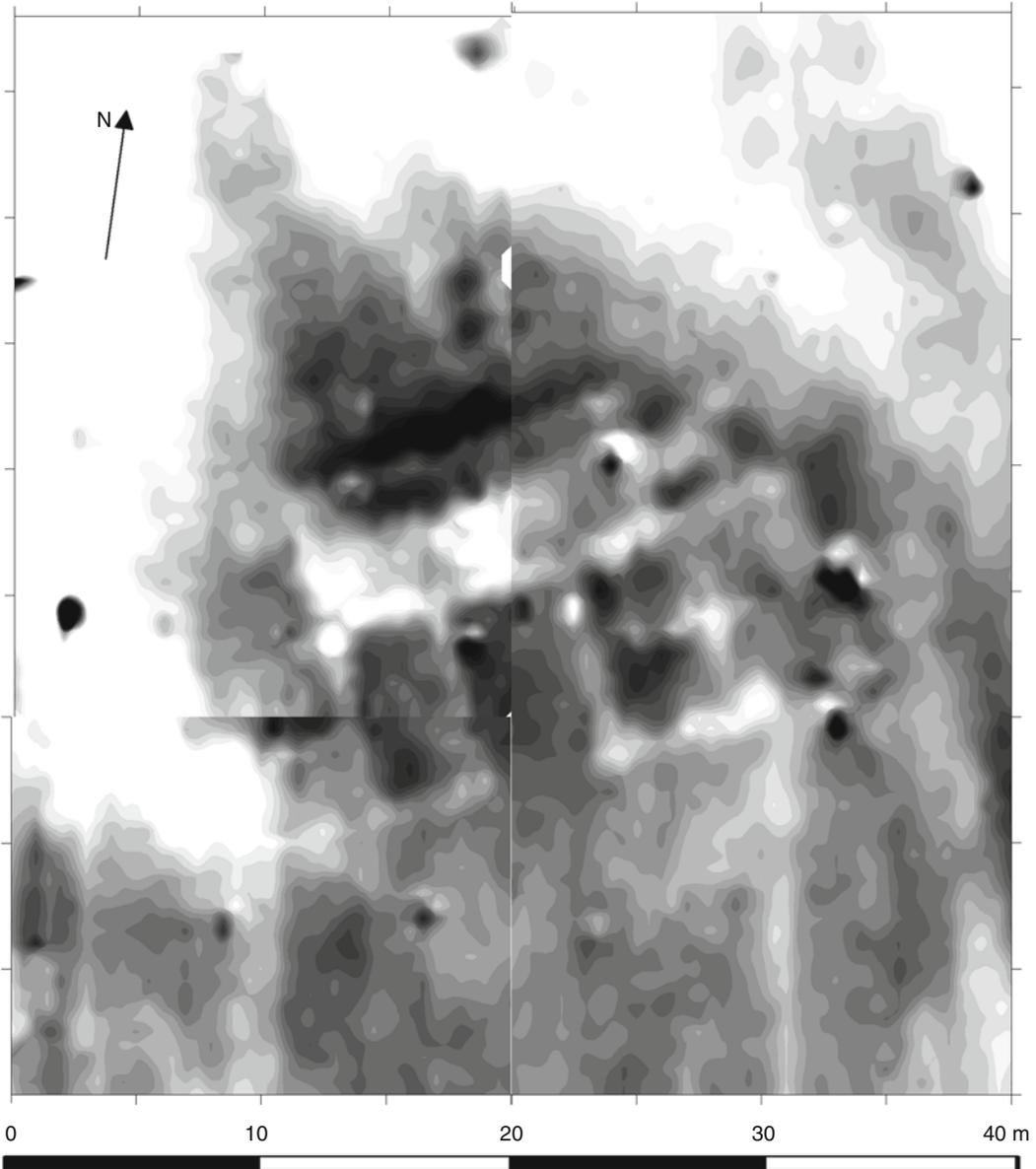
**Fig. 7.6** The limestone walls of a Roman villa in Macedonia are detected as magnetic lows with an amplitude of 5–10 nT
