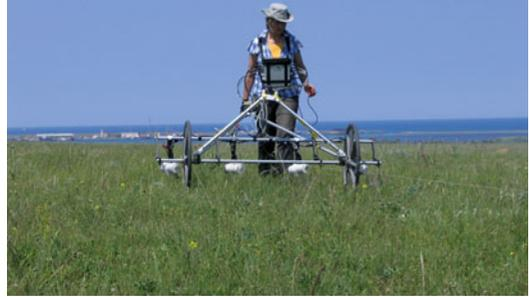
**Fig. 7.12** Four magnetic sensors (the *white cylinders*) on a cart allow an exploration of a band that is 2 m wide
