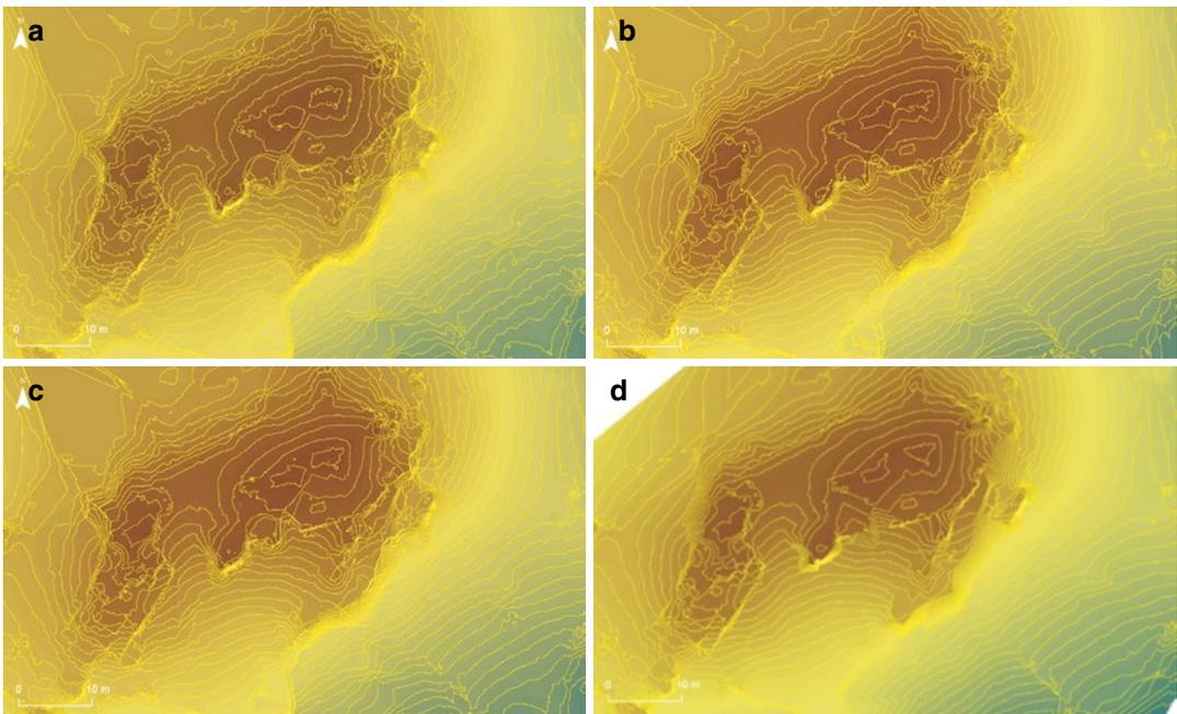
**Fig. 13.7** Visual comparison of raster DEMs obtained by IDW (a), kriging (b), splines (c) and TIN (d) of an archaeological site (Taken from Martínez del Pozo et al. 2010)
