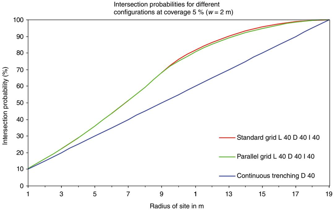
**Fig. 12.7** Effect of trench configuration on intersection probability, using the same area coverage of 5 % (Source: Verhagen and Borsboom 2009)
