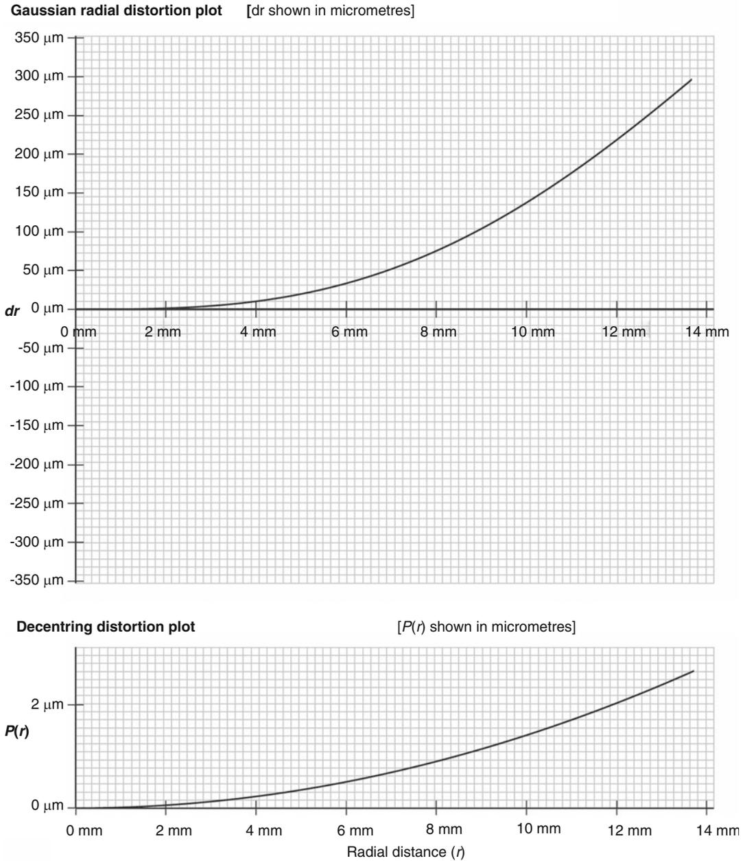
**Fig. 3.3** Radial and decentering distortion plots of the AF Nikkor 24 mm f/2.8D (infinity focus). The radial distortion  $dr$  (expressed in micrometres) and decentering distortion  $P(r)$  are given as a function of radial distance  $r$  (mm)
