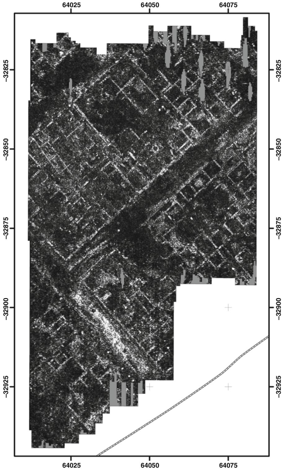
**Fig. 10.4** Amplitude slice of GPR data, *Ammaia*, Portugal (Verdonck and Taelman 2012)
