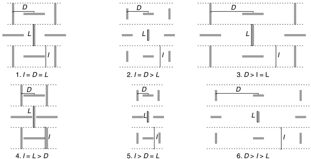
**Fig. 12.6** Manipulating trench length ( $L$ ), interval ( $I$ ) and distance ( $D$ ) can lead to a potentially endless array of systematic trenching patterns (Source: Verhagen and Borsboom 2009)
