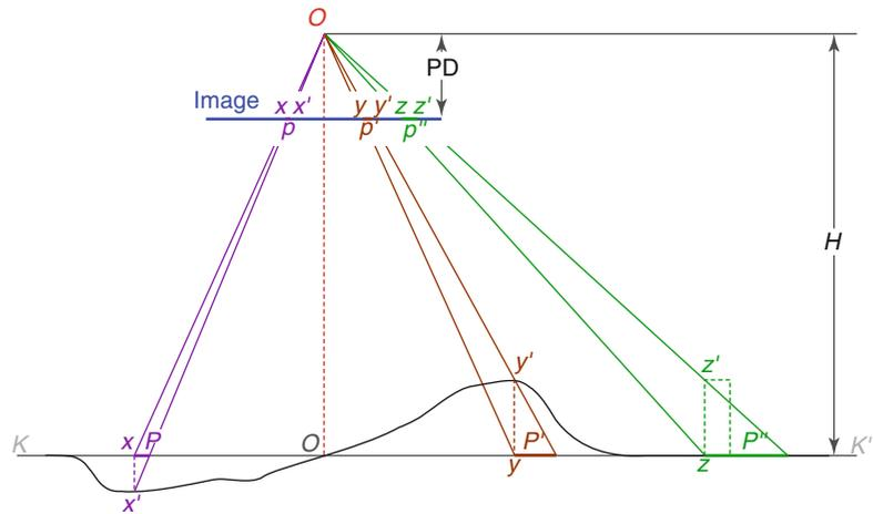
(because its projection is a perfect orthogonal projection), relief displacement is always radial from the nadir or plumb point  $o$ . This is determined by the intersection of a vertical, constructed from the optical centre  $O$  towards the ground, and the image plane; this vertical axis is equal to the optical axis of the whole system in the case of a perfect vertical photograph – such as Fig. 3.5 (Tewinkel et al. 1966).
