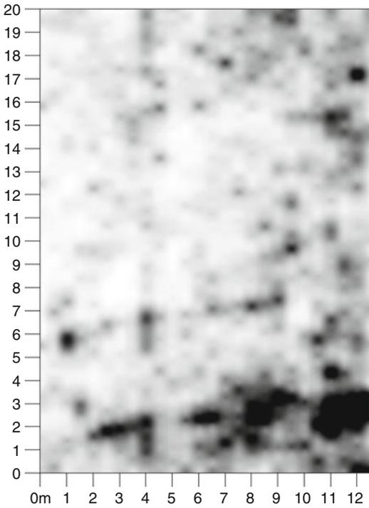
**Fig. 9.7** Horizontal depth slice at 52 cm depth generated from a standard pseudo 3D surveying and processing. Some linear targets (*black colour*) are hardly visible
