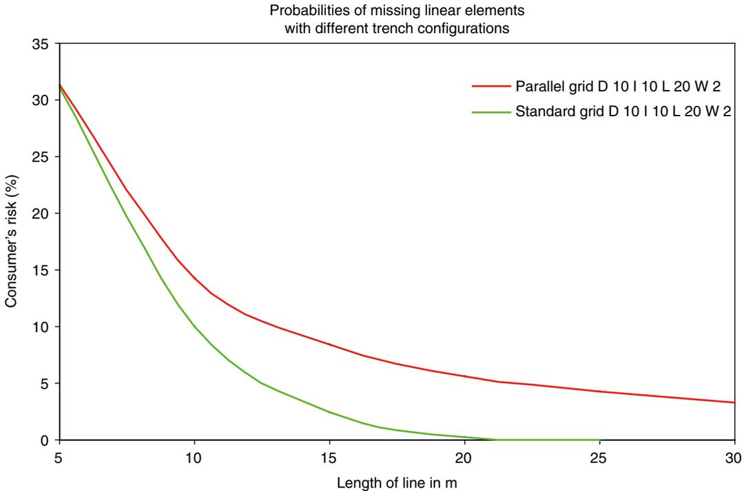
**Fig. 12.8** Probability of missing a linear element with different trench configurations, using the same area coverage (Source: Verhagen and Borsboom 2009)
