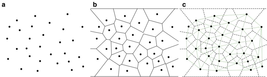
**Fig. 13.9** How a TIN model is produced
