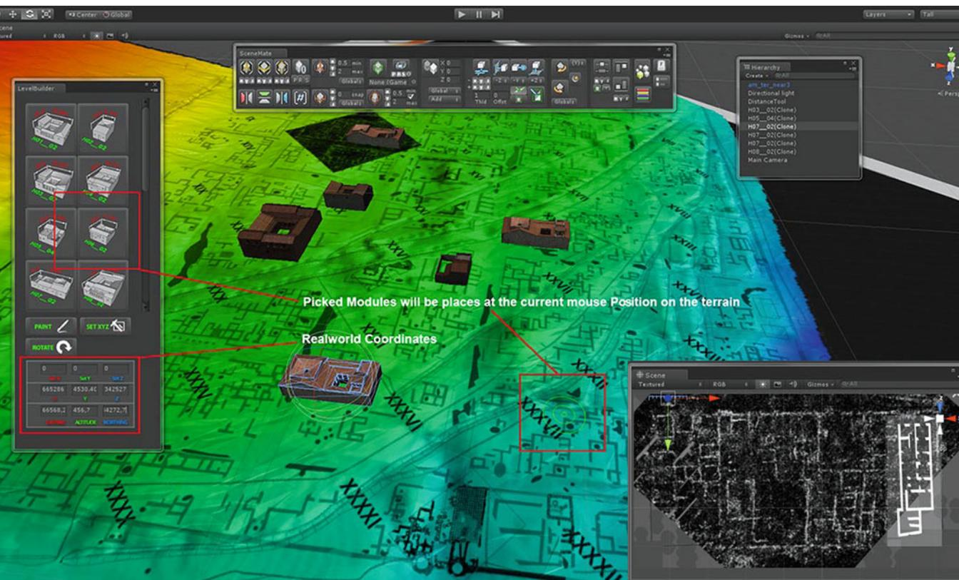
**Fig. 18.3** Real-time construction editor with the library of modularised building blocks
