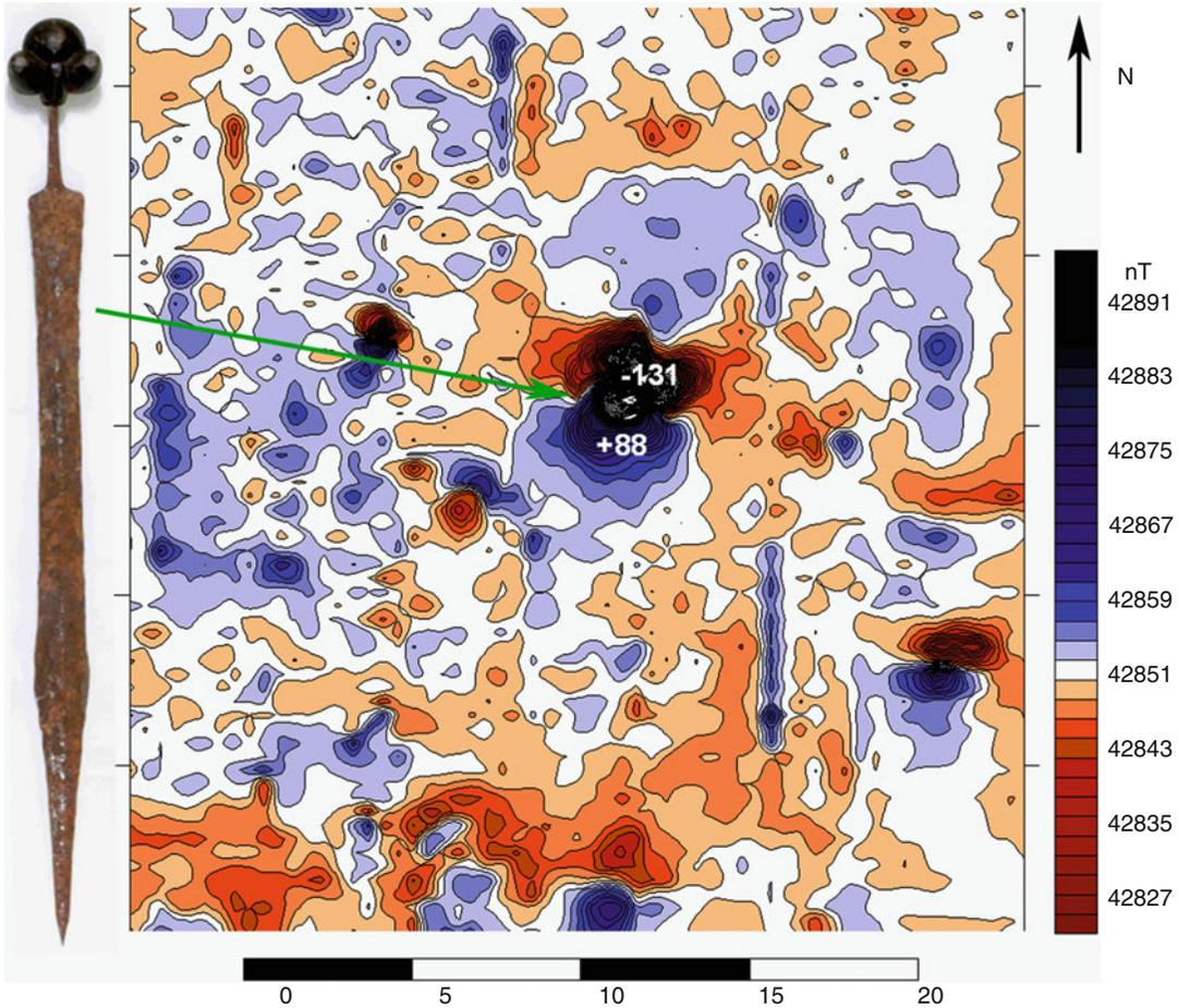
**Fig. 7.11** In the Fayoum Oasis, a dipolar magnetic anomaly with an amplitude of about 100 nT located an iron sword (shown on the *left*) that dates to about the second century AD
