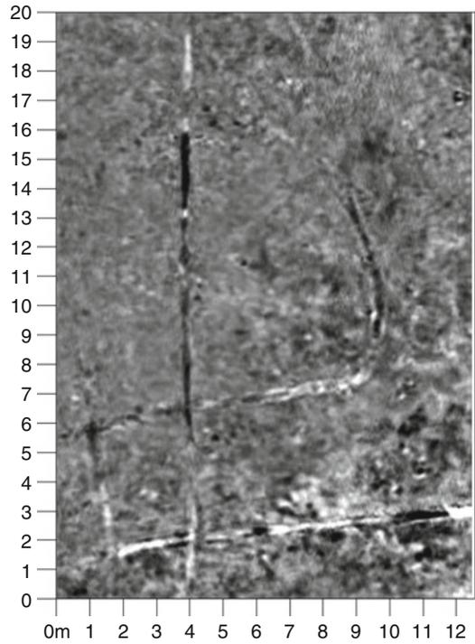
**Fig. 9.8** Horizontal depth slice at 52 cm depth generated from full-resolution data acquisition and processing. Linear anomalies represent as small objects as 5 cm diameter PVC pipes and irrigation lines
