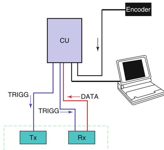
**Fig. 9.2** Basic scheme of a GPR system. *Tx* transmitter, *Rx* receiver, *CU* control unit, *TRIGG* trigger
