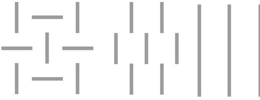
**Fig. 12.5** The three most commonly used systematic trial trenching patterns. From *left to right*: the standard grid, the parallel staggered grid and the continuous parallel trenching pattern (Source: Verhagen and Borsboom 2009)
