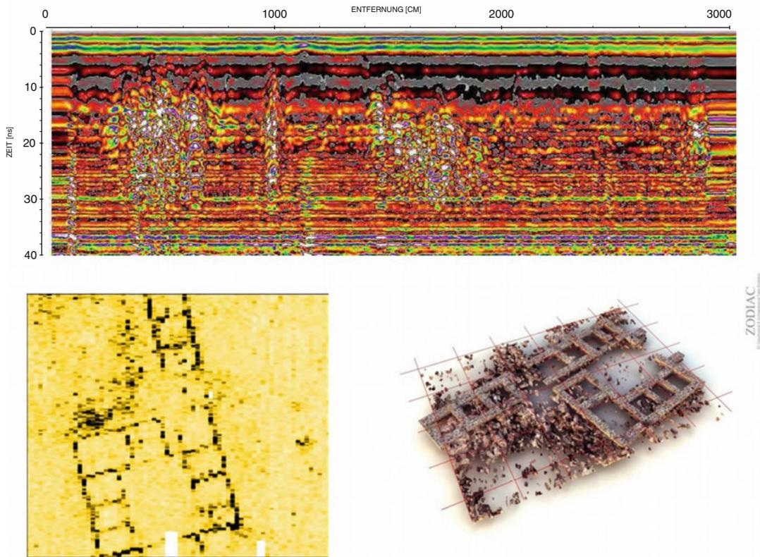
**Fig. 10.6** GPR data presentation: single 2D profile, amplitude slice and 3D reconstruction (Meyer et al. 2007)
