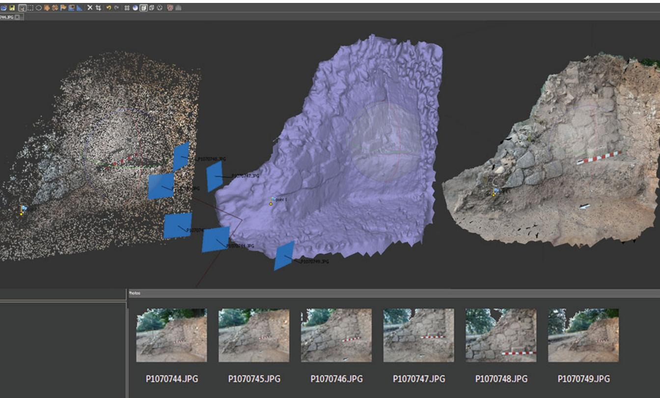
**Fig. 18.2** Production of a 3D reconstruction with Agisoft
