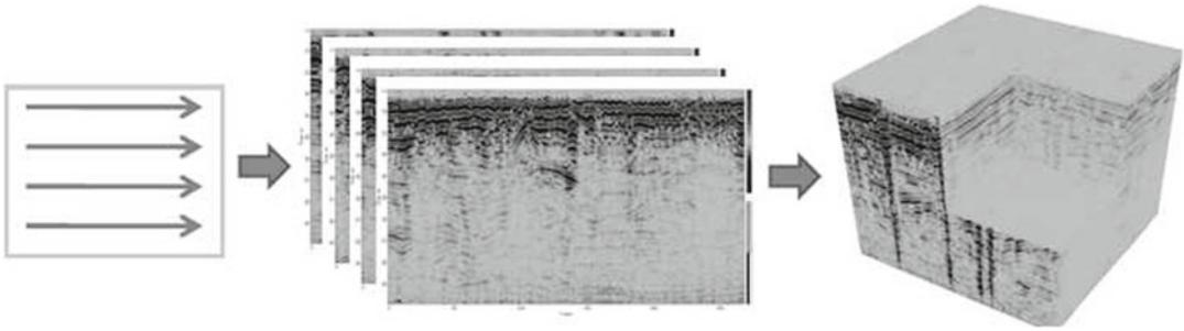
**Fig. 9.5** From *left to right*: Grid plot of data collection shows four parallel profiles. The raw data acquired are four B-scans. During post-processing the B-scans can be compiled into a 3D volume (or C-scan)
