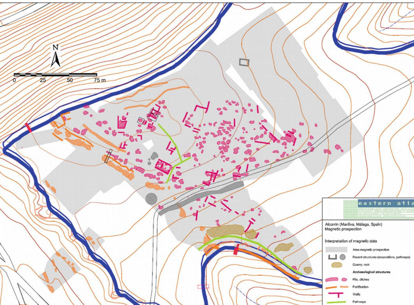
**Fig. 10.3** Topographic map and interpretation of magnetic data, Alcorrín, Spain (Marzoli et al. 2010)
