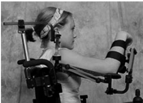
FIGURE 8.17 Wilmington Robotic Exoskeleton (WREX) mounted to a wheelchair.
