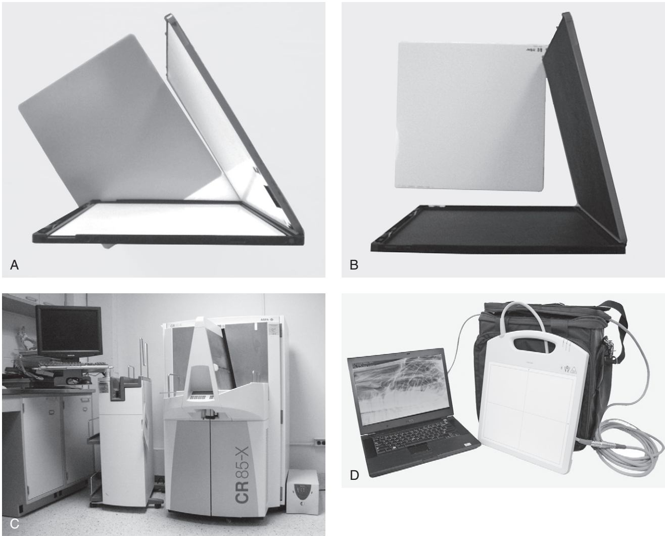
Figure 67-3. Radiographic equipment: A , 400-speed film screen equipment with green-based film. B , Computed radiography cassette and imaging plate. C , AFGA computed radiography processor. D , Sound-Eklin Mark IIG direct digital radiography system. Image plate sends the x-ray information transformed into electric signal to a computer for display. ( D , Courtesy Sound-Eklin Medical Systems, Inc.)
