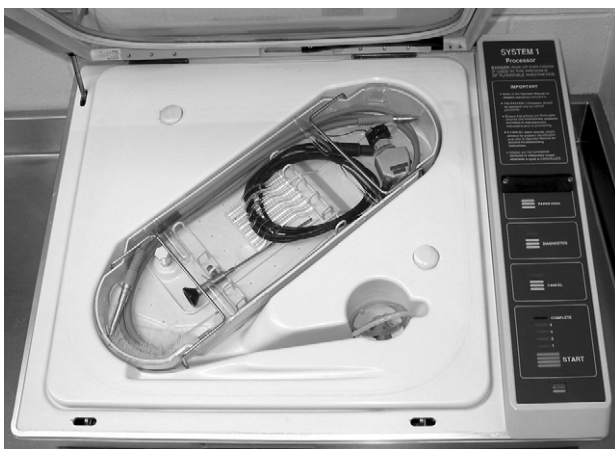
Figure 9-8. Peracetic acid sterilizer (Steris System 1), which is used to sterilize endoscopes, arthroscopes, and other equipment.
