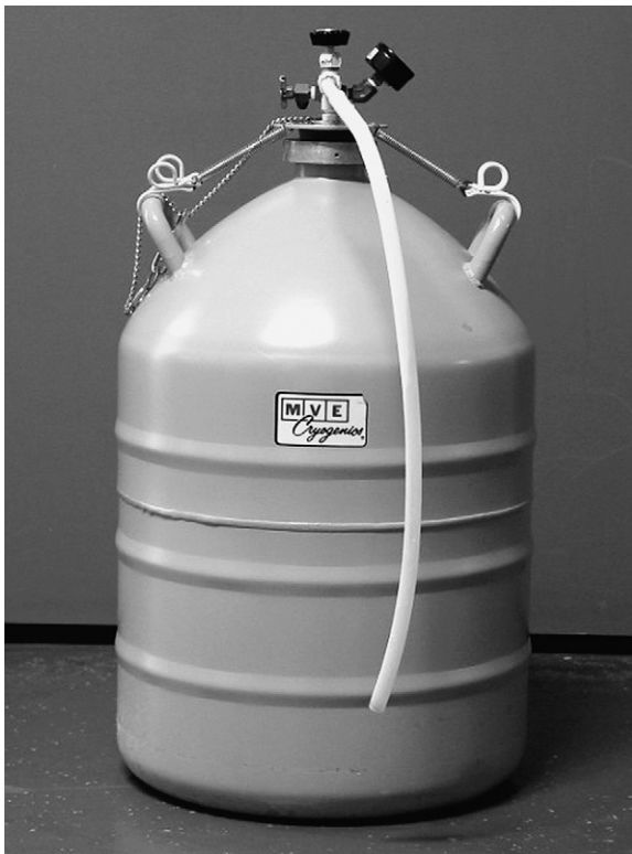
Figure 14-1. Insulated Dewar flasks are used to store liquid nitrogen. This tank is fitted with a special adaptor lid and spray gun attachment. Note the pressure gauges used to regulate the liquid nitrogen.
