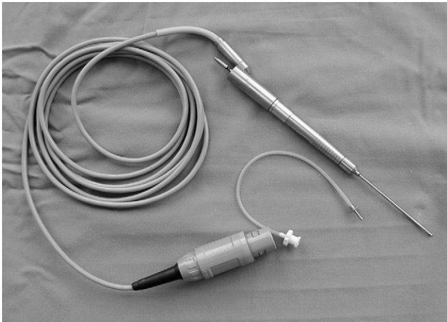
Figure 58-10. Custom-made vitrectomy handpiece with a 55-mm shaft and independent irrigation port.
