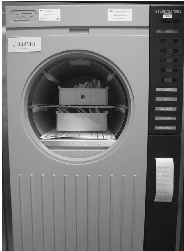
Figure 9-7. Gas plasma sterilization unit (Sterrad) that uses H_2O_2 to generate free radicals, which inactivate microbes.
