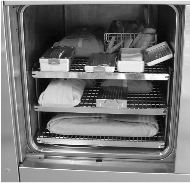
Figure 9-5. A typical sterilization unit in a large hospital, loaded and ready for use. Note that the contents are loosely arranged to facilitate access of steam around each item.
