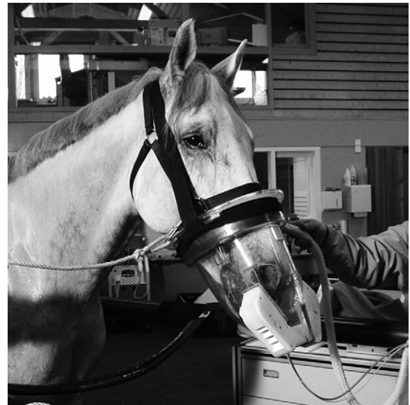
Figure 42-14. Horse with mask and ultrasonographic spirometer used to generate flow volume and flow time curves during high-speed treadmill exercise.
