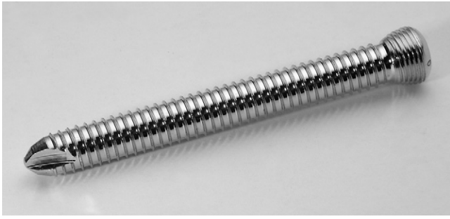
Figure 76-13. A self-tapping locking-head screw. Note the threads manufactured into the conical screw head. These interlock with complementary threads in the plate. The self-tapping ends are visible at the tip of the screw.
