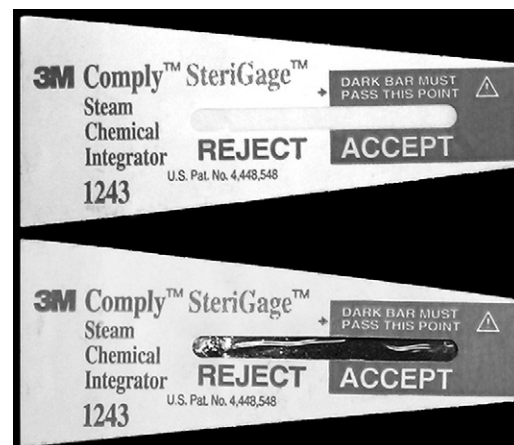
Figure 9-3. Example of a chemical indicator used to confirm that sufficient exposure conditions have been met in the center of the pack. In this 3M Comply (SteriGage) Steam Chemical Integrator, the chemical pellet contained in a paper, film, and foil laminate envelope melts and migrates as a dark color along the paper wick. The distance or extent of migration shown at the bottom (compare with unused, top) depends on exposure to steam, time, and temperature. The dark color should enter the Accept window for an Accept result.
