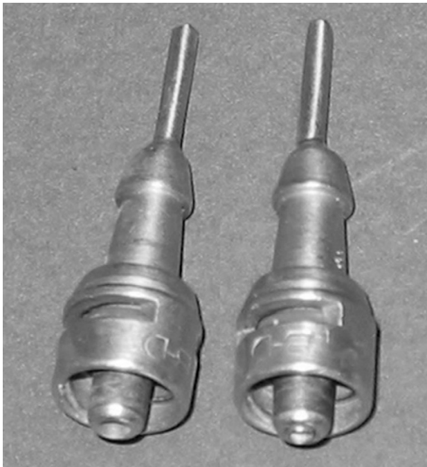
Figure 14-3. Two examples of needles that attach to the spray gun to deliver liquid nitrogen sprays directly onto the tissue to be frozen. The volume and size of the spray drop is determined by the diameter of the needle orifice.
