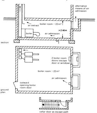
(3) Boiler room with 2 doors (min. 22 m<sup>3</sup>) needed for heat output > 350 kW
