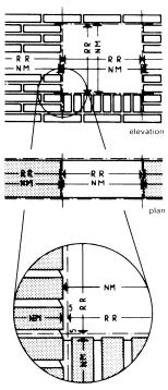
Standard dimensions for basic construction (RR) and nominal dimensions (NM) for brickwork
