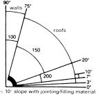
Corrugated cement fibre (1)board with ridge and eaves components 0.2 kN/m<sup>2</sup>
