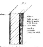
facing panel of plastered wood fibre board; light construction panels 15mm plaster; 115mm pumice concrete masonry; 16mm expanded styrofoam; 25mm light wood wool building panels nailed, with large separation between nails; 20mm gypsum-sand-plaster
