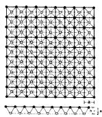
Space structure grid of semioctahedrons and tetrahedrons parallel to the edges
