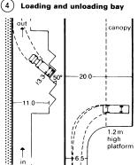
Loading and unloading bay with raised platform and side unloading
