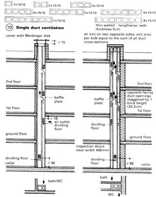
**Branching duct ventilation** system with one main and one auxiliary duct
