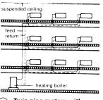
Twin-pipe system with horizontal distribution (standard construction for office buildings)
