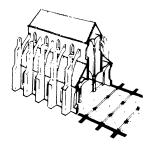
Bothic architecture evolved from cross-vaulting, allowing the vaulting of oblong bays by using the pointed arch (characteristic buttresses and flying buttresses)
