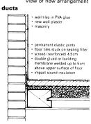
Floor/wall structure in damp areas in a masonry building with wooden beam floors
