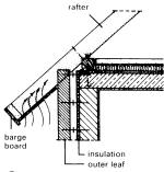
**Eaves detail with cavity** (2) walling
