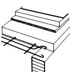
Reinforced concrete slab floor, reinforced in one or two directions
