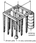
Grid pile and sinking (10)caisson arrangement for deep foundations
