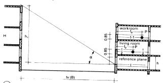
36 Diagram to determine the window widths required
