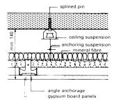
Example of vibration mounting ceiling element
