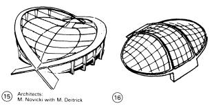
concrete suspended diaphragms with rigid edge beams can create economical and impressive buildings  $\rightarrow$  (5), and may be used as basis for cantilever constructions  $\rightarrow$  (6).
