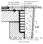
Tanking at junctions of slab bearing on retaining wall
