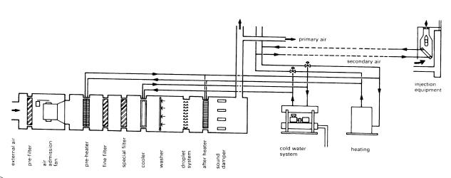
1 High-pressure air conditioning system (System LTG)
