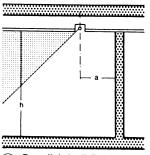
Downlight/wall floodlight, distance from wall: a = 1/3h
