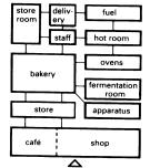
Functional diagram for a bakery: good ventilation needed, possibly dehumidify
