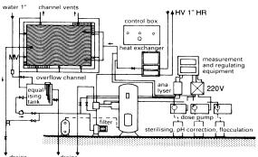
(3) Servicing diagram for pool with overflow channel
