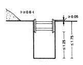
Partly secured excavation
