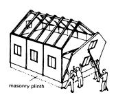
Panel construction uses large prefabricated wall panels, which are quick and inexpensive to erect
