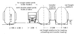
Lay-out of yard for loading and unloading
