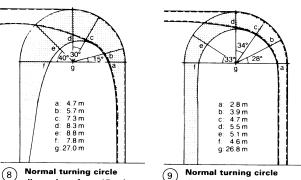
(9) dimensions for a 15 m long dimensions for a truck with articulated truck a rigid chassis and long wheelbase
