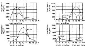
(21) Examples of radiation intensity on vertical surfaces facing in various directions on cloudless days in winter (Dec.) and summer (June)
