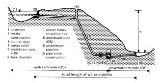
Power station with high-level reservoir and long supply pipe line (underground)
