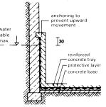
12 Subsequently constructed tanking
