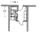
Prefabricated bathroom with kitchen utility wall
