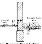
4 Damp-proofing of building with no cellar and with non-habitable room use; floor at ground level
