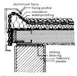
Flat roof edge with open sliding joint
