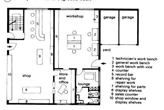
(3) Example of an electrical repair (ground floor)
