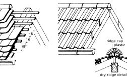
Double roof (plain tiles) heavy roofing, 0.6 kN/m<sup>2</sup>, 34-44 tiles/m<sup>2</sup>
