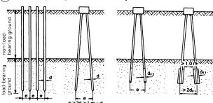
4 Requisite pile separations for driven piles
