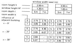
37 Determination of the required window widths (ww) with different room dimensions and interference from various adjacent building (extract)
