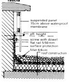
Chimney connection with suspended facia panel
