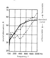
Airborne sound insulation of the wall  $\rightarrow (1)$  from measurements by Prof. Gäsele: sound insulation without covering -7 dB; with covering +2dB
