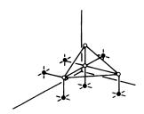
each joint in the three-dimensional space must be fixed by three members rigid so, to achieve kinematic stability:
