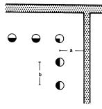
3 Downlight/wall floodlight, separation between lights: b = 1-1.5a
