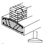
Yet wider foundation in the form of a steel reinforced concrete plate
