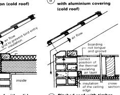
Pitched roof with timber Pitched roof with solid beam ceiling
