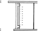
Winter day: incident solar radiation heats the air between the pane and the Trombé wall; room air is circulated through the lower and upper flaps and thus heated
