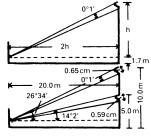
To be readable at a distance of, say, 700 m the width w of the letters must be: ≥ 700 × 0.000291 = 0.204; height h is usually 5w: 5 × 0.204 = 1.020 m
