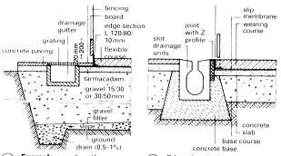
Example construction; drainage suitable for cohesive ground
