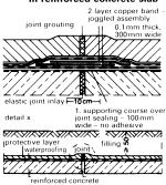
10 Tanking over expansion joint in reinforced concrete slab; thermal insulating screed
