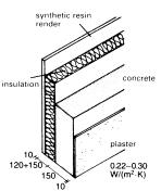
Concrete with bonded insulation panels
