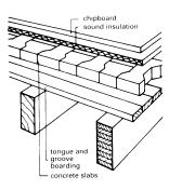
2 Timber joist/laminated beam floor construction with exposed floor underside
