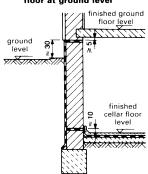
8 Damp-proofing of building with cellar; masonry walls on strip foundations
