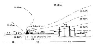
1) Isophonic map: effect of an earth bank or noise shielding wall on sound levels
