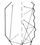
For the music listener, early sideways reflections are better than ceiling reflections, even at very low delay times (asymmetry of the acoustic impression), since each ear receives a different signal. Narrow, high rooms with geometrically reflecting walls with multiple angles and diffusely reflecting ceilings are the simplest from the point of view of room acoustics.
