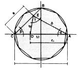
arc of the circle at A with AB results in point D on AC =  $c_1$ ; arc of the circle at C with CM results in point E on arc of BD = a; segment DE approximately corresponds with ½ of the circle's circumference  $\triangle$  D
