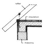
Rafter ends fixed with bolts into downstand beam
