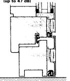
(6) Aluminium/timber combination casement window (up to 40 dB)
