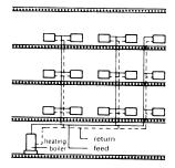
Twin-pipe system with distribution from below and vertical rising branches
