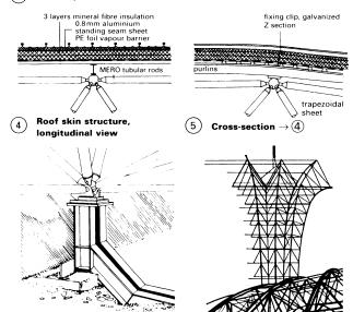
$\begin{array}{c} \textbf{70 cm high support allowing} \\ \textbf{one-way movement} \rightarrow \boxed{3} \end{array}$
