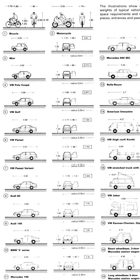
The illustrations show dimensions, turning radii and weights of typical vehicles with particular reference to space requirements and regulations for garages, parking places, entrances and passages.
