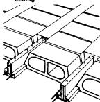
Prefabricated reinforced concrete component floor with non-load-carrying filling blocks
