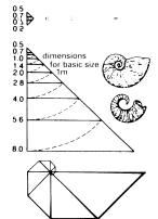
The geometric series for the length of members with the factor \2 and the natural pattern for the geometric series: shells of Ammonites
