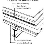
Composite steel/concrete floor
