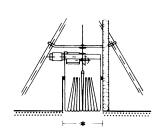
Partitioning curtain with pulley system mounted in a sound absorbing recess
