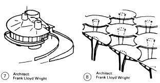
Typical characteristics are cantilevered floors on beams (5) from tower cores  $\rightarrow$  (6), or house core supports  $\rightarrow$  (7), or as mushroom structures  $\rightarrow$  8.
