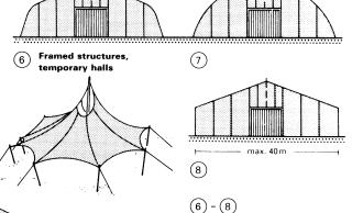
Temporary buildings with supporting structures of wood, steel or aluminium; maximum span 40 m; prefabrication for
