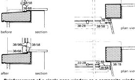
Reinforcement of a single-pane window as a composite window
