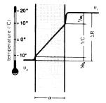
Principle of heat transfer through a component
