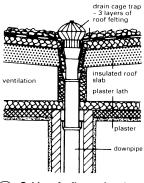
Cold roof - flat roof outlet, insulated in void
