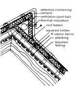
Ridge ventilation on a sloping cold roof (indoor swimming pool)
