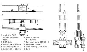
Cable clamp, showing roof construction
