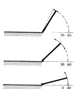
South-facing surfaces inclined at an angle of 55–65° provide optimum utilisation of solar energy during the cold winter months
