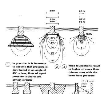
Intersection of (4) foundation influence lines causes danger of settlement and crack formation (important when new building is adjacent to old building)
