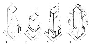
1) and 2) Curved surfaces reduced wind load by up to 25%,
