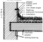
Wall connection zinc sheet (10) angle and flashing
