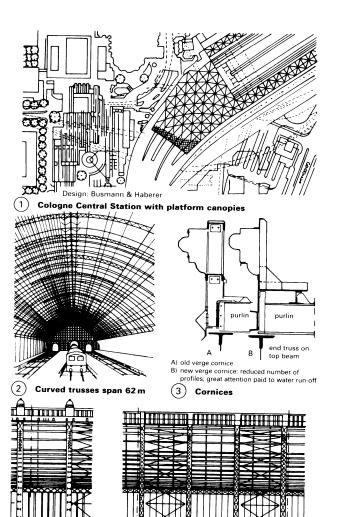
Old wind bracing installed right down to platform; new bracing with strengthened curved trusses in lower area
