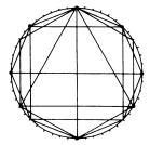
Octagonal coordination system for columns made of squares, each subdivided into six façade elements, 48 angles developed from a triangle → 13
