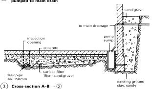
water repellent covering waterproof concrete existing ground clay, sandy 71177 existing drainage ground clay horizontal filter layer sandy gravel drainage horizontal mixed infill sandy gravel coarse vel/rubble 32–63 mm perforated drainpipe ith 20 mm dia. base concrete base concrete infil
