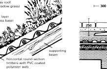
Transition from road surface to intensive roof
