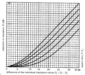
(11) Determination of reduction in insulation
