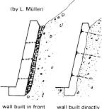
wall built in front of (and away (bonded) onto from) rock wall built direct (bonded) onto rock
