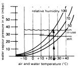
e.g. water temperature t<sub>w</sub> 27°C: evaporation limit in use 36mbar (30°C/84% humidity) and 28mbar when still (30°C/65% humidity)
