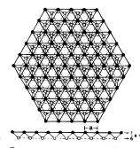
Space structure grid of octahedrons and compressed format
