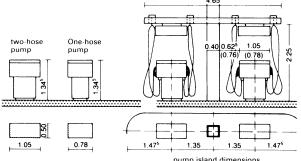
pump island dimensions (short island, two 2-hose pumps) (1) Pumps 0.715 0.715 2.25 8 4.20 roof + light support column 0.58 0.58 0.39 0.40
