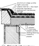
Plat roof with membrane waterproofing
