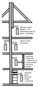
Connections to the exhaust gas stack
