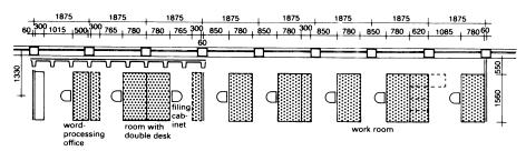
With standard desks (size 0.78 × 1.56m), a division of 187.5 is suitable for a ribbed/slab-and-beam floor having a 62.5 grid module (Koenen floor) with normal formwork. Better for movable partitions
