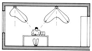
Orrect arrangement of lights in relation to work position: light from the side
