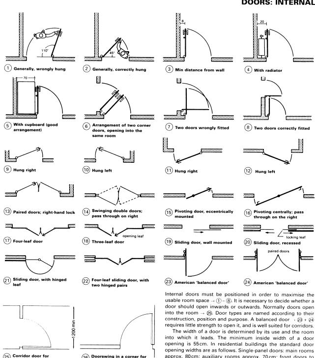
usable room space  $\rightarrow$  1 - 8. It is necessary to decide whether a door should open inwards or outwards. Normally doors open into the room  $\rightarrow$  25. Door types are named according to their construction, position and purpose. A balanced door  $\rightarrow$  23 + 24
