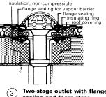
sealing and foam glass insulation material, underside embedded in concrete ('Passavant') scale 1:10
