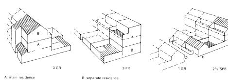
number of storeys gable roof single-pitch roof flat roof
