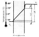
Principle of heat transfer through a component
