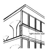
Reinforced concrete mushroom structure with light steel supports in outer wall between windows → p. 38 In the earliest civilisations, building form was dictated by the techniques of binding, knotting, tying, plaiting and weaving. Building in timber followed later, and in nearly all civilisations became the basis for architectural form (see the example of the Greek temple  $\rightarrow$  1) and 2).
