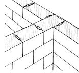
Aerated concrete blocks with cemented joints: 1 mm
