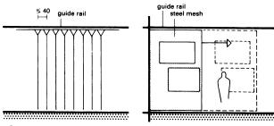
Painting store with sliding steel mesh frames on which pictures can be hung as desired and be available for study
