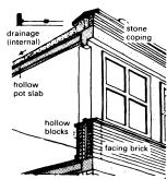
6 Reinforced concrete building with supports in external wall, fronted by outer leaf of parapet wall supported by the cantilevered floor
