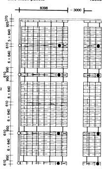
Detail of a sliding rack system for storing files
