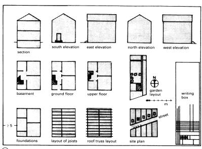
(1) Suitable arrangement of a construction drawing
