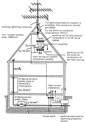
(6) Scheme for lightning protection earthing
