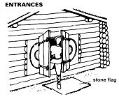
5 Ab 1000: log cabins had low doors, high thresholds; no windows; lit through an opening in the roof ROOM CONNECTIONS
