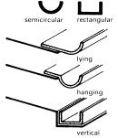
Shape and position of the guttering
