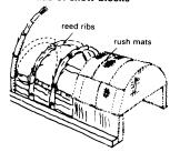
As well as circular domes, barrel vaulting was widely used (e.g. Mesopotamia: reed ribs were covered with rush mats)
