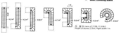
All stairs without landings, whatever the type, take up almost the same surface area. However, - (11) the distance from the top of the lower floor stairs to the foot of the next staircase can be considerably reduced by curving the steps ightarrow igl( igl) - igl( igr) . Therefore curved steps are preferred for
