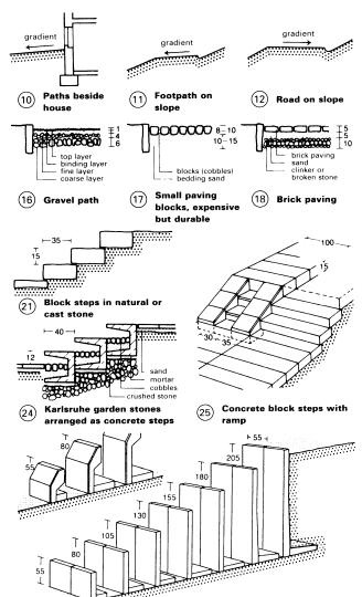
Ready-made concrete sections for retaining walls
