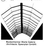
Structure made of loadbearing glazing bars that span the space
