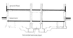
(4) Cross-section of lab with well-positioned central corridor
