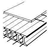
7 Prefabricated reinforced concrete I-beam floor
