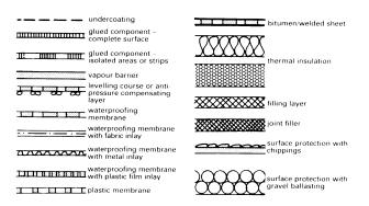
(12) Key to representation of roof covering components
