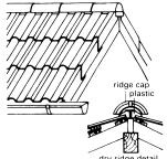
Concrete roof tiles, 0.6-0.8 slope 18° kN/m²
