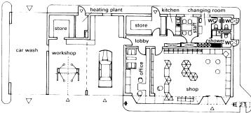
Corner filling station on an enclosed site. This is used only in exceptional cases, and usually not suitable for trucks
