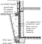
Protective layer of fibre cement boards
