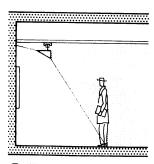
Wall flood on a power supply rail; partial room illumination
