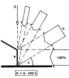
The dependency of the level of incident radiation on a surface on the angle of incidence
