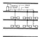
Twin-pipe system with distribution from above and vertical branches
