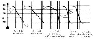
temperature of the inner surface of the wall  $\theta_{w_{\ell}}$  increases as the thermal insulation is improved
