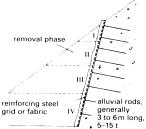
in steps, material removal from top to bottom, with immediate securing using sprayed concrete and reinforcing steel fabric and alluvial rods
