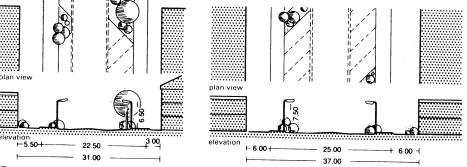
15.00 (5) With parking on one side of the road Parking spaces between (6) With parking on both sides of the road the houses
