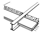
Steel supported floor with pre-cast reinforced pumice concrete infill units
