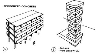
For many building types, building regulations require fire resistant or even fire proof construction and encased steel members consequently resemble reinforced concrete.
