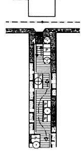
(A3) + B1 + B2 + B3 + B4 + B5 + B6 + C1; layout for driving, parking and walking in a common (mixed) area so multiple use of the whole road area is possible; speed is limited to 'walking pace' (or 20
