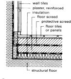
Floor construction with (8)ceiling for bathrooms with shower
