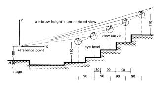
2 Drawing for calculating view curve
