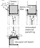
Moisture damage to outer cladding
