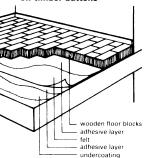
Wooden floor blocks, glued down on even, smoothed concrete underlayer (specialised finish)
