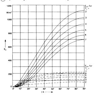
19 Horizontal irradiances due to the sun  $E_{eS}$  and the (cloudless) sky  $E_{sH}$ , with various turbidities  $T_L$ , as a function of the elevation of the sun  $\gamma_e$
