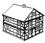
In contrast, this framed building has isolated windows and corner struts; the panels are interlaced wickerwork with mud or clay rendering (wattle and daub)
