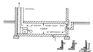
(2) Boiler room (min. 8 m³) needed for heat output ≥ 50 kW
