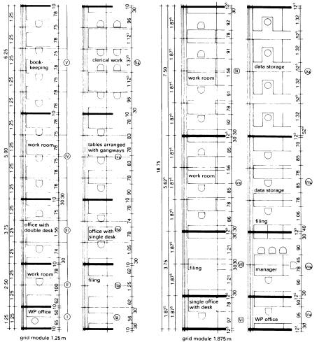
(1) Minimum room width according to window grid modules
