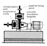
Equipment installation with elastic insert in foundation
