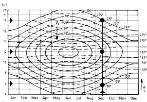
$\bigcirc$  Solar azimuth  $\alpha_{\rm s}$  and solar elevation  $\gamma_{\rm s}$  at 51° latitude (English south coast: Southampton, Brighton) as a function of time of year and time of day
