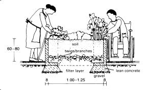
(8) Raised bed made from prefabricated concrete units
