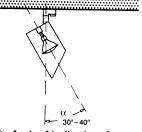
6 Angle of inclination of spotlights illuminating objects and walls: α = 30°-40° (optimum)
