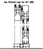
(5) Aluminium thermally separated sliding window (up to 35 dB)
