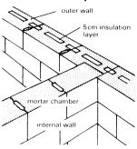
Building blocks with 5 cm insulation layer and mortar filled cavities
