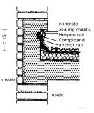
Wall connection: flanged connection with anchorage
