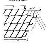
Pantile roof, lighter, 0.5 kN/m<sup>2</sup>
