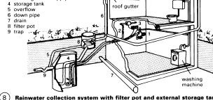
Rainwater collection system with filter pot and external storage tank
