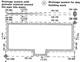
Example of an arrangement of drainpipes, inspection and cleaning access in a ring drainage system
