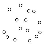
Arrangement of atoms: metal in gaseous phase
