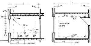
32 Daylight ratio with side lighting, showing the reference plane and the variation in daylight in the internal area
