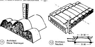
shell  $\rightarrow$  10, rhythmically arranged transverse shells  $\rightarrow$  11, rows of shells with inclined supports at neutral points  $\rightarrow$  (2).
