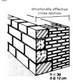
Mixed masonry with structurally effective crosssection
