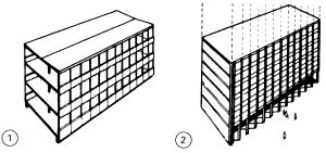
Slender supports give steel-framed construction the lightest possible appearance  $\rightarrow$  ①. However, this form is not permitted everywhere. Exterior unenclosed supports are rarely allowed  $\rightarrow$  ② but, if combined with externally visible
