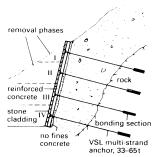
in steps, material removed from top to bottom and immediately shored with wall elements and alluvial anchors (Brenner motorway)
