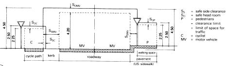
(19) Clearance dimensions for motor vehicle traffic
