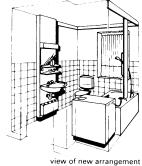
Pipes/lines laid in surface-mounted ducts
