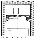
Top of shaft with Neoprene bearing layer
