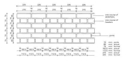
(6) A wall elevation illustrating brick sizes in the UK
