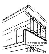
Reinforced concrete structure with internal columns, cantilevered floor and continuous ribbon windows
