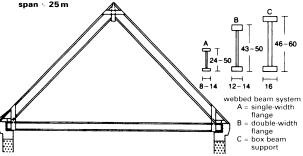
4 Couple close roof with webbed rafters, glued timber construction; ratio of profile height to supported span = 1:15-1:20
