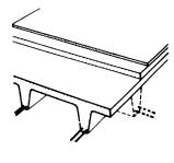
In situ reinforced concrete ribbed floor, rib separation ≤ 70 cm, rib width ≥ 5 cm
