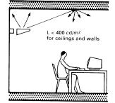
Lights which can generate reflections should have low luminance levels in the critical incidence range
