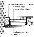
Possible solution for (10) impact sound insulation on a timber joist ceiling
