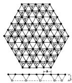
Space structure grid of octahedrons and tetrahedrons with regular cut-outs in the
