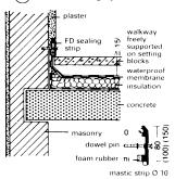
Wall connection with FD (12)sealing strip (walkway)
