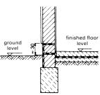
6 Damp-proofing of building with no cellar; low lying floor at ground level
