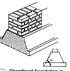
Chamfered foundation in unreinforced concrete
