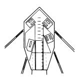
Transfer of loads from the cables to the cross-beams on a mast head
