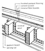
Timber joist/laminated beam floor construction with ceiling
