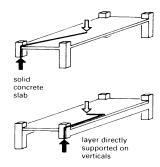
Floor support structure with a single load-bearing layer
