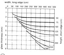
recommended glass thicknesses for inside and outside panes of double glazing up to 20.00 m installation height (wind load = 1.2kN/m² or 1200 Pa)
