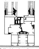
(4) Aluminium thermally separated composite casement window (up to 47 dB)
