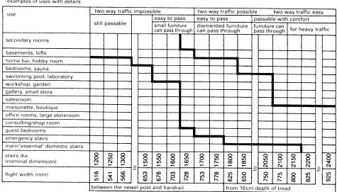
(13) Determination using minimum sizes for spiral stairs of all types
