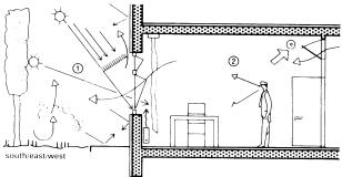
Heat reduction through solar protection with simultaneous cooling by means of passive precautions (e.g. office buildings without air conditioning)
