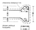
Hammerhead turning place for cars
