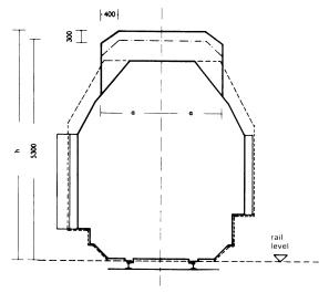
for existing superstructures, tunnels and engine shed doors when electrification takes place
