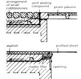
11) Tanking at connections to windows and access openings
