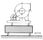
9 Double elastic suspension for ventilator
