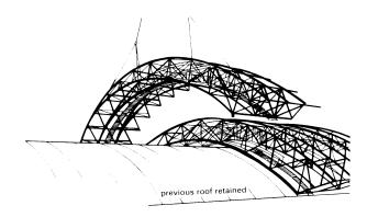
(8) Lifting a space frame section into place  $\rightarrow$  (7)
