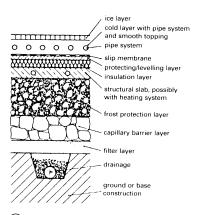
(5) Detail of surface pipes → ④
