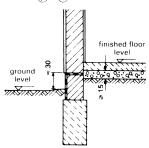
3 Damp-proofing of building with no cellar and with non-habitable room use; hardcore at the level of the damp-proof course
