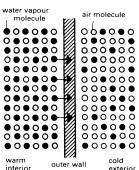
Water vapour moves from warm interior of a building, hindered by outer wall, to cooler outside air; air molecules move inside in exchange
