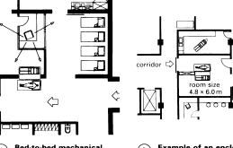
1 Bed-to-bed mechanical transfer device separates operating department from entrance area (by Maquet)
