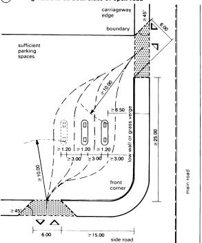
Filling station with fuel pump islands obliquely angled in an (2) enclosed site (mainly for one-way traffic)
