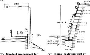
4 Standard arrangement for noise shielding walls on roads
