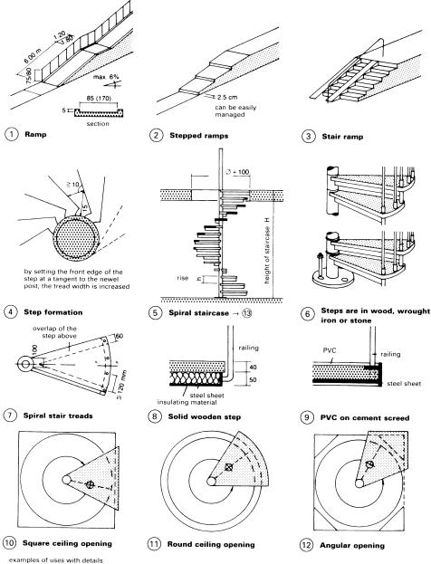
Ramps should be provided to allow wheelchair users and those with prams or trolleys to move easily from one level to another  $\rightarrow$  (1) – (3).
