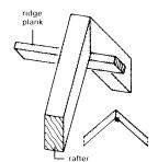
Ridge details of purlin roof; ridge plank to align the ridge
