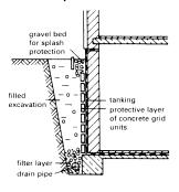
Protective wall of concrete grid units
