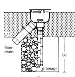
Floor drain with groundwater pressure balance
