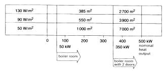
Central heating boilers with a heat output > than 50 kW require individual boiler rooms
