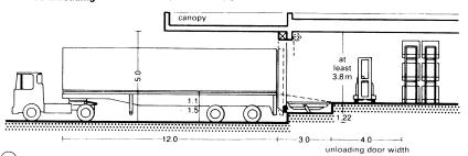
Section through a loading bay with an adjustable loading platform
