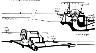
Power house with inclined ducted turbine and spur
