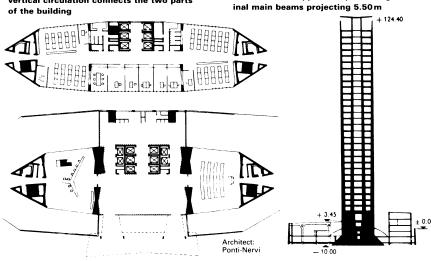
Load-bearing structural towers  $\rightarrow$  (5) with pre-stressed floors with spans up to 24m but only 0.75m in depth in between
