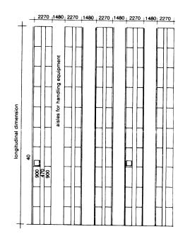
Detail of a plan for a pallet rack store for ball bearings (structural elements of shed concealed in shelving)
