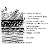
Roof garden on a warm roof - protective layer could be replaced by shredded rubber sheet
