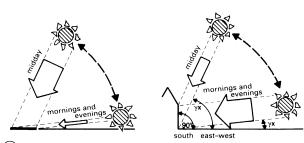
(20) Comparisons of the direct radiation on horizontal and vertical surfaces at various positions of the sun during the day. The level of incident radiation on a surface depends on the angle of that radiation (x).
