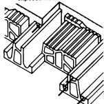
Floor assembled from reinforced concrete ribs with cellular clay infill components
