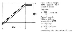
(14) Reinforced concrete staircase unit
