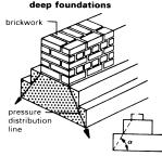
Widened, stepped (12)foundation in unreinforced concrete
