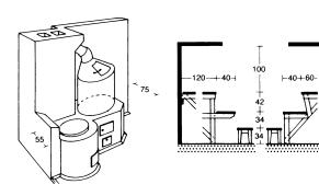
Finnish sauna oven with water container (also useable for washing clothes)
