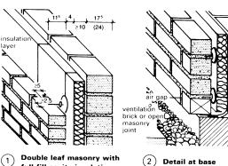
Double leaf masonry with full fill cavity insulation
