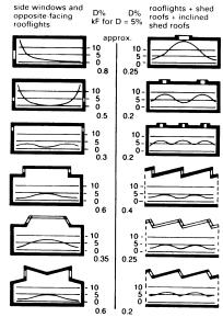
kF = window area/floor area = 1.6 values required for Dmin = 5% are shown for comparison
