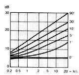
read off the shielding ordinate as a function of angle  $\alpha$  · (8), and height (m)/sound wavelength example:  $\alpha$  = 30°, h = 2.50 m: at 500 Hz (med. freq. range) = 340/500 = 0.68; wavelength is  $h/\lambda$  = 2.5/0.68 = 3.68, hence shielding effect = 17 dB
