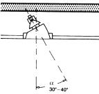
5 Angle of inclination of directional spotlights and floodlights: α = 30°-40° (optimum)
