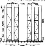
Section through pallet rack for stacker loading. U-section steel guide rails for stackers
