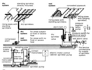
(1) General arrangement of a sprinkler system
