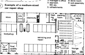
Usually single storey of light steel construction or prefabricated elements. Single-span shed without columns is preferable. Choose an appropriate module to allow extension.
