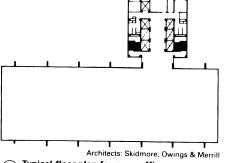
Typical floor-plan for open offices; lavatories separated. External columns allow furniture to be positioned anywhere. 17.50m free span
