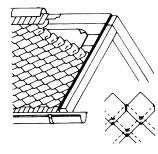
English slate roof with cement fibre boards. 0.45-0.55 kN/m<sup>2</sup>
