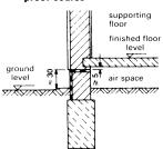
5 Damp-proofing of building with no cellar; floor with ventilated air gap between floor and ground level
