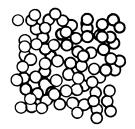
2 Arrangement of atoms metal in liquid phase
