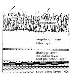
Layer construction of a cultivated roof
