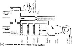
Several handling stages are usually involved in ventilation and air conditioning. Filtering; air heating; air cooling; and washing, humidifying and evaporative cooling are discussed on this page. For ventilation and damping  $\rightarrow$  p. 107.
