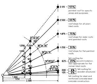
Roof slopes at regular intervals appropriate to specified types of roof construction
