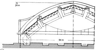
(5) Section through main hall, with travelling internal scaffolding
