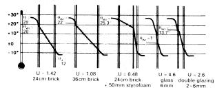
temperature of the inner surface of the wall  $\theta_{\text{wr}}$  increases as the thermal insulation is improved
