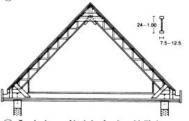
Couple close roof in timber framing with lifetime guaranteed glued joints with 45° inclined struts as twinned supports over
