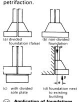
Application of foundations on dividing lines and movement joints
