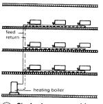
6 Single-pipe system with special valves and horizontal distribution
