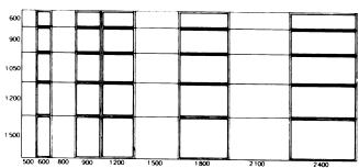
Note: Above diagrams intended for general guidance on overall sizes only; no distinction made between types of opening light; some sizes, fixed lights only (designated fl) obtainable in standard ranges
