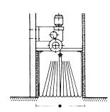
Partitioning curtain to one side of a beam; with sound absorbing recess
