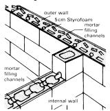
Special wall blocks with (10) insulation and mortar filling channels
