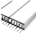
Hollow core, pre-cast concrete flooring units with twisted, pre-stressed steel wires
