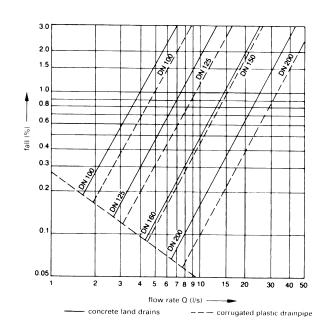
(11) Measurement nomogram for drainage pipework
