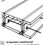
U-section reinforced concrete beams bolted to provide lateral stiffness
