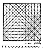
Space structure grid of (6) semi-octahedrons and tetrahedrons in a rotated position (45°)
