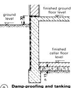
9 Damp-proofing and tanking of building with cellar; walls of concrete
