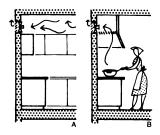
(13) Extractor fan on outer wall (A), better if directly above cooker (B)
