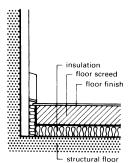
Plaster applied down to floor level before floor screed prescribed for porous walls
