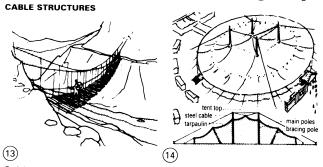
Cable structures for long spans have been in use since early times - 13. Circus tents are the best-known lightweight suspended diaphragm structure  $\rightarrow$  (4). Modern reinforced
