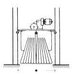
**Partitioning curtain** between two beams
