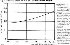
(4) Curve of upper limit for comfortable room air velocities
