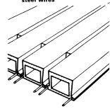
8 Prefabricated reinforced concrete hollow beam floor
