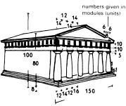
The walls slanting suitably inward seem vertical; steps, cornices and friezes when bowed correctly upwards look horizontal
