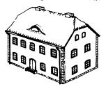
From a later period: framed openings and corners with carefully formed, dressed stones; the rest of the walls in rubble masonry which was then rendered
