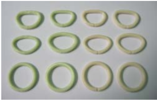
Fig. 6. Different polyurethane resin prototypes obtained under vacuum casting in silicone moulds. Both open and closed rings were made to analyse alternative performances.
