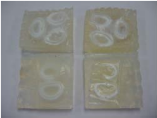
Fig. 5. Silicone Moulds obtained from stereolithographic models
