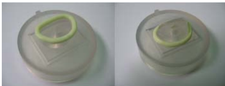
Fig. 8. Alternative device with interchangeable heads (depending on the type of ring to be implanted). Deformation induced at 80 °C to obtain a temporary shape.
