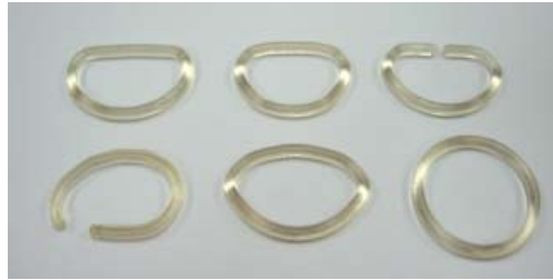
Fig. 4. Physical models obtained by laser stereolithography from files containing the 3D part geometry
