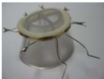
Fig. 9. Active ring with heating resistances and with the temporary shape already applied. It is ready to be implanted and subsequently activated.
