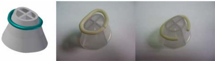
Fig. 7. Design and prototype of base for programming shape-memory effect. Deformation induced to the ring at 80 °C to obtain a temporary shape.
