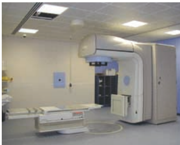
Figure 39.1 Siemens Primus Dual Energy 6/15 MeV Linear Accelerator with electron facility installed in the Oncology Centre at Addenbrooke's Foundation NHS Trust, June 2003.
