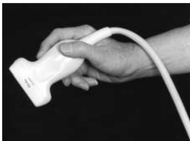
Figure 17.1 A 15 MHz transducer for breast and small parts scanning (Acuson, Mountainview, CA).
