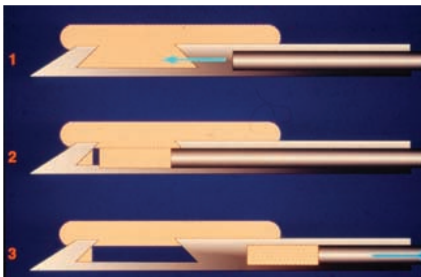
Figure 23.4 Vacuum-assisted core biopsy: mechanism of action. (1) Tissue is pulled into the biopsy aperture by the vacuum. (2) The cutting cylinder separates the tissue specimen from the surrounding breast tissue. (3) The tissue specimen is withdrawn within the cutting cylinder.
