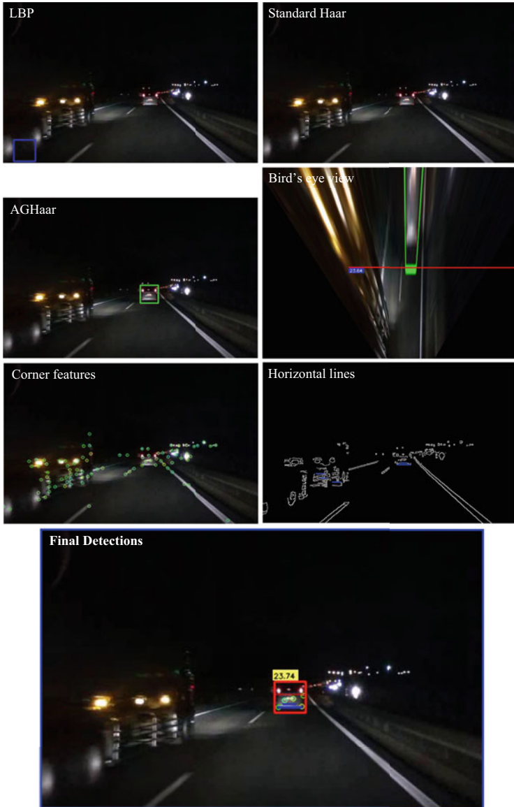
Fig. 7.25 Vehicle detection and distance estimation for situation night . Order of images and descriptions as per Fig. 7.23
