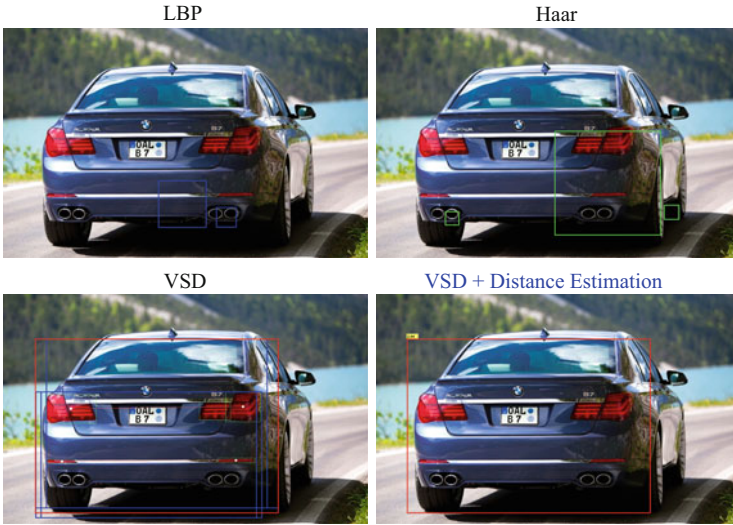
Fig. 7.22 Short-distance vehicle detection and distance estimation with different approaches (Sample 3)
