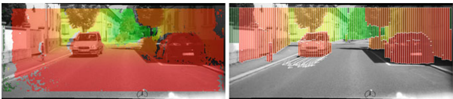
Fig. 2.2 Left : Use of a colour key (different to the one shown in Fig. 2.4) for showing depth data calculated by stereo matching. Right : Illustration of calculated stixels (based on the depth data illustrated above, forming an occupancy grid ), groupings of stixels, and of estimated motion for such stixel groups (Courtesy of Uwe Franke)
