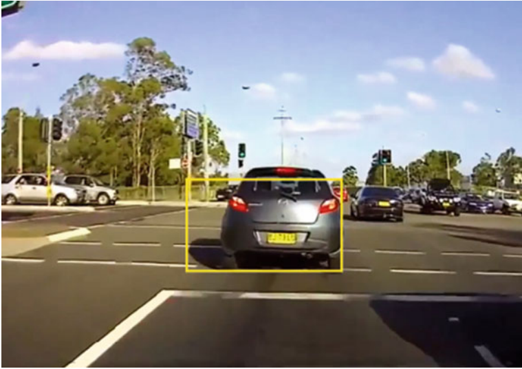
Fig. 7.1 An example of an inaccurate vehicle detection based on underneath shadow
