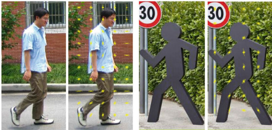
Fig. 4.13 Two sample images and a visualization of their corresponding HOG outputs, assuming a subdivision of a standard-size window into 5 blocks horizontally, and 10 blocks vertically
