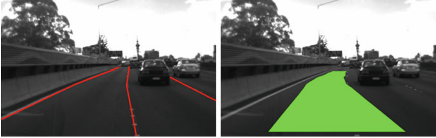
Fig. 2.11 Left: Detected lane borders. Right: Expected area the ego-vehicle will drive in (i.e. the corridor), adjusted to the lane border after crossing lanes (Courtesy of Ruyi Jiang)
