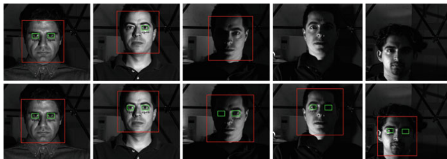
Fig. 5.17 Yale database: face and eye-state detection under difficult lighting conditions; standard classifier ( top ) vs. adaptive classifier ( bottom )
