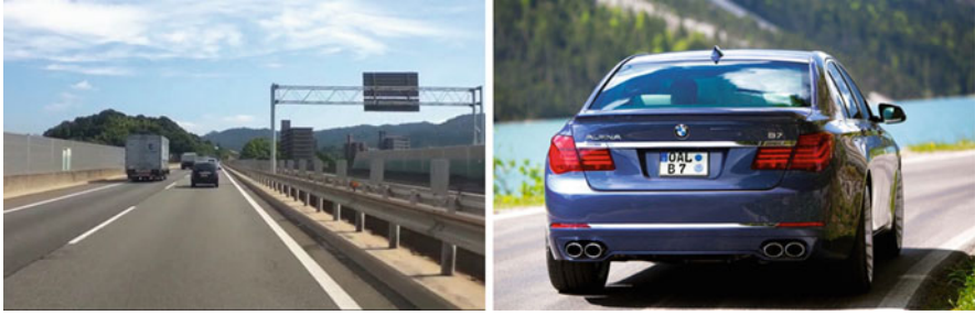
Fig. 7.2 Left: Distant vehicles appearing as plain rectangles, with a shade underneath the vehicle. Right: A close vehicle with multiple edges, shades, and complicated features and details
