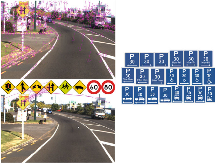
Fig. 2.10 Left, top: Detected relevant features in an input image. Left, bottom: Detected sign due to voting by SIFT features which passed the potential location filter. Right: Diversity of the appearance of the P30 sign in New Zealand (Courtesy of Feixiang Ren)
