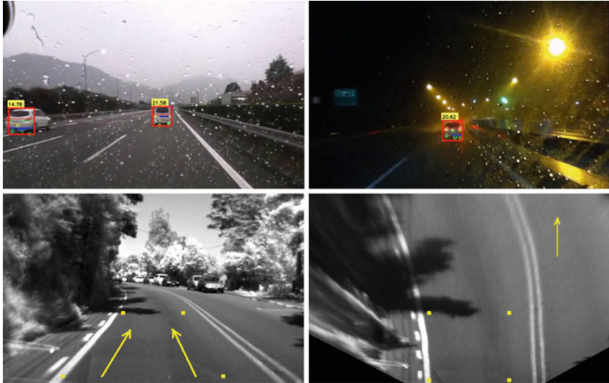
Fig. 2.3 Top : Monocular vehicle detection under challenging lighting conditions, to be discussed later in this book in detail; detected vehicles are also labelled by monocular distance estimates. Bottom : A transform from perspective view into bird's-eye view is used for monocular distance estimates (Courtesy of Ruyi Jiang)
