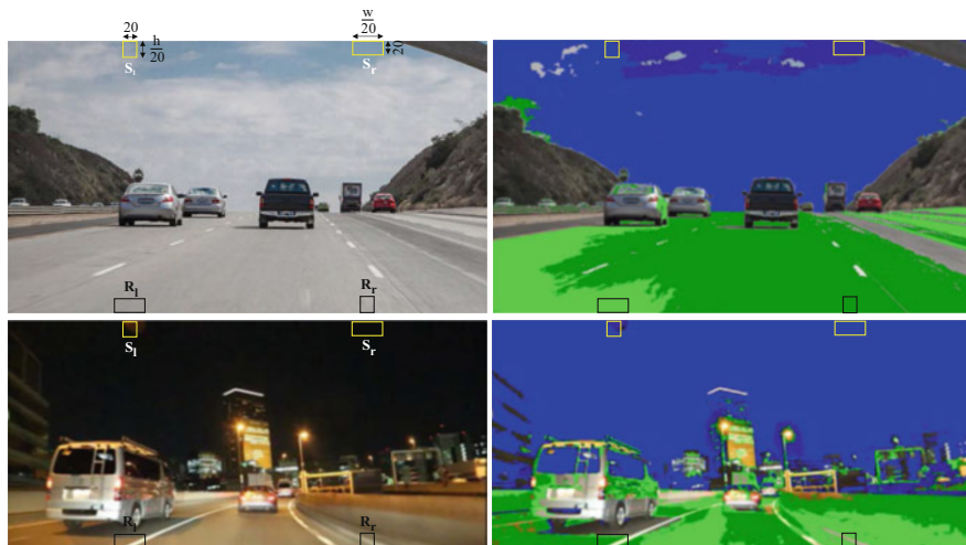
Fig. 7.5 Intensity measurements for road and sky regions under day or night conditions
