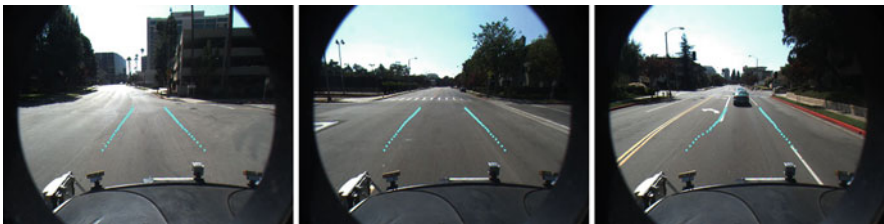
Fig. 2.9 Three examples of data provided by [20] where a used lane detector follows its strategy for detecting lane borders by temporal inference, but where one given frame alone would be insufficient for a judgement of whether the detected border is correct or not. The three images show detected lane borders composed of sequences of individual points (Courtesy of Bok-Suk Shin)
