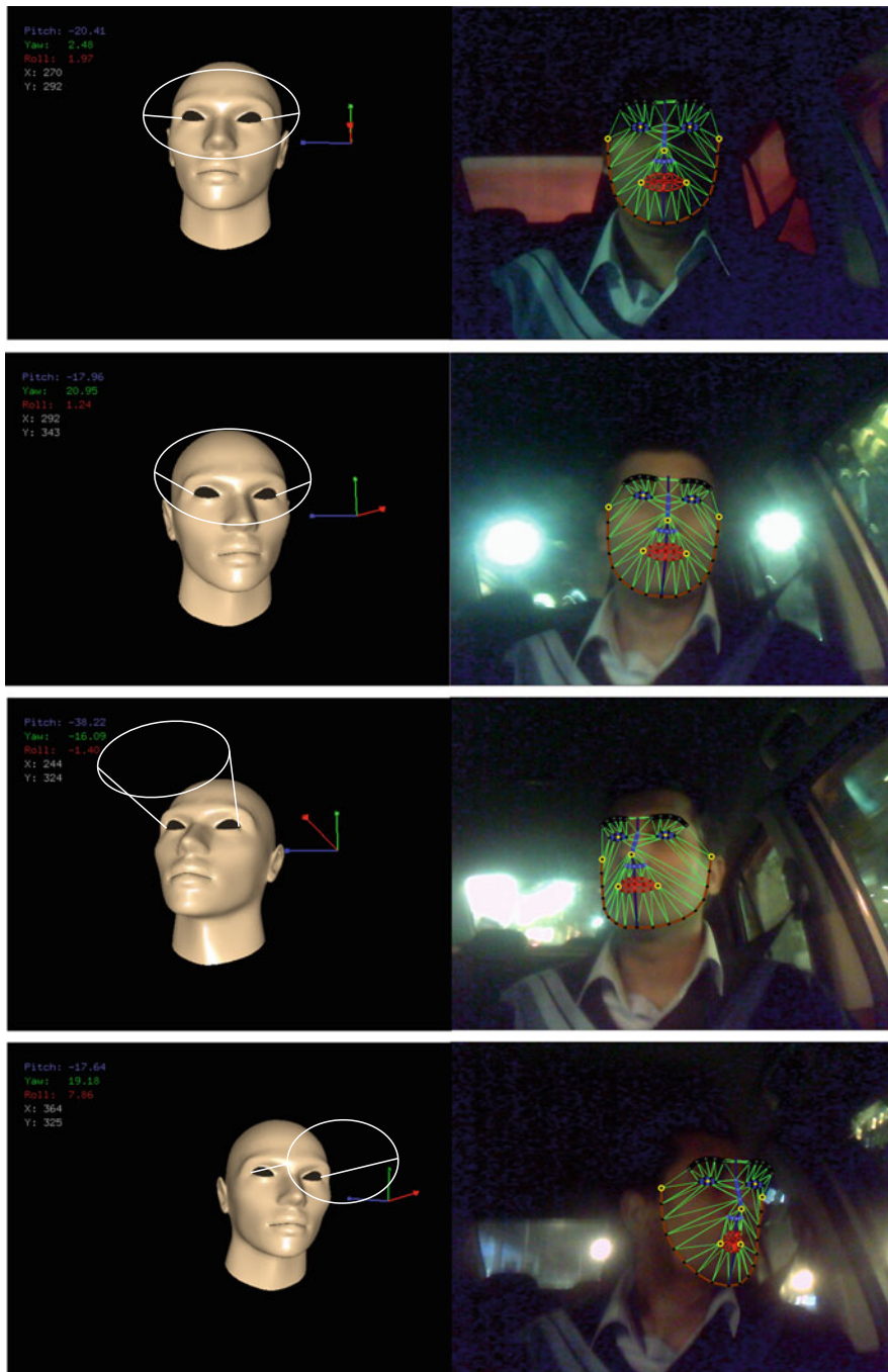
Fig. 6.9 Driver's head-pose estimation based on ASAAM, Fermat-point transform, and EPnP; (Night Condition)
