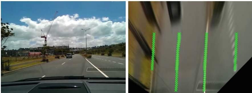
Fig. 1.7 Three detected lanes in a country driving on the left-hand side . Matching with an available e-map simplifies the decision about which lane the ego-vehicle is currently driving in (Courtesy of Junli Tao)
