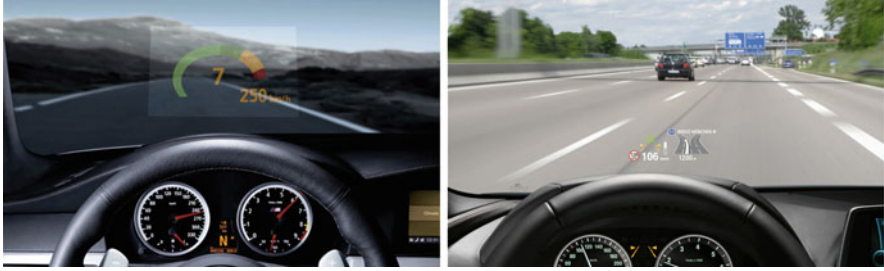
Fig. 1.4 Two examples of a virtual windshield in a BMW. The “7” in the image on the left identifies the current gear (Courtesy of Clemens Dannheim)
