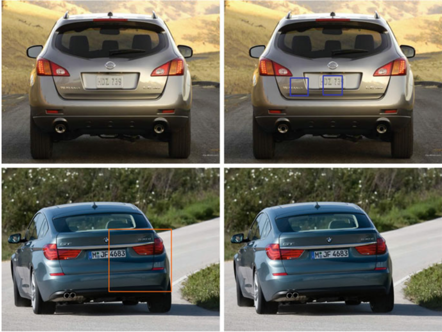
Fig. 7.10 Failed detections or false positive detections for close-up vehicles. Left : Haar-based detections. Right : LBP-based detections
