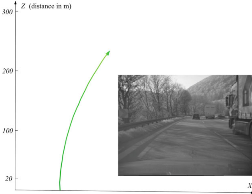
Fig. 2.6 Calculated trajectory for the ego-vehicle of sequence 3 in Data-set 1 of EISATS (Courtesy of Ali Al-Sarraf)
