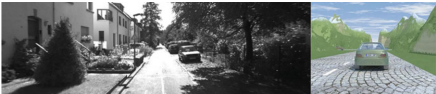
Fig. 1.3 Examples of benchmark data available for a comparative analysis of computer vision algorithms in a traffic context. Left: Image of a real-world sequence provided on KITTI (with approximate ground truth about distances on [118]). Right: Image of a synthetic image sequence provided on EISATS (including accurate ground truth about distances and movements)
