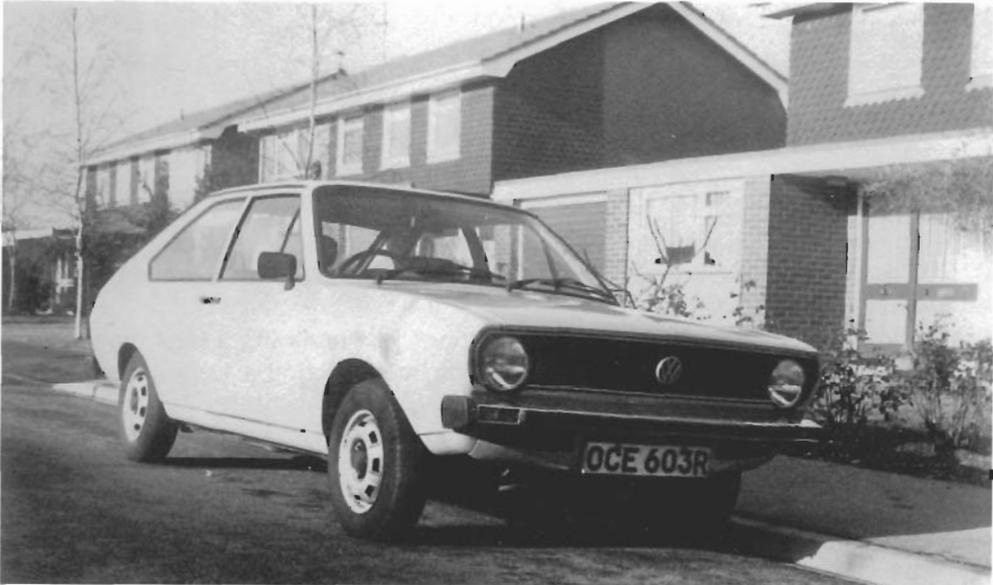
**Fig. 27.2.** The Volkswagen Passat – a typical 1970s pressed-steel body with no separate chassis. For a given material this ‘monocoque’ construction gives a minimum weight-to-strength ratio.
