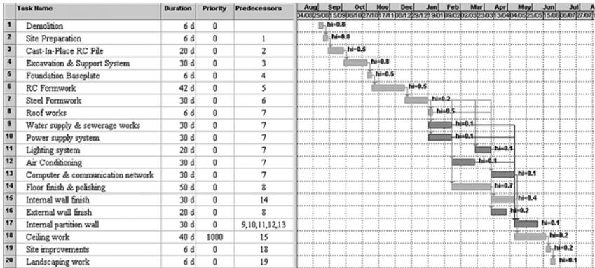
Figure 3.2 Initial schedule of a construction project.
