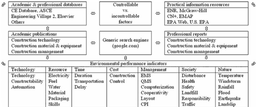
Figure 3.9 The framework for identifying environmental indicators.
