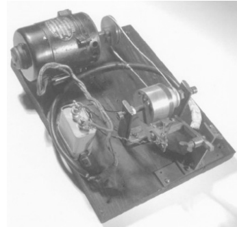
Andrew Booth's prototype magnetic drum of 1947
