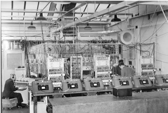
The Elliott Nicholas computer, used for guided bomb trajectory calculations for the Royal Aircraft Establishment, Farnborough (1952).
