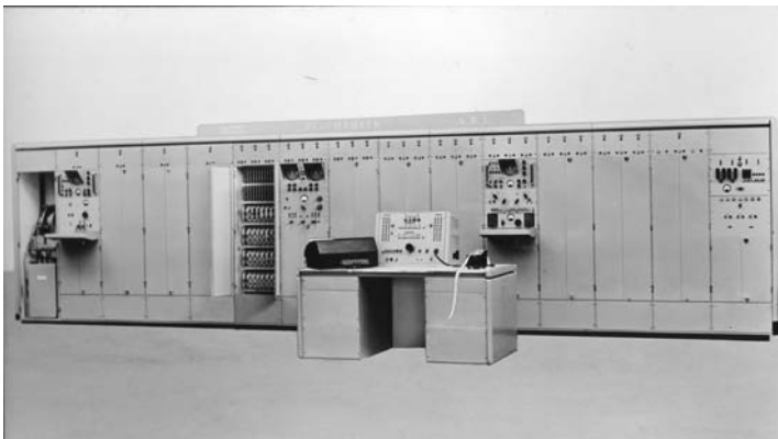
The Elliott 153, for rapid plotting of Direction Finding (DF) signal intercepts at GCHQ's Irton Moor Establishment near Scarborough (1954).
