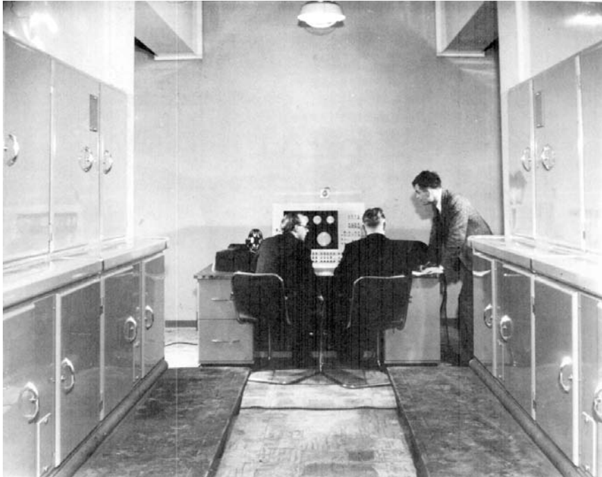
The Ferranti Mark I computer with the operator's control console between the rows of cabinets holding the logic circuitry. The person standing to the right of the console is Alan Turing.
