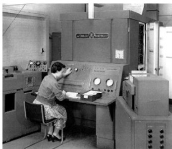
An English Electric DEUCE computer at the NPL in 1956. The pieces of equipment in the left and right foreground are respectively a card reader, used for input, and a card punch, for output.
