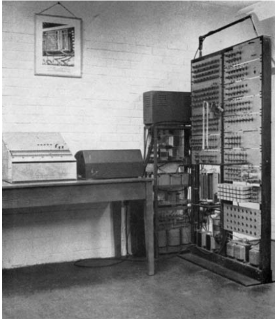
Booth's All-Purpose Electronic Computer , known as APE(X)C and put to use for X-ray crystallography at Birkbeck College, in 1953
