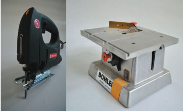
Fig. 4.1 Cutting tools – a jig saw and a special circular saw used by model builders
