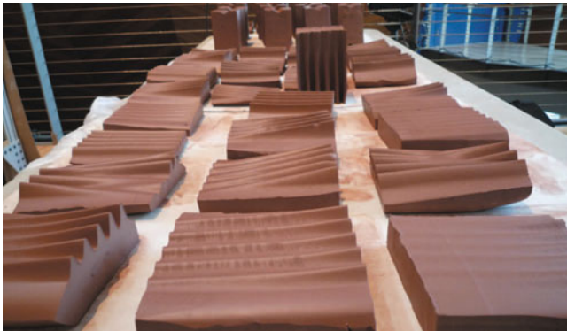
Fig. 4.31 Clay shapes cut with a robot arm, Smart Geometry Workshop 2012
