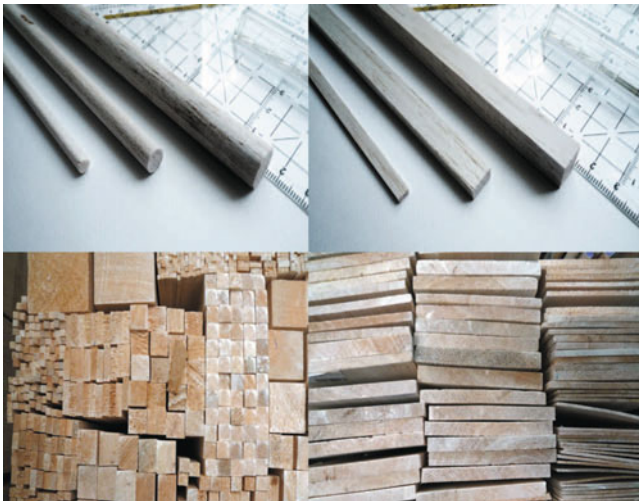
Fig. 4.28 Wood dowels, strips and battens
