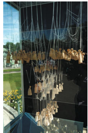
Fig. 2.2 A model of Sagrada Familia by Gaudi. A wire model that can self-generate the form under the influence of gravity and the load. A mirror image (the mirror is on the floor) gives a true image of the final form
