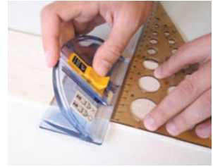
Fig. 5.26 Cutting with a 45-degree blade angle scalpel
