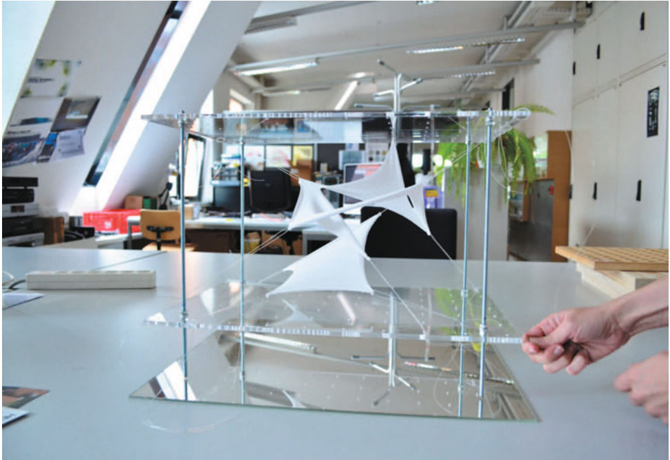
Fig. 7.26 Acrylic glass frame used for experimenting with membrane forms
