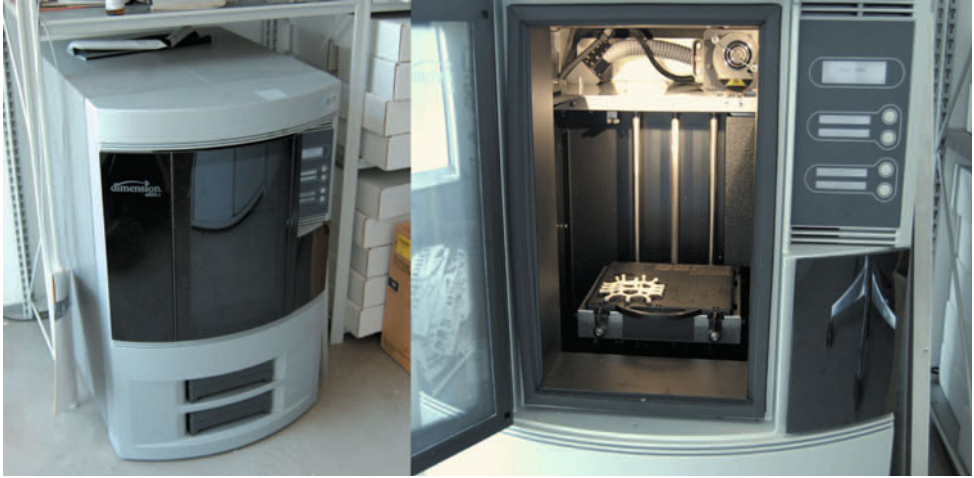
Fig. 6.13 FD printer (left) and a detail showing the modelling basket (right)
