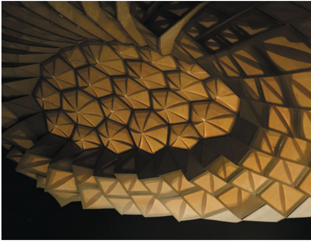
Fig. 4.33 HygroScope project: closed structure as a response to relative humidity within its microenvironment of the glass case
