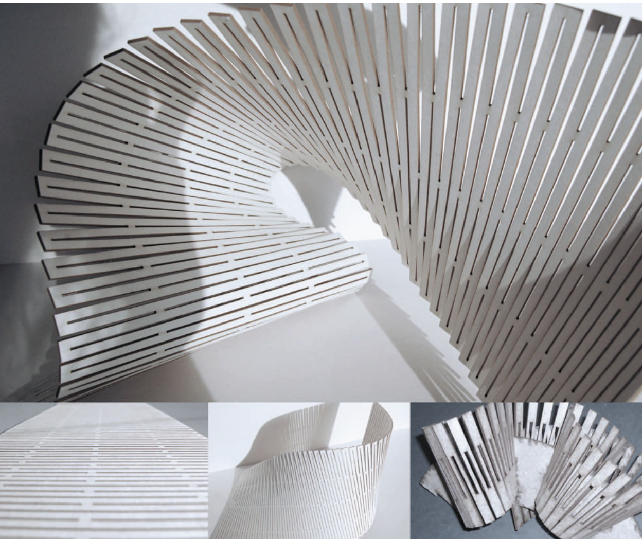
Fig. 3.21 The thickness and elasticity of the material defines different folding possibilities
