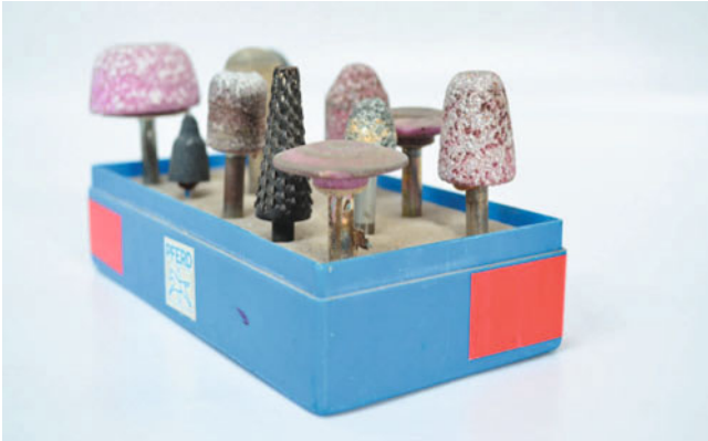
Fig. 4.3 Various kinds of grinding bits used for fine-finishing
