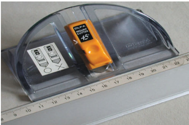
Fig. 4.8 Scalpel for cutting at an angle of 45^\circ
