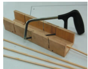
Fig. 5.28 Cutting a rod with a hand saw in a mitre box
