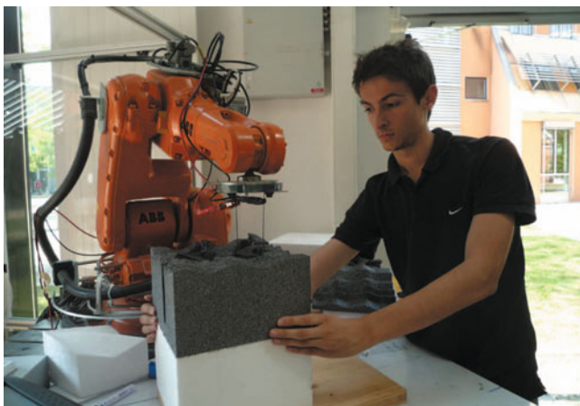
Fig. 6.7 Cutting a part out of an EPS block with hot wire controlled by a robot arm
