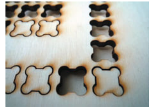
Fig. 5.22 Cutting marks on plywood
