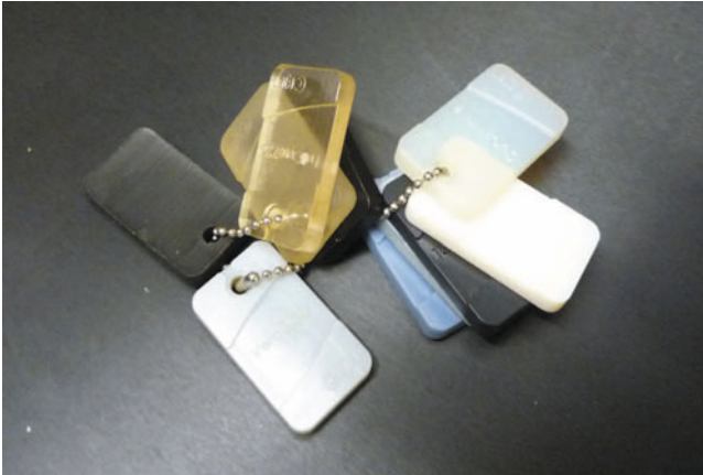
Fig. 6.16 Different kind of material (elastic, transparent) printed with stereolithography method
