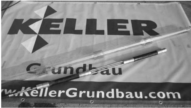
Figure 7.20 Double packer for 2" grouting pipes.
