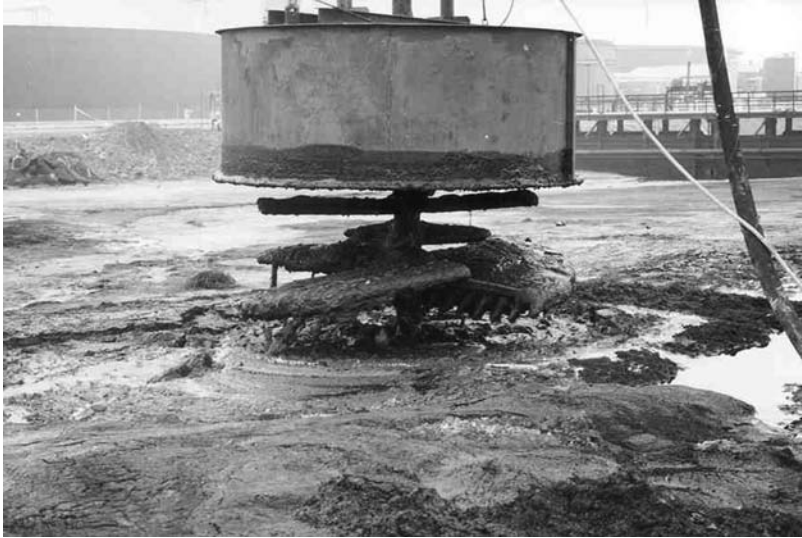
Figure 9.9 SSM mixing tool diameter 3.7 m for the dry method. (Courtesy of Geo-Con Inc.)
