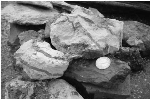
Figure 7.19 Coloured frac sample deriving from grouting in cohesive soils.
