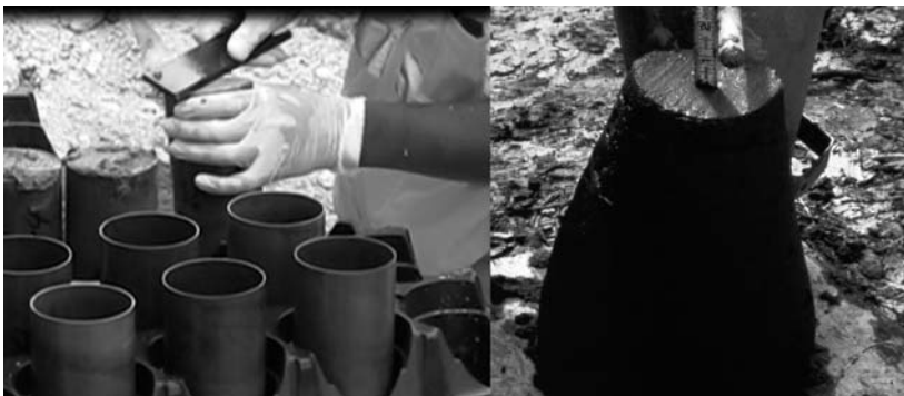
Figure 8.16 Casting test cylinders and measuring LMG slump. (Courtesy of Hayward Baker Inc.)
