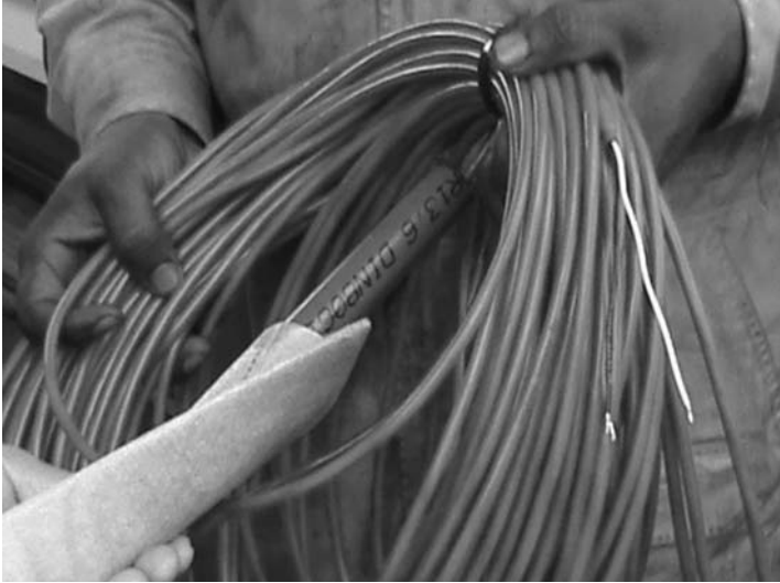
Figure 4.39 Putting piezometer inside a PVD for pore water pressure measurement.
