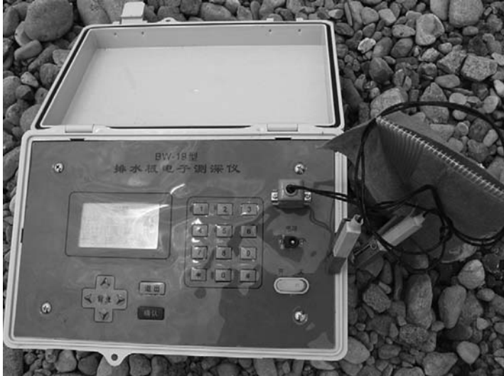
Figure 4.36 Readout unit for the measurement of PVD penetration depth. (From Liu, H.L., Chu, J. and Ren, Z.Y. (2009). Geotextiles and Geomembranes , Vol. 27, No. 6, pp. 493–496.)
