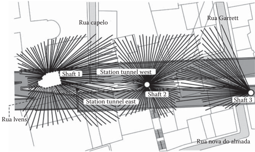
Figure 7.7 Arrangement of shafts and drilling for the installation of grouting pipes for settlement correction in densely built-up area of approximately 15,000 m 2 .
