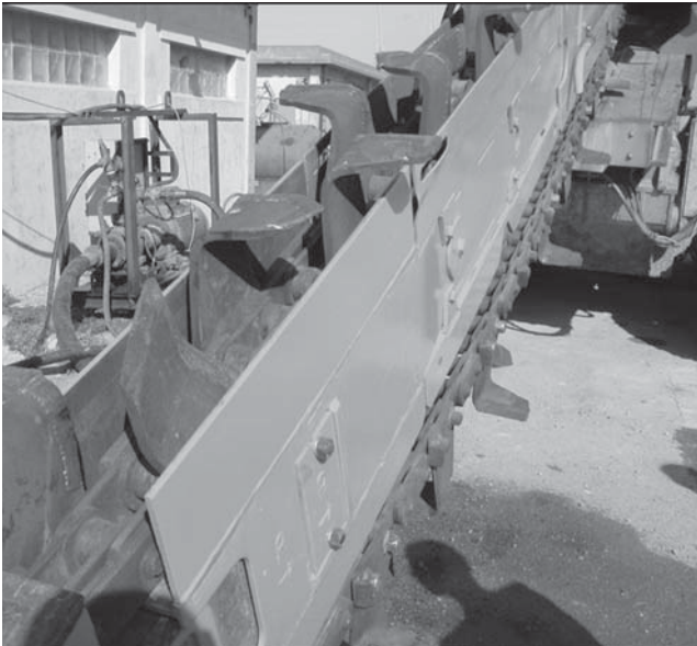
Figure 9.21 TRENCHMIX equipment. (a) Rig in operation on a river dike. (b) Close-up of cutting/mixing teeth. (Courtesy of Bachy Soletanche and Mastenbroek.)
