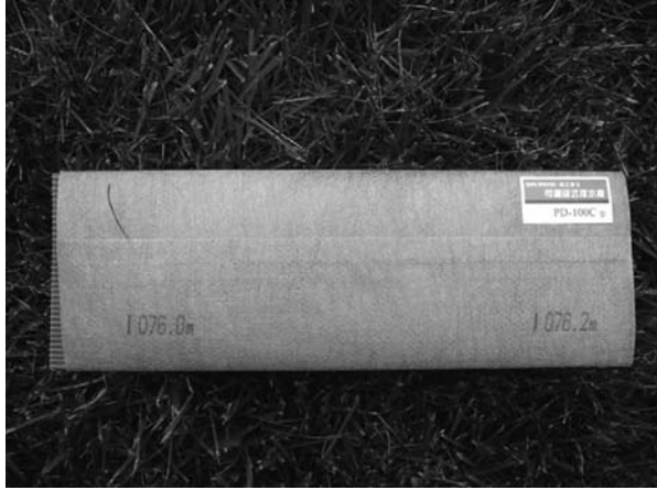
Figure 4.37 PVD with one copper wire embedded for PVD penetration depth measurement. (From Liu, H.L., Chu, J. and Ren, Z.Y. (2009). Geotextiles and Geomembranes , Vol. 27, No. 6, pp. 493–496.)
