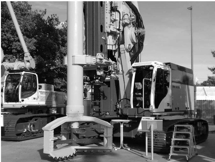
Figure 9.14 Single-column mixing tool for double rotary drives (SCM-DH); column diameter 1.8 to 2.4 m, max. depth 23.5 m. (From Bauer Maschinen GmbH. (2010). Cutter Soil Mixing: Process and Equipment . Brochure No. 905.656.2.)
