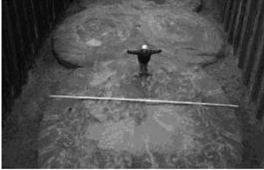
Figure 6.6 Trial SuperJet columns.
