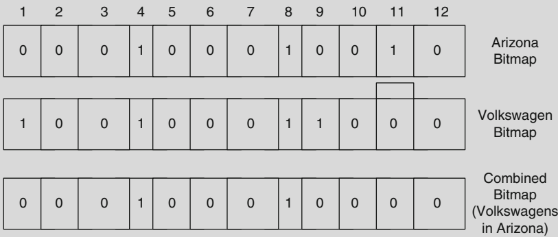
Fig. 4.2 Bitmap Indexes. The top two arrays (bitmaps) record information in a vehicle database for the State of Registration ( Arizona ) and the Manufacturer ( Volkswagen ) respectively. There are as many cells as there are records: a 1 indicates that the value is present, 0 means it is absent. In the first bitmap, the cars in records 4,8 and 11 are registered in Arizona. The third bitmap is computed on the fly if we want to find out all Volkswagens registered in Arizona. The two bitmaps are merged with an AND operation – a given cell takes the value 1 only if both corresponding cells have the value 1: otherwise, it is zero. Here, records 4 and 9 match both characteristics of interest
