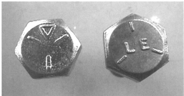
Figure 6-12. Fasteners and forgings are stamped or embossed with identification markings.
