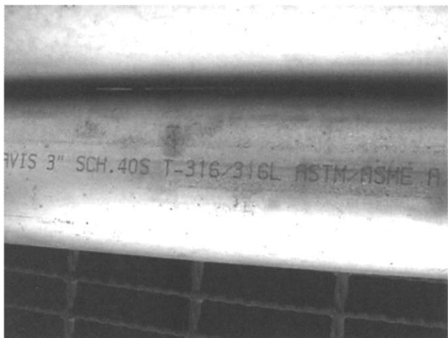
Figure 6-11. Stencil markings are used on wrought products and are usually applied during the manufacturing process.
