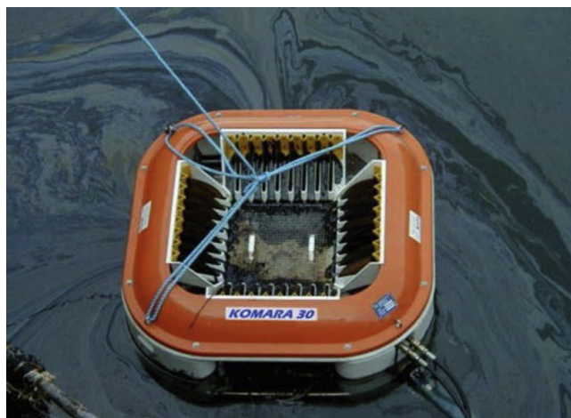
Figure 4.6 Oleophilic disk skimmer (Vikoma International Ltd, 2015).
