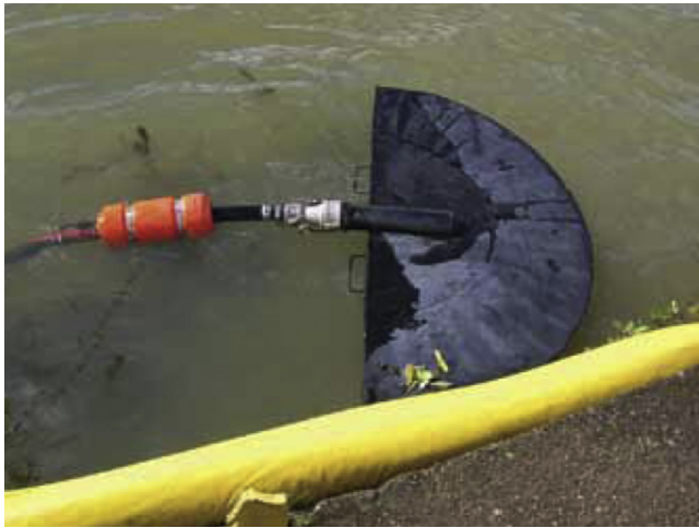
Figure 4.11 Skimmer head of a vacuum/suction skimmer (ITOPF, 2012).
