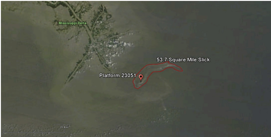
Figure 2.6 A suspected oil slick from site 23,051 in the Gulf of Mexico measuring 18 miles long and covering a surface area of 53.7 square miles. The image was captured on August 11, 2007 by NASA’s Terra spacecraft and is available from the MODIS image library. SkyTruth, 2015a. SkyTruth oil spill reports. Oil Slick Site 23051 2007, 08–11. [Online] Available from: http://oil.skytruth.org/site-23051/site-23051-oil-slick-observations/oil-slick-site-23051-2007-08-11 .
