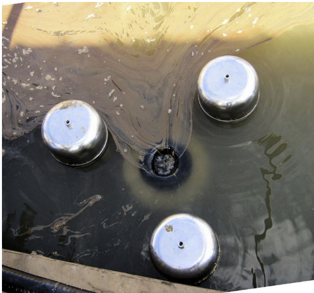
Figure 4.12 Weir skimmer ( https://en.wikipedia.org/wiki/Skimmer_(machine)#/media/File:Self_adjusting_weir_type_oil_skimmer,_Ultraspin.jpg ).
