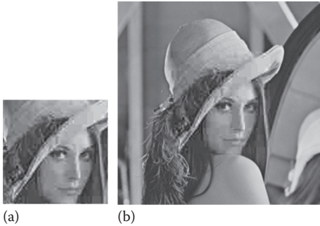
FIGURE 5.11 (a) Clipped version of the JPEG-encoded (10% quality) Lena , (b) the restored version.
