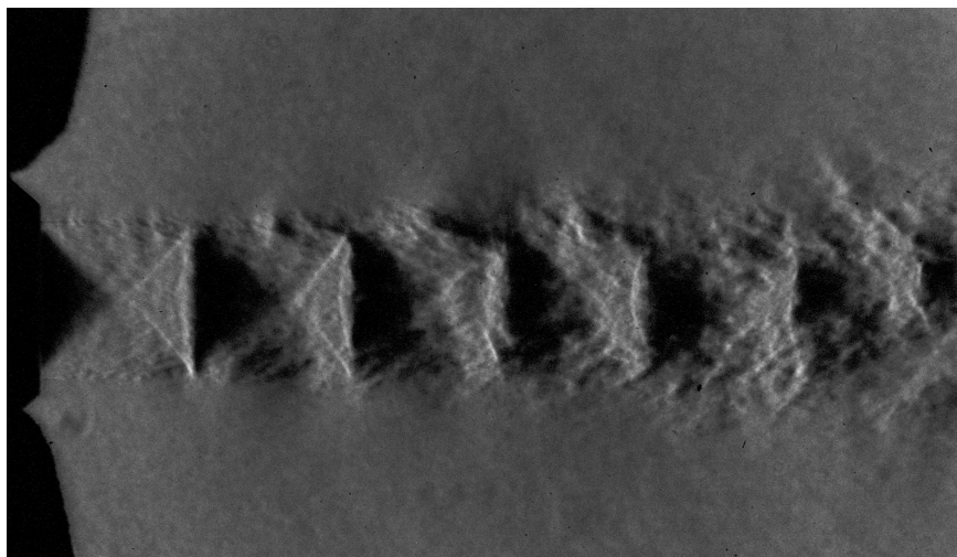
Figure 4.16d: Schlieren picture of Mach 1 jet at NPR 2.5.
