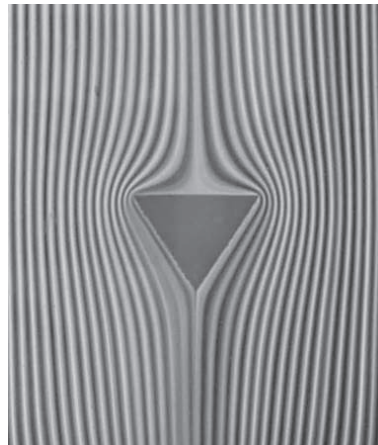
Figure E6.14: Flow past a triangular plate with vertex down
