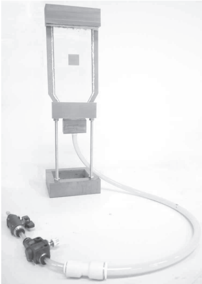
Figure E6.9: A view of complete Hele-Shaw device assembly, with a square plate model in the test-section
