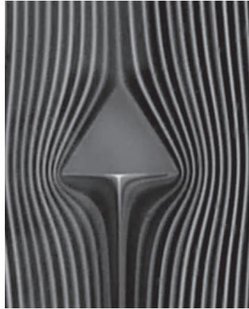
Figure E6.13: Flow past a triangular plate with vertex up
