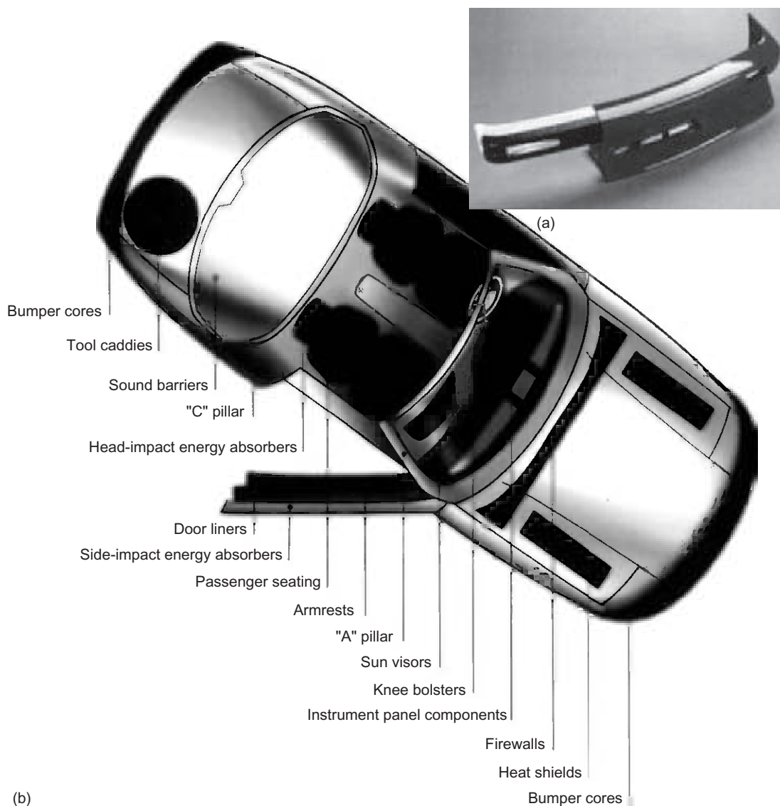
Figure 6.4 Automotive applications for EPP foam (EPP, BASF). (a) A bumper for the Buick Park Avenue and (b) interior and exterior automotive uses of EPP foam ( Neopolen ).
