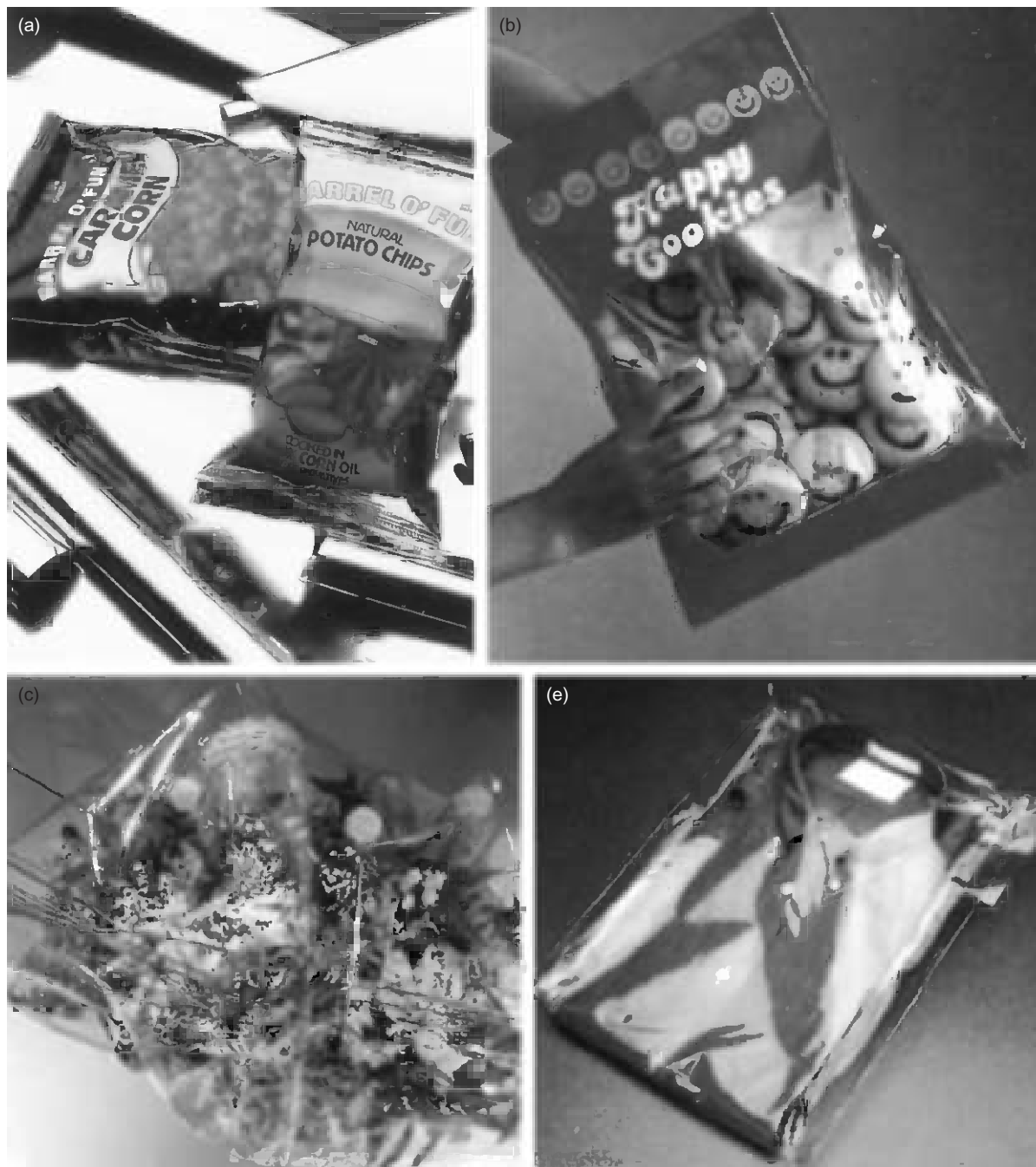
Figure 6.15 Applications of polypropylene films in packaging. (a) Snack food packaging using metallized film (Amoco), (b) snack food packaging using clear film (Amoco), (c) floral packaging (Escorene, Exxon), and (d) apparel packaging (Escorene, Exxon) (Amoco Polypropylene Homopolymers, 1992; Polypropylene, 1993).
