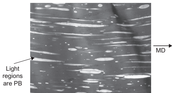
Figure 15.25 Elongated second phase (PB-1 in a polyolefin matrix) found in blown film. Source: Photograph courtesy of DuPont.
