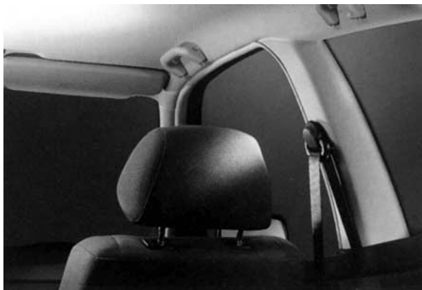
Figure 6.6 Pillar trim of the Volkswagen Polo, made with 20% talc-reinforced polypropylene (Hostacom, Hoechst) (Future—The Hoechst Magazine, 1992).
