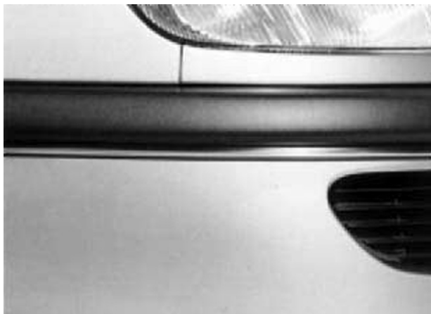
Figure 6.3 A bumper made from talc-reinforced, elastomer-modified polypropylene ( Hostacom, Hoechst ) ( Inform—Hostalen PP, 1996 ).
