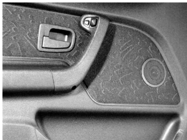
Figure 6.8 Polypropylene door handles on the BMW 3 series (Hostacom, Hoechst) (Inform—Automotive Industry, 1995).
