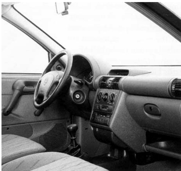
Figure 6.7 Fascia on the Opel Corsa, made from 40% mineral-reinforced polypropylene (Hostacom, Hoechst) (Inform—Automotive Industry, 1995).
