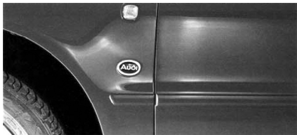
Figure 6.5 The side rubbing or protector strip on the Audi A4, produced from a polypropylene mineral-reinforced thermoplastic elastomer ( Hostacom, Hoechst ). The strip is painted to match the color of the car, and no metal insert is used ( Inform—Automotive Industry, 1995 ).
